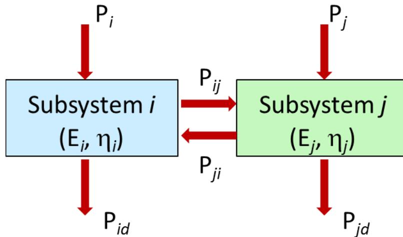
Figure 1. A two subsystems SEA model
