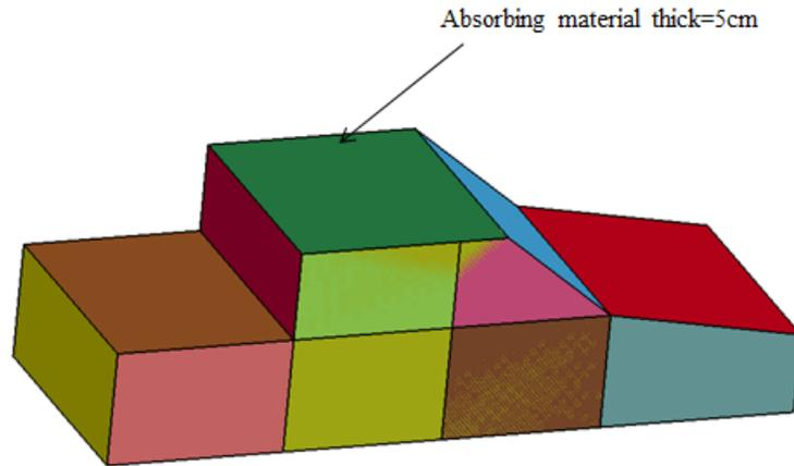
Figure 10. The absorbing material is added to the roof
