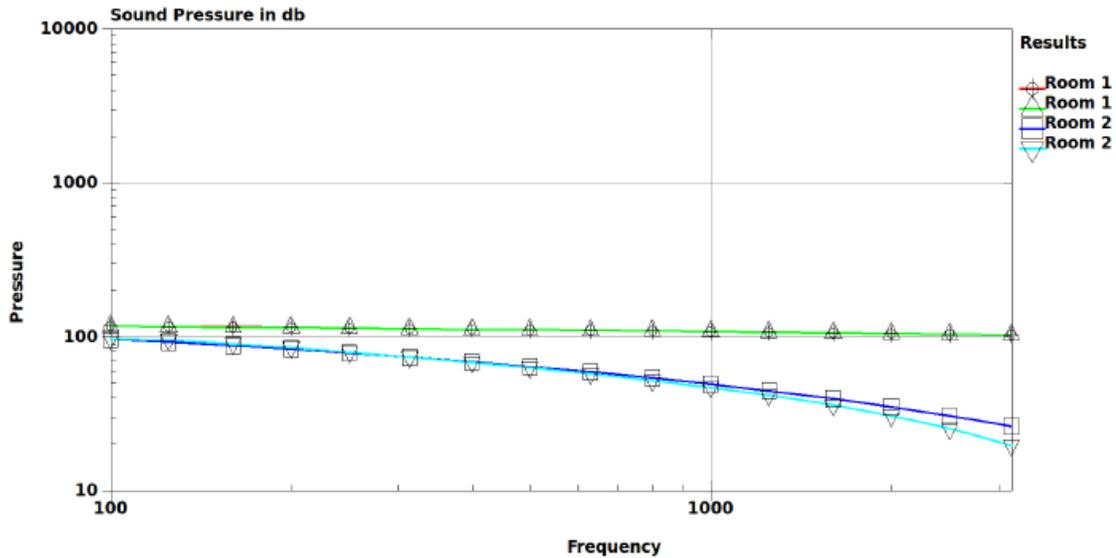
Figure 6. Comparison for acoustic pressure (Log-Log) in room 1 and room 2
