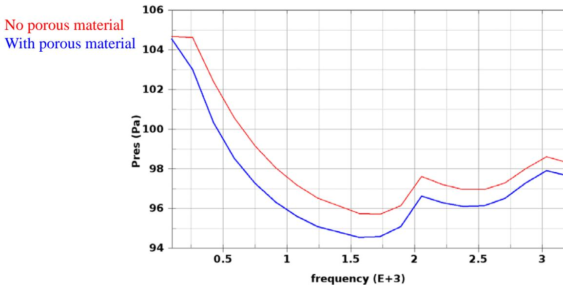
Figure 11. Comparison of acoustic pressure with and without porous material
