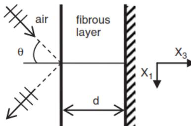
Figure 9. A layer of fibrous material backed by an impervious rigid wall
