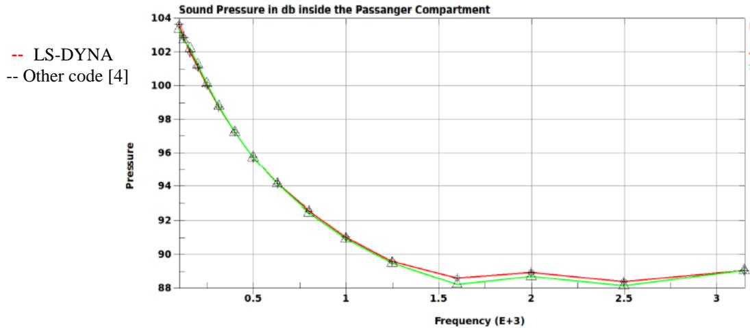
Figure 8. Comparison of acoustic pressure in passenger cavity
