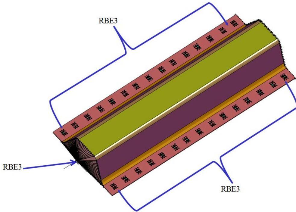
Figure 5. The HAT section model with RBE3 element
