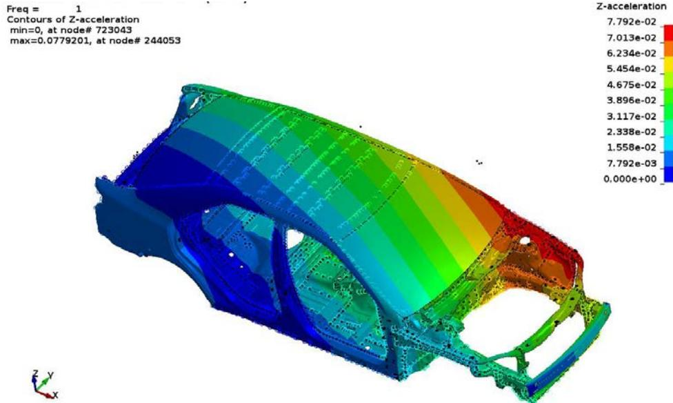
Figure 7. Z acceleration at 1 Hz by MCMS method
