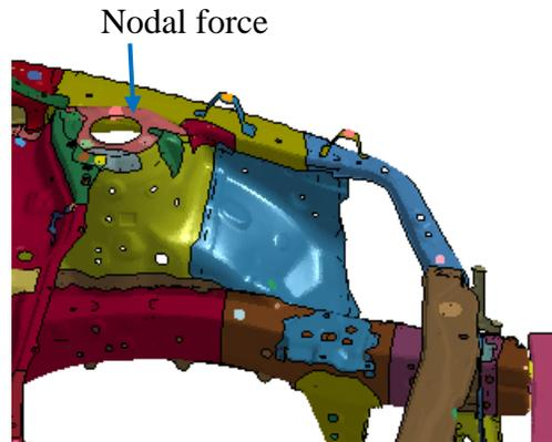
Figure 5. A nodal force applied to the BIW model
