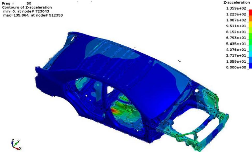
Figure 9. Z acceleration at 50 Hz by MCMS method
