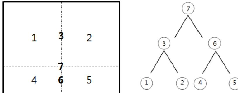
Figure 1. A plate FE model partitioned with two level and the substructure tree topology
