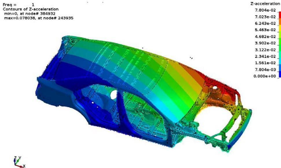
Figure 6. Z acceleration at 1 Hz by Lanczos method
