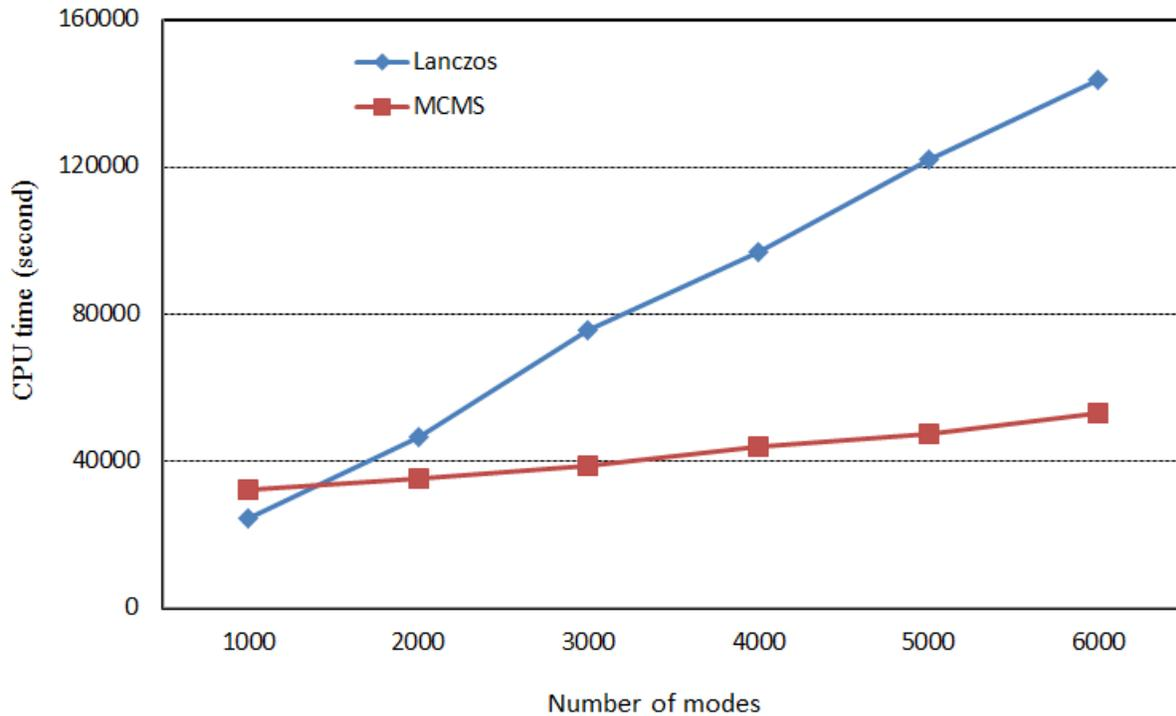
Figure 3. Comparison of CPU time between Lanczos and MCMS
