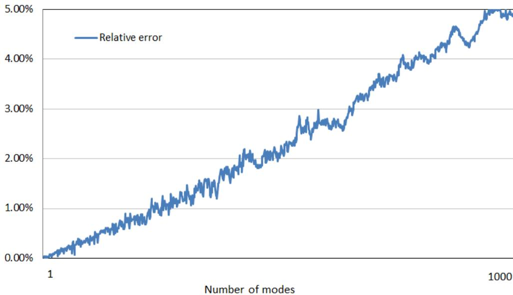
Figure 4. Relative error of eigenvalues computed using MCMS compared to Lanczos
