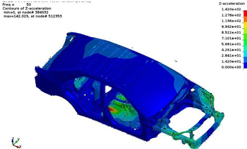
Figure 8. Z acceleration at 50 Hz by Lanczos method
