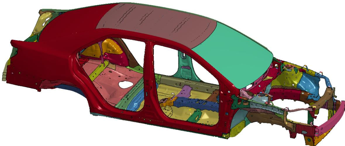
Figure 2. The finite element model of 2012 TOYOTA Camry (NCAC)
