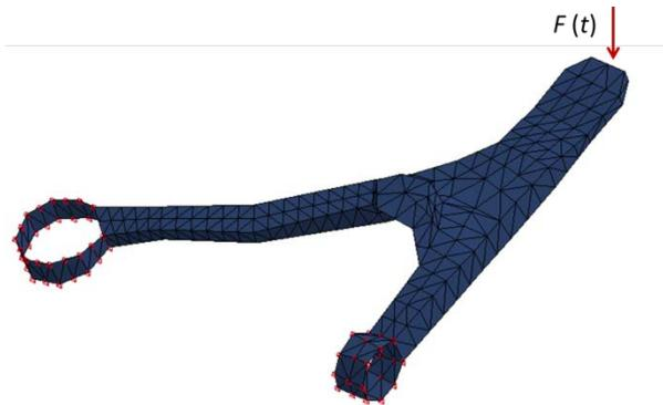
Figure 21. A bracket model with sinusoidal nodal force excitation
