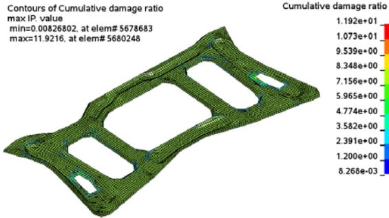
Figure 6. Cumulative damage ratio for x-, y- and z-acceleration loading cases
