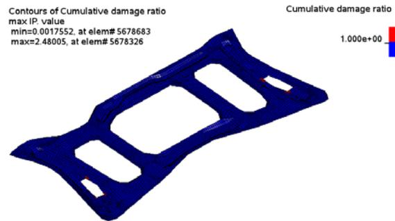
Figure 5. Safe / Failed zone for the case of z-acceleration loading
