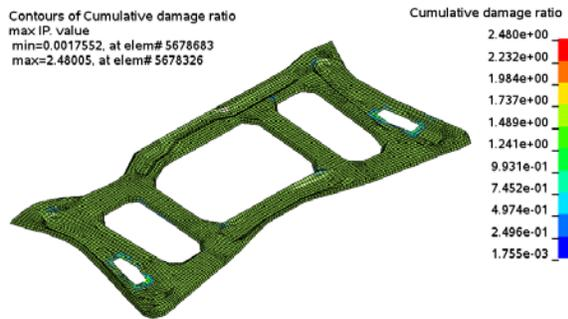
Figure 4. Cumulative damage ratio for the case of z-acceleration loading
