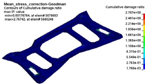
Figure 9. Cumulative damage ratio for z-acceleration PSD loading only (use Goodman’s equation for mean stress correction)
