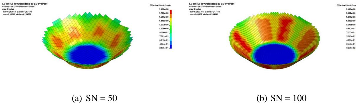
Figure 8. Contours for the effective plastic strain of the blank at the end of the forming processes.
