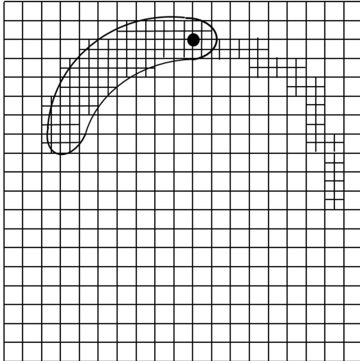
Figure 4: Refined meshes in the tube at the beginning of a subsequent adaptive step. The tube region is formed according to the loading path, adaptive time interval and the user defined radius. Notice that mesh coarsening is carried out outside the tube region, according to curvature of the elements.
