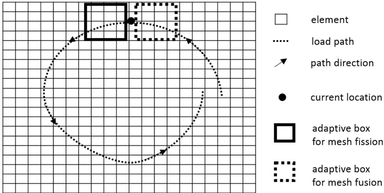
Figure 1: Adaptive boxes on a load path in the current LS-DYNA, mesh is refined in the front and coarsened in the back, which is desirable.
