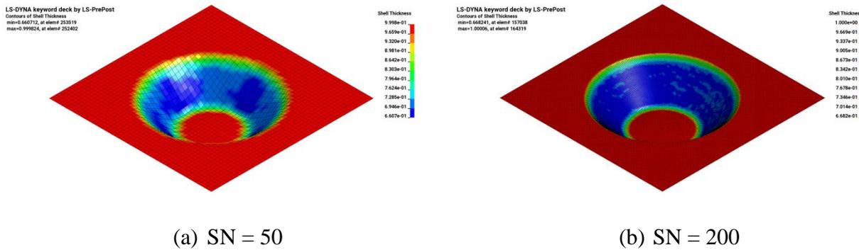
Figure 7. Contours for the shell thickness of the blank at the end of the forming processes.
