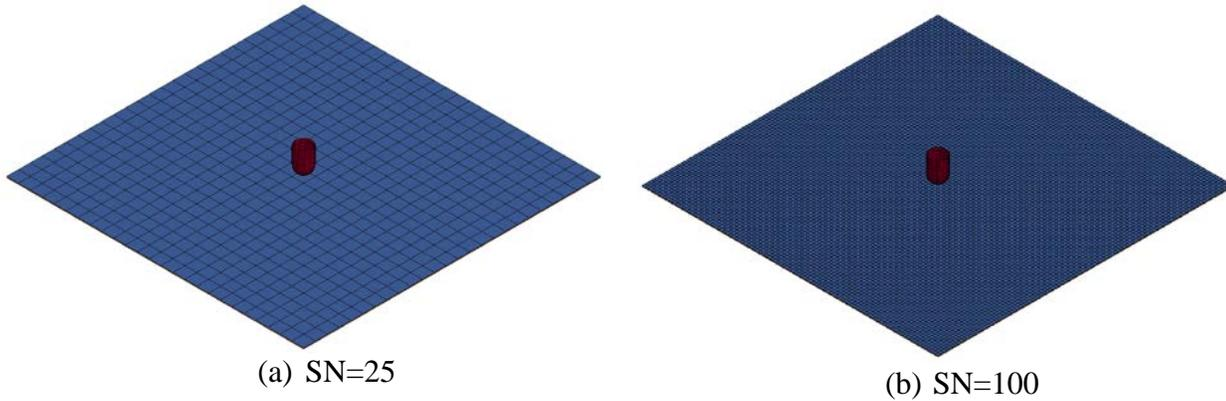
Figure 6. Different meshes of the blank, discretized into quadrilateral elements.
