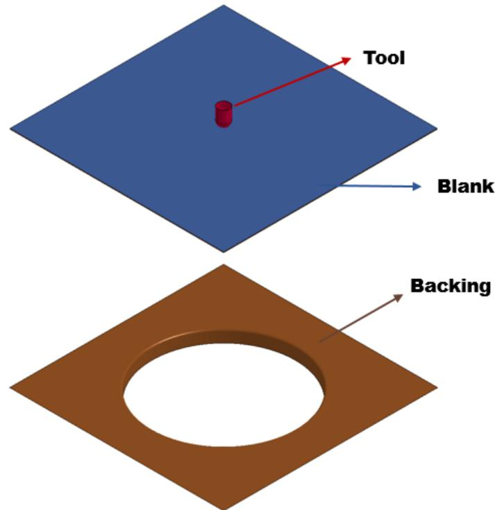
Figure 5. An example of incremental forming: The Tool and Backing are both rigid. Initially, the closest distance between the Blank and Backing is 0.6 mm. A circular loading path is prescribed on the Tool, which will form the Blank into desired shape upon the Backing.
