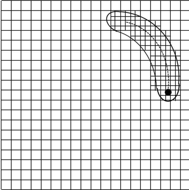
Figure 3. Refined meshes in the tube at the beginning of an adaptive step. The tube region is formed according to the prescribed boundary motion and the user defined radius.
