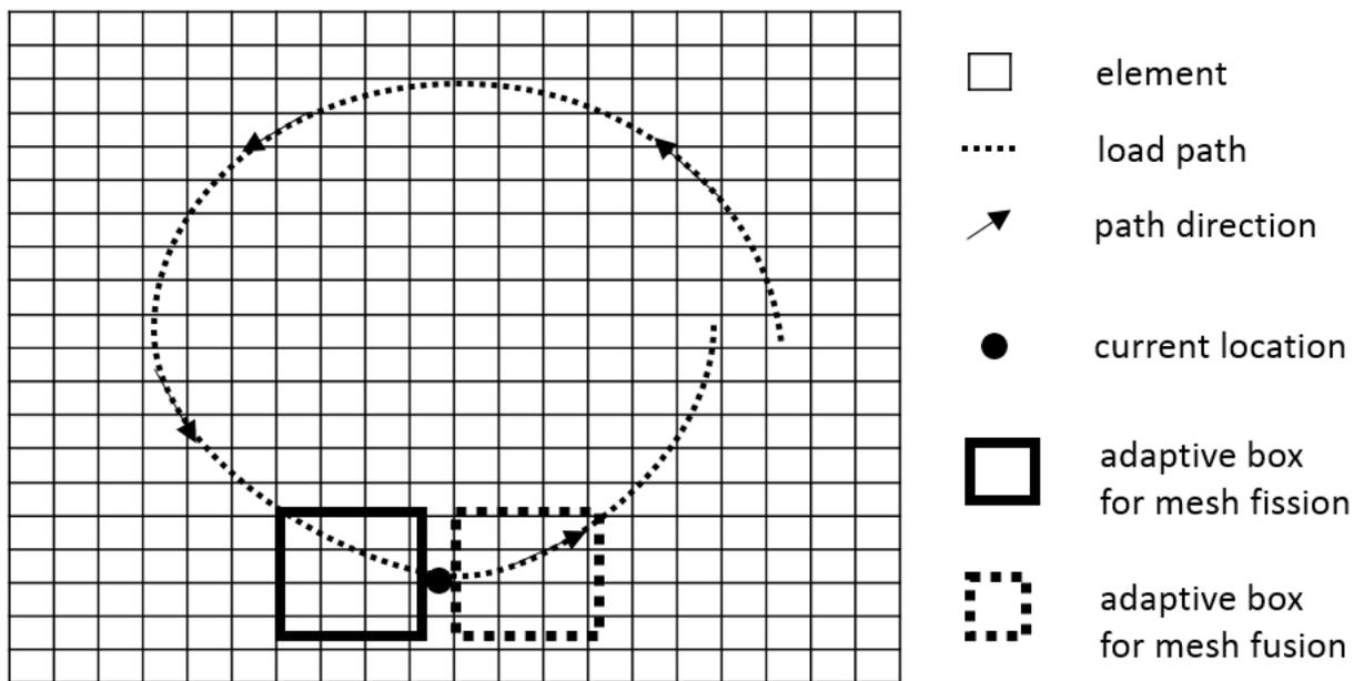
Figure 2: Adaptive boxes on a load path in the current LS-DYNA. Since the path is traced backward, the mesh is coarsened in the front and refined in the back, which is not right.
