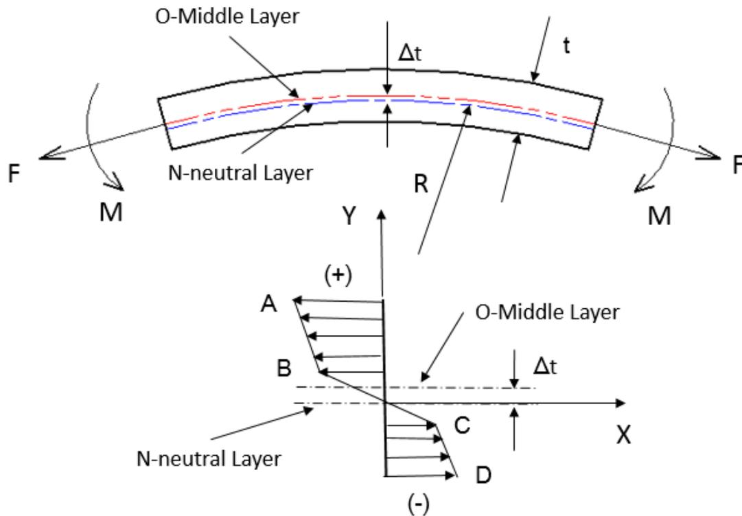
Figure 5. Stretch bending mechanics model
