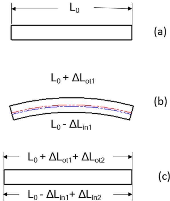
Figure 6. Bending and un-bending. (a) Before bending; (b) After bending; (c) After unbending
