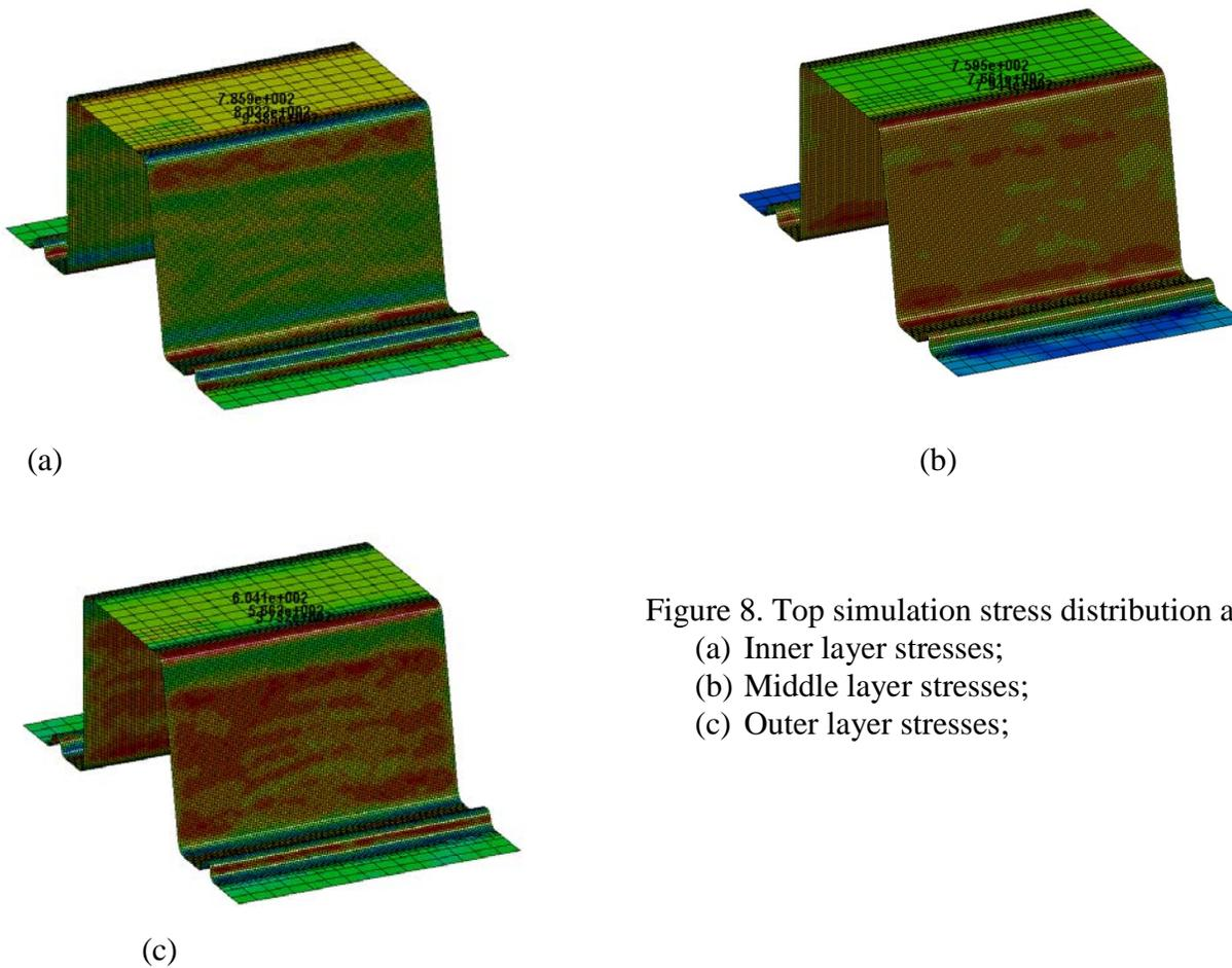
Figure 8. Top simulation stress distribution after unbending
