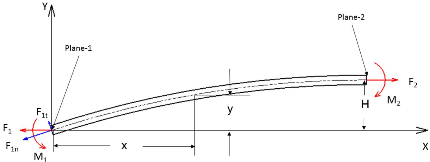
Figure 4. U-Shape part top mechanics model
