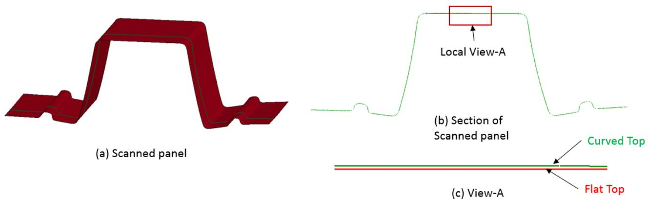
Figure 1. U-Shape part top curvature
