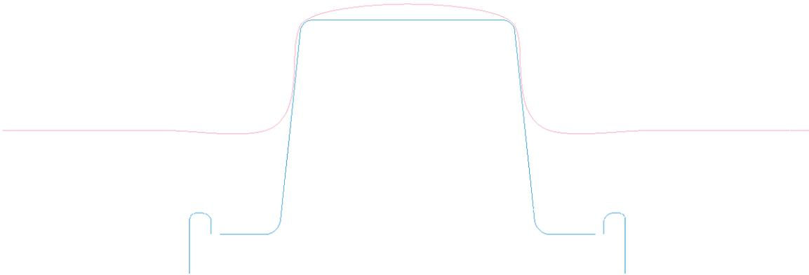
Figure 2. U-Shape part top bending curve
