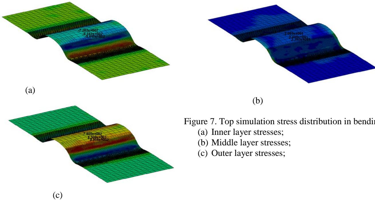
Figure 7. Top simulation stress distribution in bending
