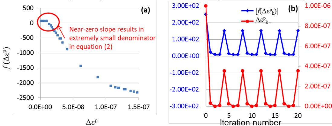
Figure 1 (a)  $f$  as a function of  $\Delta\varepsilon_p$  in the scenario of divergence. (b) The divergence of the return mapping scheme: The red curve shows each iterate and the blue shows the corresponding  $f$  evaluations. The secant procedure would direct the solution away from the true root whenever the iterate gets into the flat part of the curve indicated in (a). Therefore the iterate keeps bouncing without a sign of convergence.
