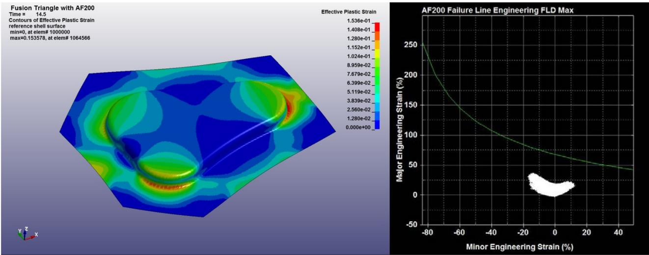
Figure 5b: partially formed blank shown alongside limit strain diagram for fracture.
