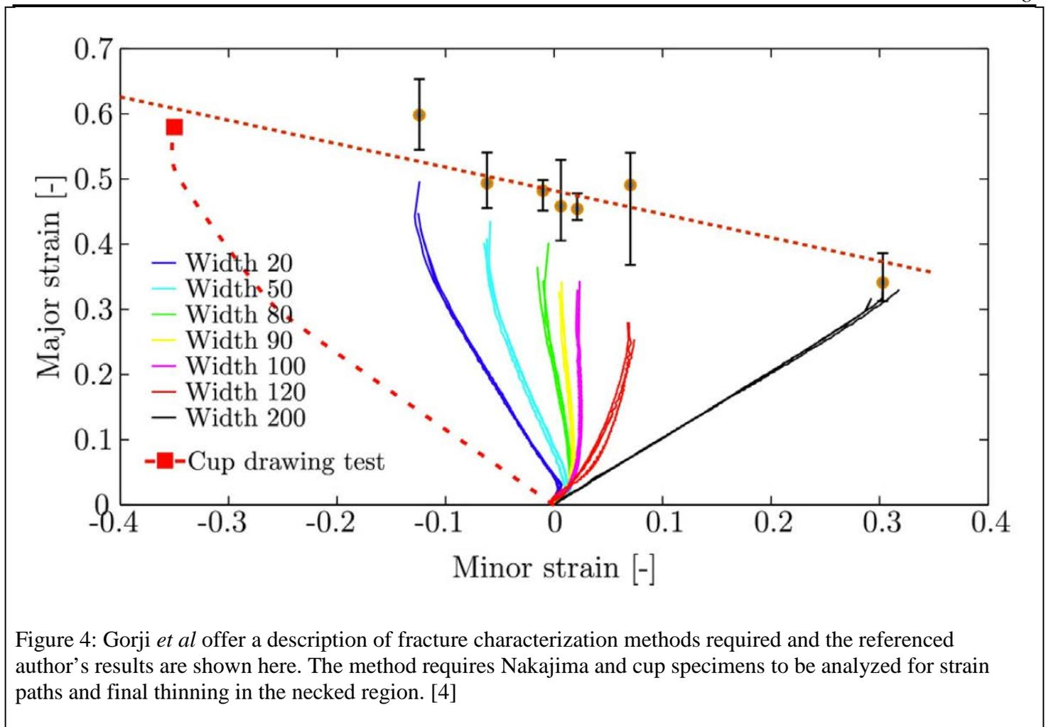
Figure 4: Gorji *et al* offer a description of fracture characterization methods required and the referenced author's results are shown here. The method requires Nakajima and cup specimens to be analyzed for strain paths and final thinning in the necked region. [4]
