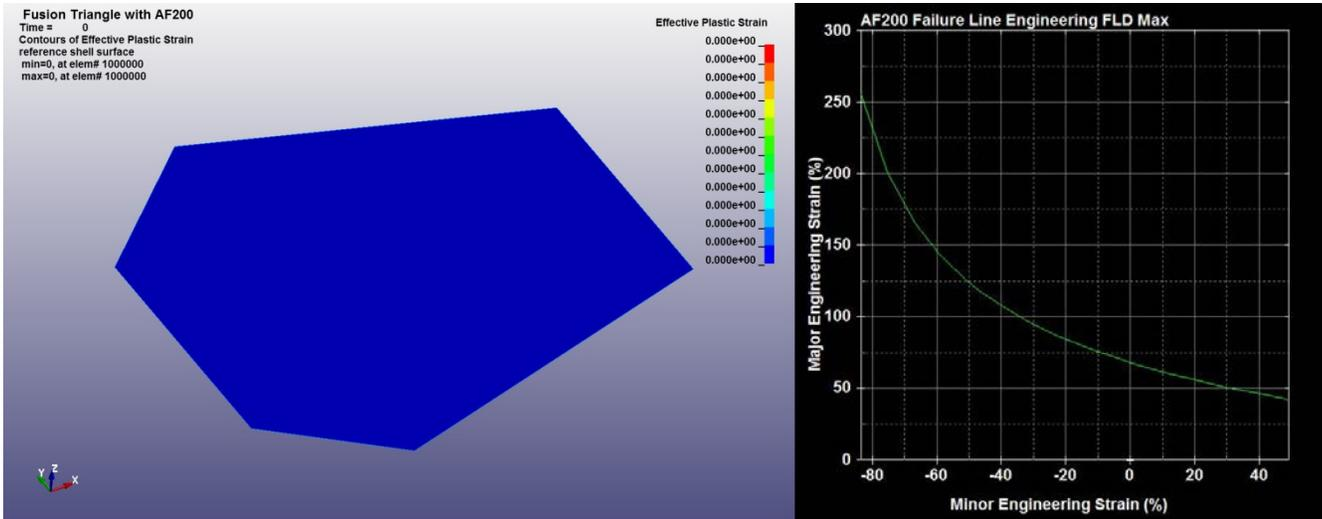
Figure 5a: initial blank shown alongside limit strain diagram for fracture. Strain is engineering and plotting is described below.
