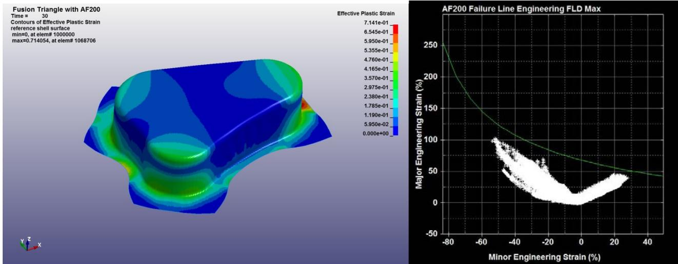
Figure 5c: part at depth of 55mm shown alongside limit strain diagram for fracture.
