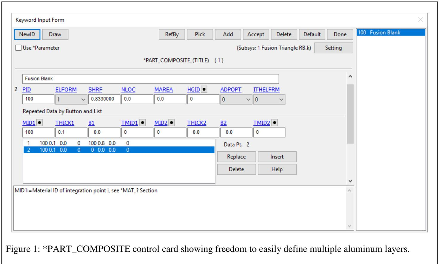
Figure 1: \*PART\_COMPOSITE control card showing freedom to easily define multiple aluminum layers.
