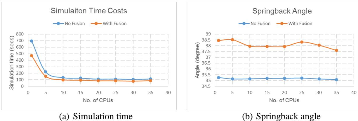
Fig. 5. Comparisons of the simulation CPU time and springback angles in MPP with different number of CPUs, with and without mesh fusion.
