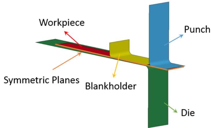
Fig. 1. NUMISHEET'93 Benchmark: The punch, die and blankholder are rigid; the workpiece is discretized into shell elements. A forming process is conducted, followed by a springback analysis.
