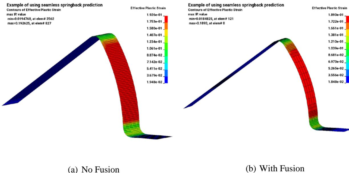
Fig. 3. The final effective plastic strain contours of the workpiece running with 10 CPUs in MPP.
