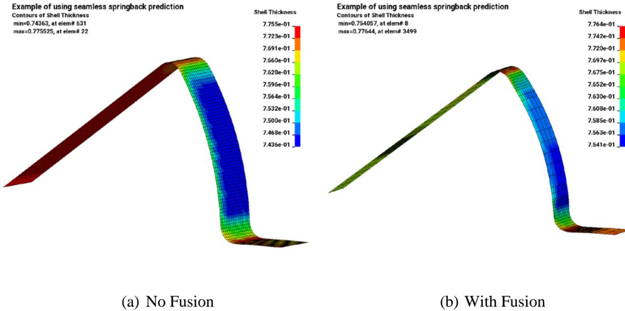
Fig. 4. The final shell thickness contours of the workpiece running with 10 CPUs in MPP.
