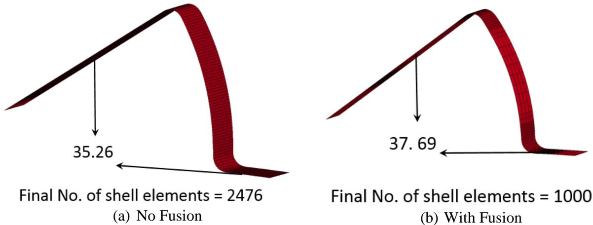
Fig. 2. The final number of elements and springback angles of the workpiece running with 10 CPUs in MPP.
