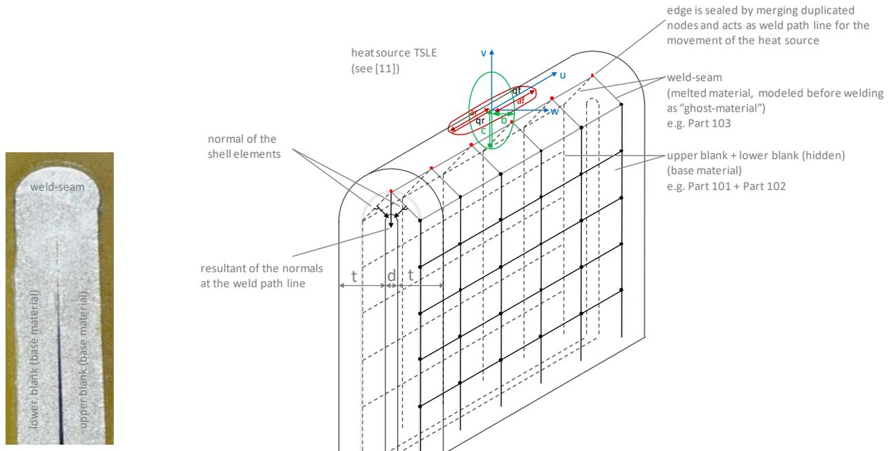
**Fig. 3:** Modeling scheme of a double-layered “Die-Less-Hydroforming” blank ([2], originally from [8], edited) including heat source for welding & corresponding exemplified macro-section of the edge weld, additional fixation equipment is not illustrated
