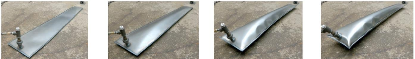
(a) initial state with a smooth buckling pattern due to welding
