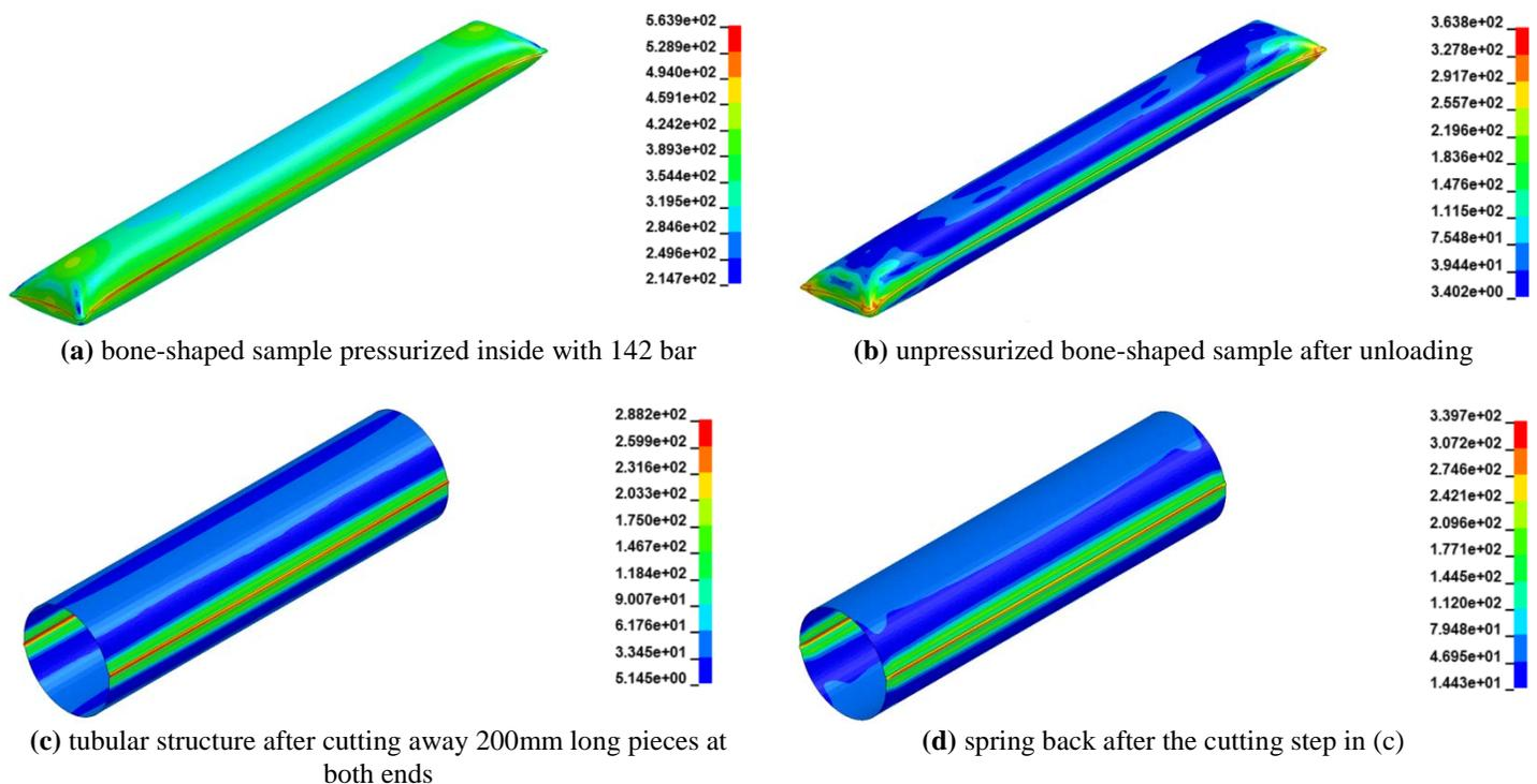
**Fig. 9:** Preparation steps for a load-Capacity simulation showing v. Mises Stress [MPa] at middle integration point for the different states of preparation and the resulting tubular structure (d)
