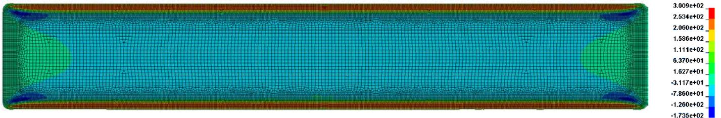
(a) Residual stress state after welding and cooling down in terms of global stress in longitudinal direction [MPa] for a sample with sheet thicknesses of 2mm with well suited regular welding
