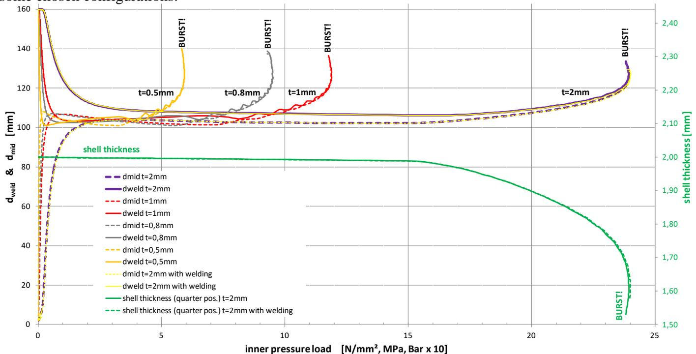
**Fig. 6:** Development of  $d_{mid}$ ,  $d_{weld}$  and sheet thickness vs. inner forming pressure load for some configurations with or without prior welding simulation
