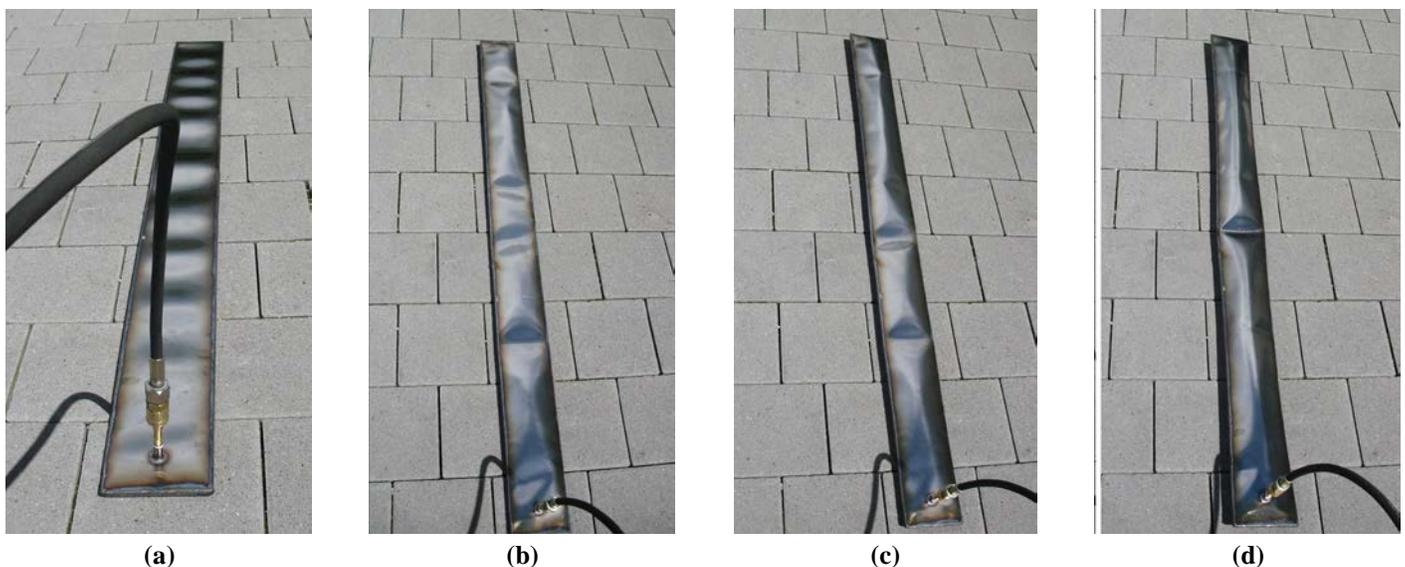
**Fig. 1:** Strip-shaped Die-Less-Hydroforming sample with welding distortions in terms of a buckle pattern after welding at initial state (a) and here from the development of some wrinkles during the subsequent inflation process (b), (c) & (d) (Image source: Bachelor thesis at Karlsruhe Institute of Technology, KIT Steel & Lightweight Structures, Research Center for Steel, Timber & Masonry)
