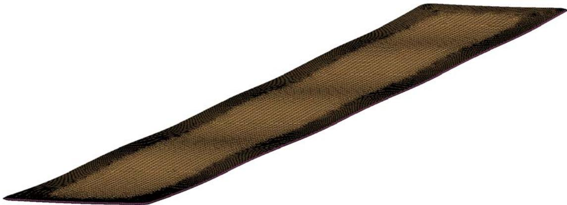
(d) 3D- view of the sample with sheet thicknesses of 1mm showing a characteristically buckling pattern
