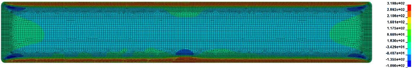
(b) Residual stress state after welding and cooling down in terms of global stress in longitudinal direction [MPa] for a sample with sheet thicknesses of 2mm with a “unmeant” heat hotspot during welding at the middle of the lower seal-weld
