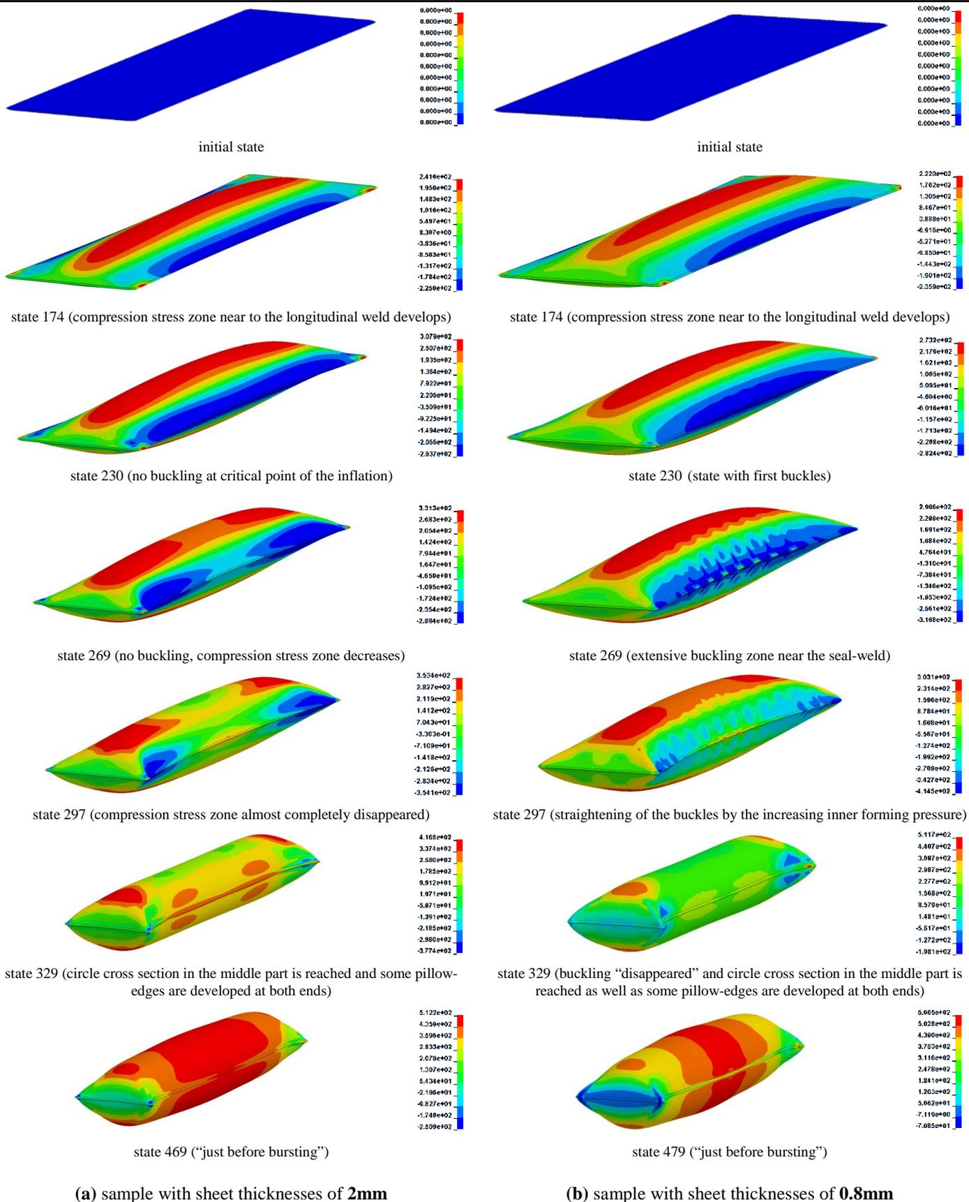
**Fig. 8:** Element true stresses [MPa] in global longitudinal direction of the strip-shaped sample (midplane integration point) for different states during the inflation (with identical mass vs. time input rate)
