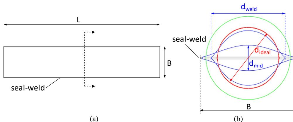
**Fig. 5:** Top view of the double-layered strip-shaped Die-Less-Hydroforming blank with dimensions (a) and cross section view (b) at different states of inflation as well as definition of some parameters [5]
