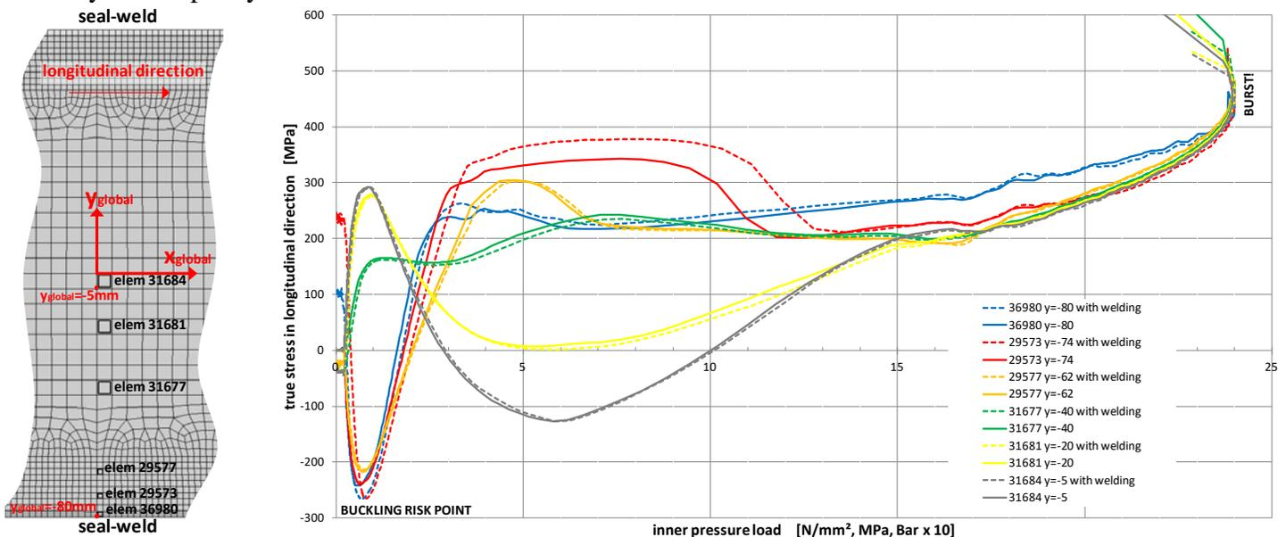
**Fig. 7:** Development of true stress in longitudinal sample direction vs. inner forming pressure load for configuration with or without prior welding simulation for some elements from weld seam (pos. -80) to the middle of the blank width (pos.-5) including illustration of the size-graded mesh
