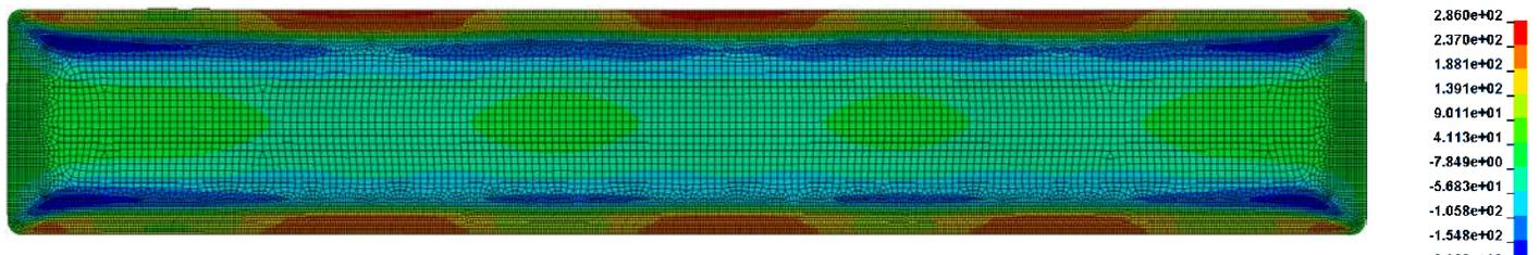
(c) Residual stress state after welding and cooling down in terms of global stress in longitudinal direction [MPa] for a sample with sheet thicknesses of 1mm showing a characteristically buckling pattern
