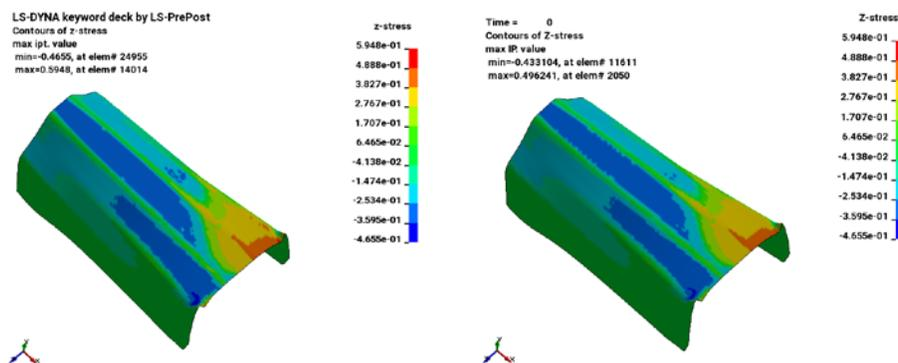
Figure 2: The one-step solutions using finite elements (left) and trimmed NURBS (right).
