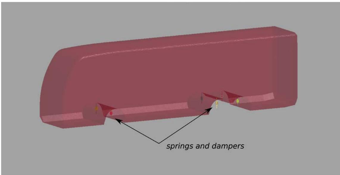
Figure 2: Mechanical model in LS-DYNA.
