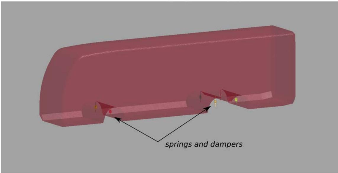
Figure 2: Mechanical model in LS-DYNA.
