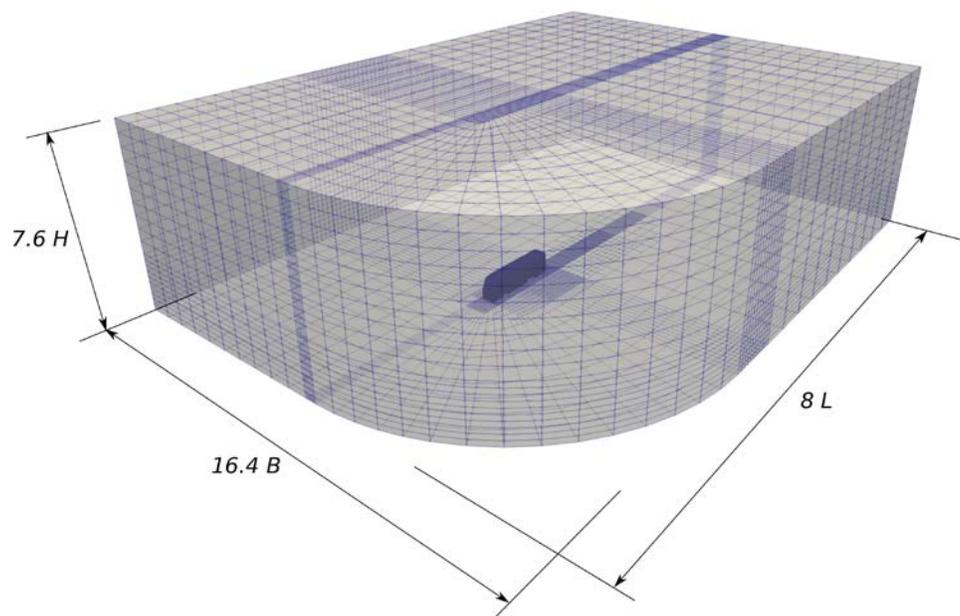
Figure 3: Configuration of the computational domain mesh (OpenFOAM).
