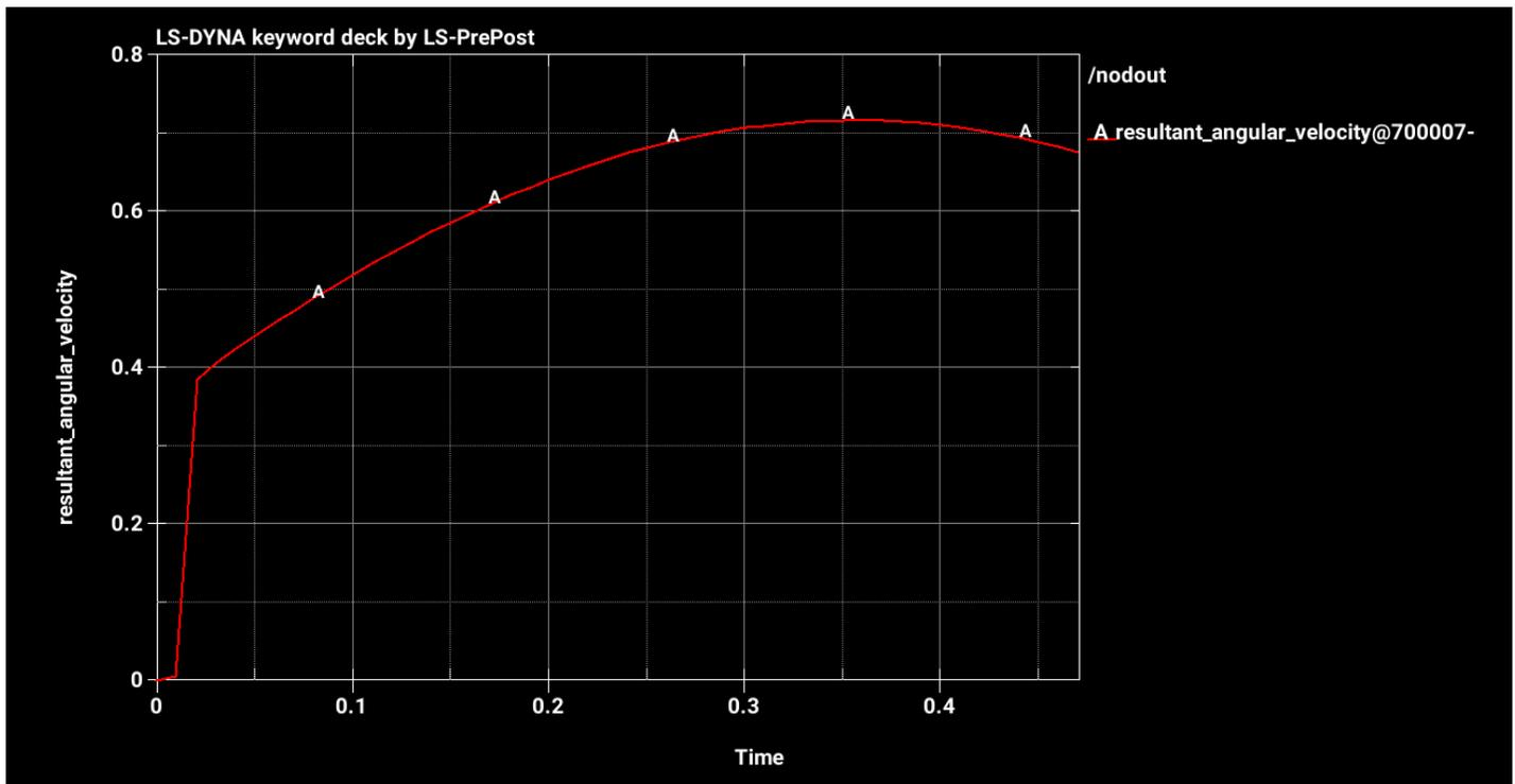
Figure 5: Velocity of the bus center of mass during rollover.
