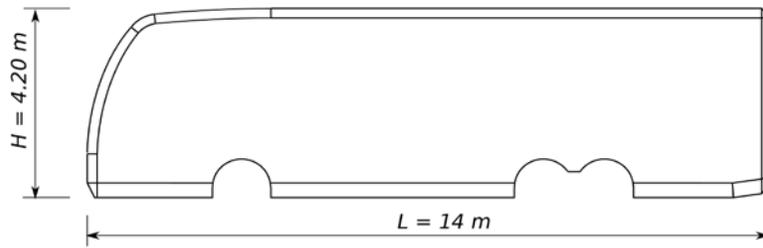
Figure 1: Main dimensions of the simplified double-deck bus model.
