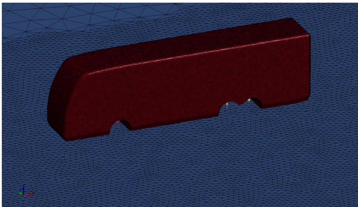
Figure 4: CFD surface mesh (LS-DYNA).
