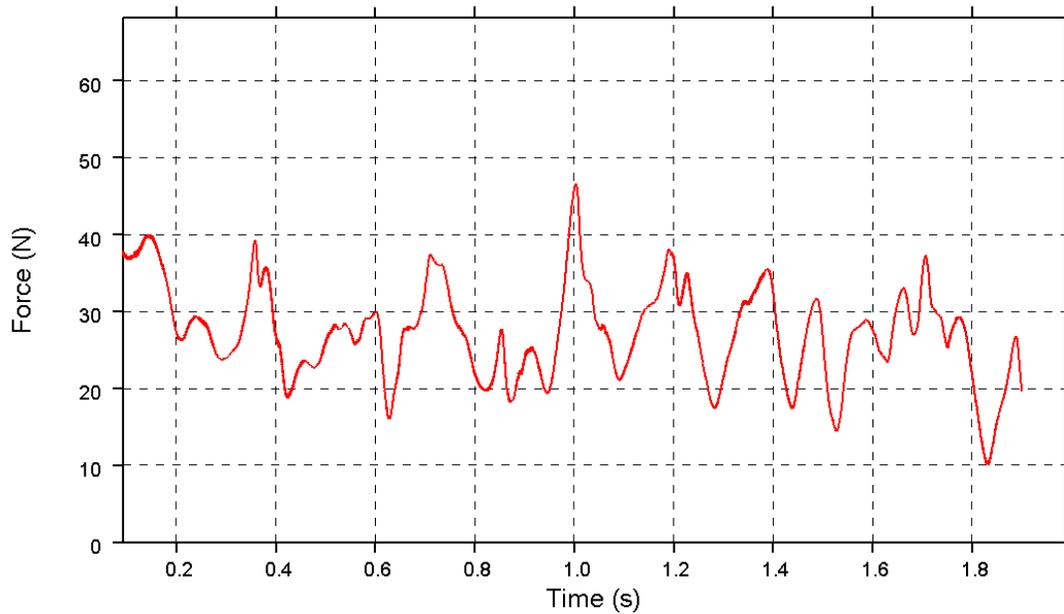
Figure 9 Time history of the vertical load on the hood of the following car
