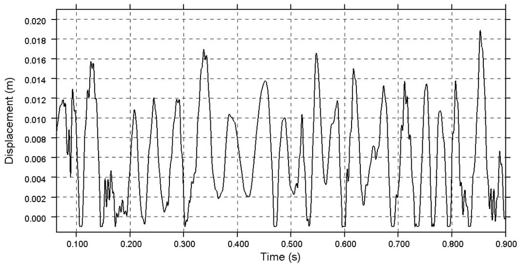
Figure 18 Time series of the deflection of the edge of the hood. Extracted from the simulation with a free stream velocity of 15m/s
