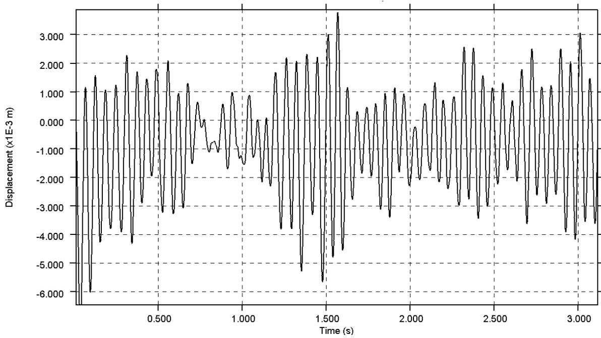
Figure 11 Time history of the vertical displacement of the end plate
