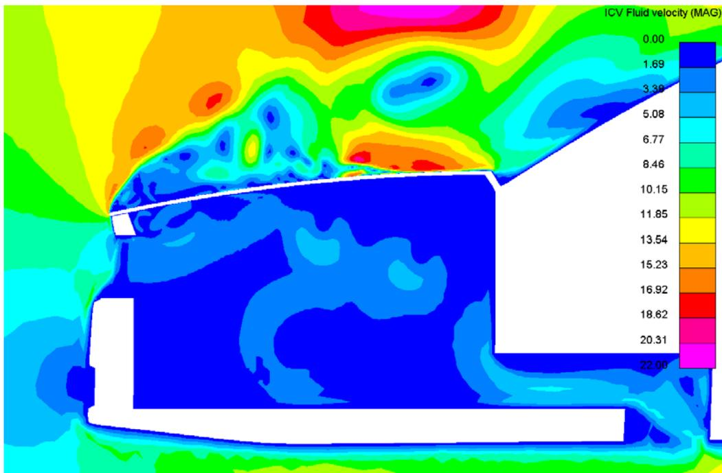
Figure 16 Velocity Contours from CFD simulation of sharpened hood profile
