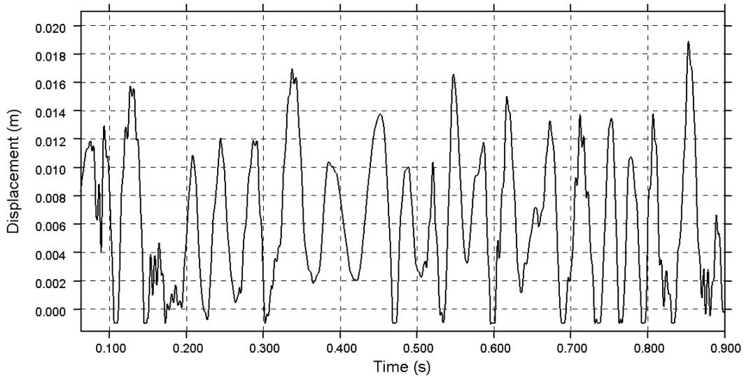
Figure 18 Time series of the deflection of the edge of the hood. Extracted from the simulation with a free stream velocity of 15m/s
