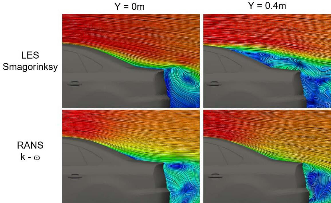
Figure 6 Velocity profiles around the rear window from the RANS and LES simulations
