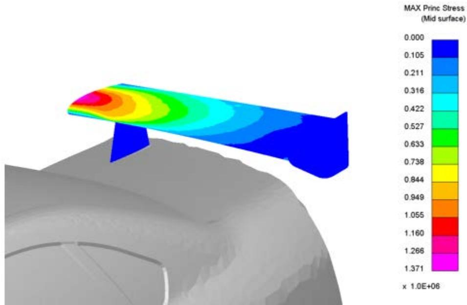
Figure 13 Maximum principal stress on spoiler during FSI simulation
