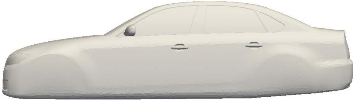
Figure 3 DrivAer geometry used for validation study
