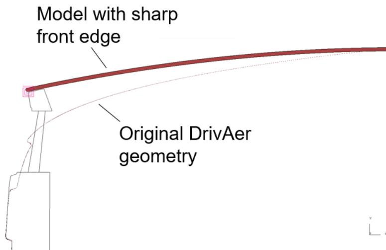
Figure 14 2D model of modified DrivAer car with a flexible hood
