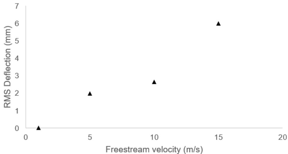
Figure 19 RMS deflection of the edge of the hood at a range of freestream velocity conditions
