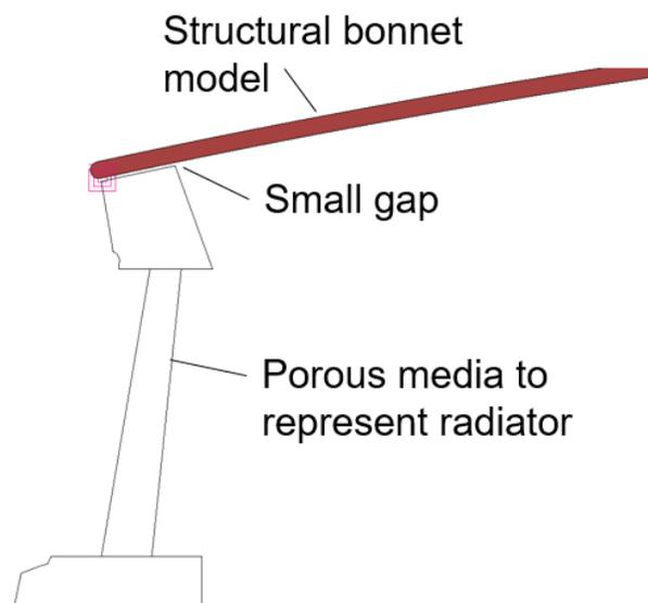
Figure 15 Close up of detail around the front of the 2D car model
