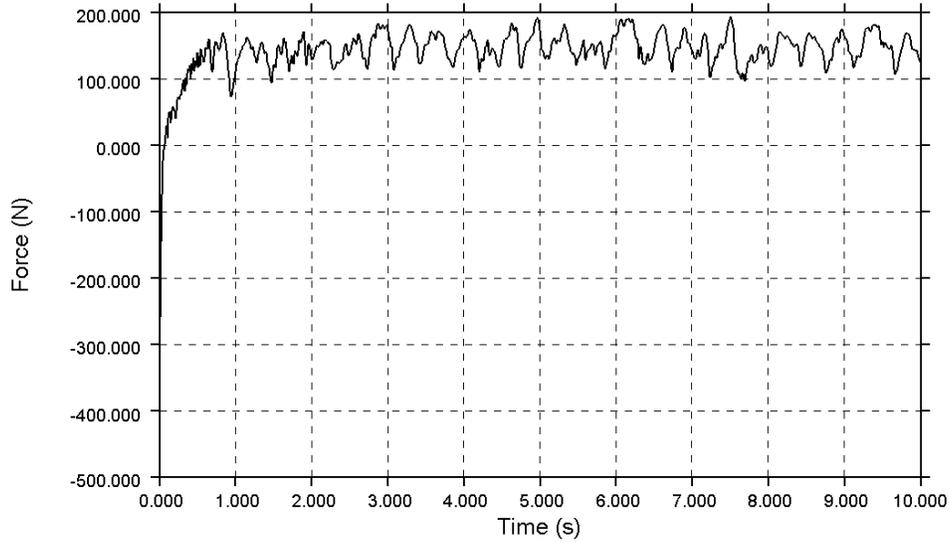
Figure 17 Time series of vertical load on the spoiler.
