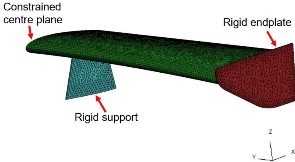
Figure 10 Structural model used in FSI simulation
