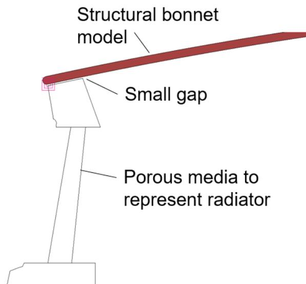
Figure 15 Close up of detail around the front of the 2D car model
