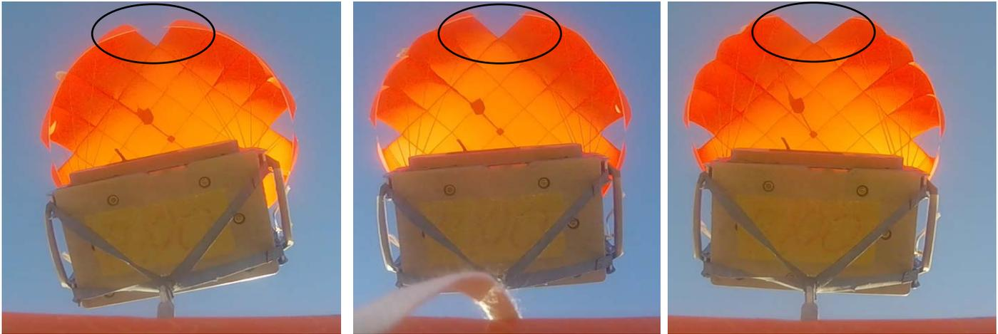
Figure 4: View from payload past AGU to canopy **Left**, deployment configuration with 0% stroke extended and the actuated corners tied together; **Center**, approximately 50% of total stroke deployed; **Right**, 100% of stroke extended to produce the fully deployed configuration. In all images, the actuated corners are at the top of the figure.
