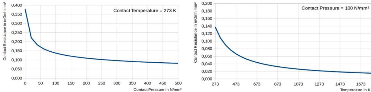
Figure 8 Example electrical contact resistance according Jonny-Kaars-Model
