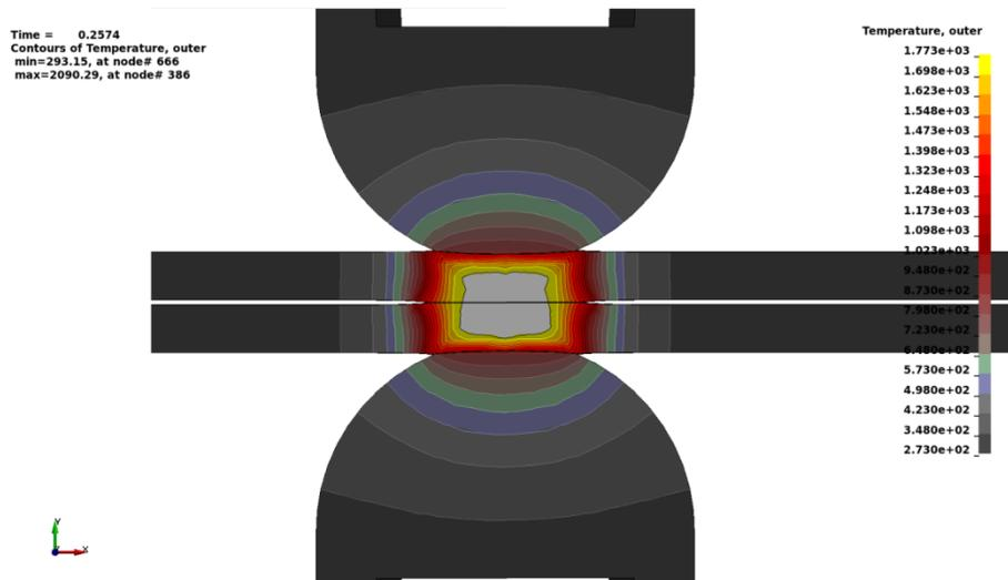
Figure 12 Weld Nugget at dynamic test
