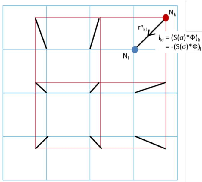
Figure 5 Illustration of the local node to node resistances used to connect the 2 parts using the contact resistances locally defined by the \*DEFINED\_FUNCTION
