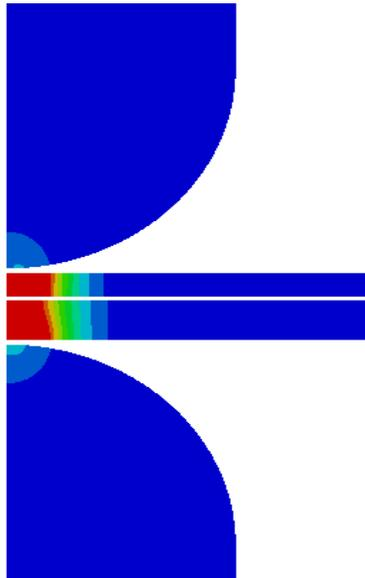
Figure 7 2D RSW model (Note: the Y axis is the symmetry axis)
