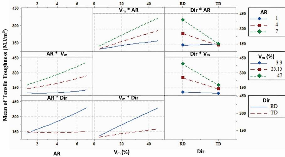
Fig. 5: Interaction Plots for tensile toughness (fitted means)
