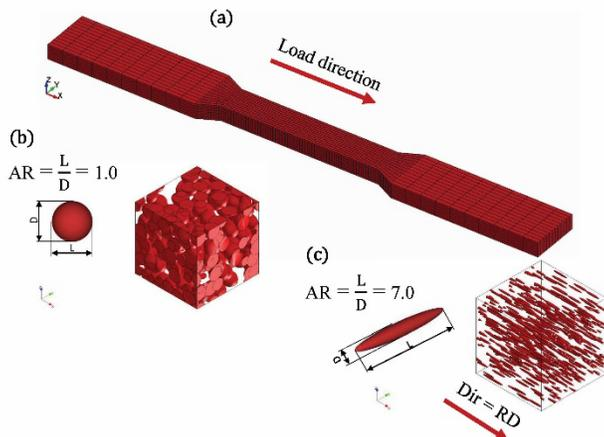
Fig. 2: (a) A standard ASTM E8 specimen geometry with load direction (b) RVE with  $AR=1$ ,  $Dir=RD$ , and  $V_m=47\%$  (DP#20), and (c) RVE with  $AR=7$ ,  $Dir=RD$ , and  $V_m=3.3\%$  (DP#4)
