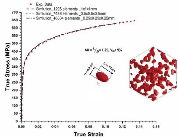
Fig. 3: Comparison between the experimental and numerical results at specific microstructure parameters ( $AR=1.85$ ,  $Dir=$  random 3D, and  $V_m=9\%$ ) [14] and different mesh size
