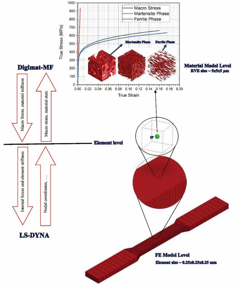
Fig. 1: Multiscale material modeling using Digimat as the material modeler and LS-DYNA as structural FEA software
