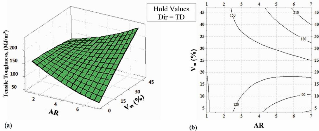
Fig. 6: (a) 3D surface plot of response surface showing the effect of aspect ratio (AR), martensite volume fraction ( $V_m$ ), and their mutual effect on toughness at  $Dir = TD$ ; (b) corresponding 2D contour plot.
