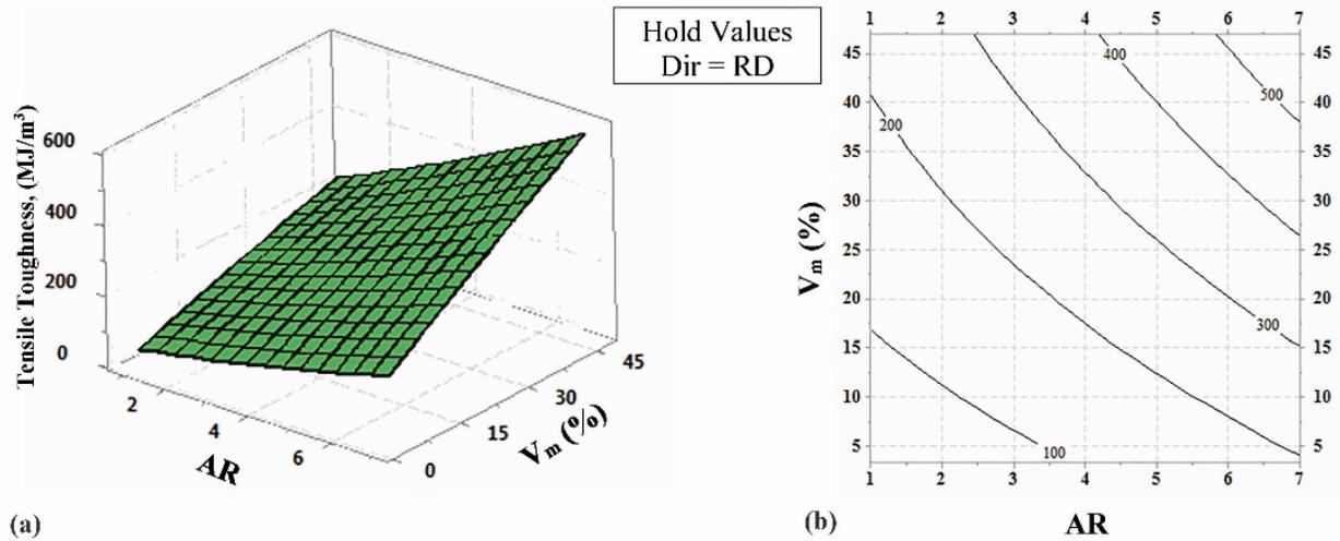
Fig. 7: (a) 3D surface plot of response surface showing the effect of aspect ratio (AR), martensite volume fraction ( $V_m$ ), and their mutual effect on toughness at Dir = RD; (b) corresponding 2D contour plot.
