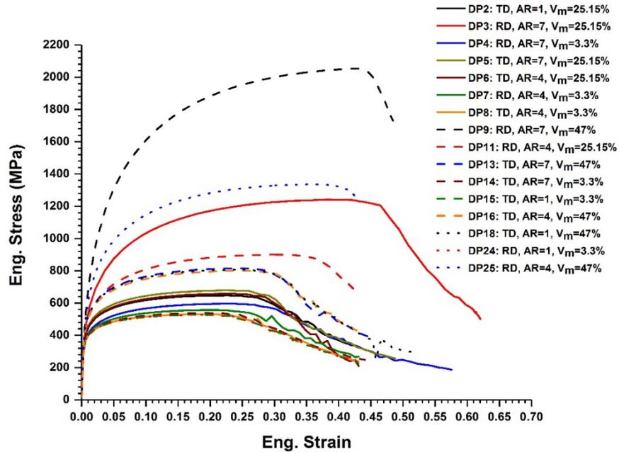
Fig. 4: Numerical stress–strain curves for all design points in the analysis
