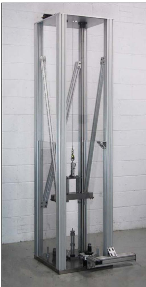
Figure 2: Veryst Engineering's custom-built drop tower.
