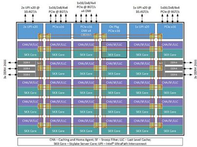
Figure 1. Intel Xeon Skylake-SP mesh-based microarchitecture
