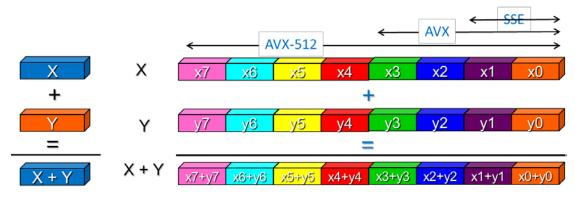
Figure 3. Intel Advanced Vector Extensions technology
