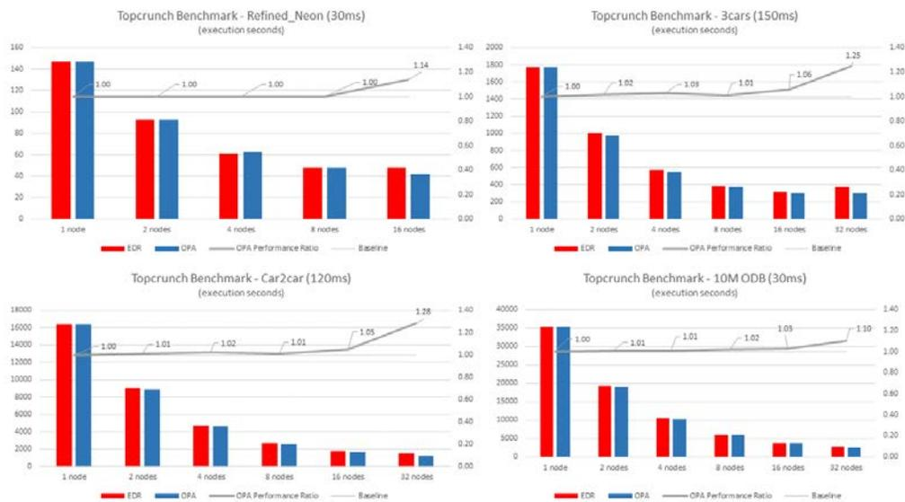
Figure 7. LS-DYNA scaling on OPA versus InfiniBand EDR
