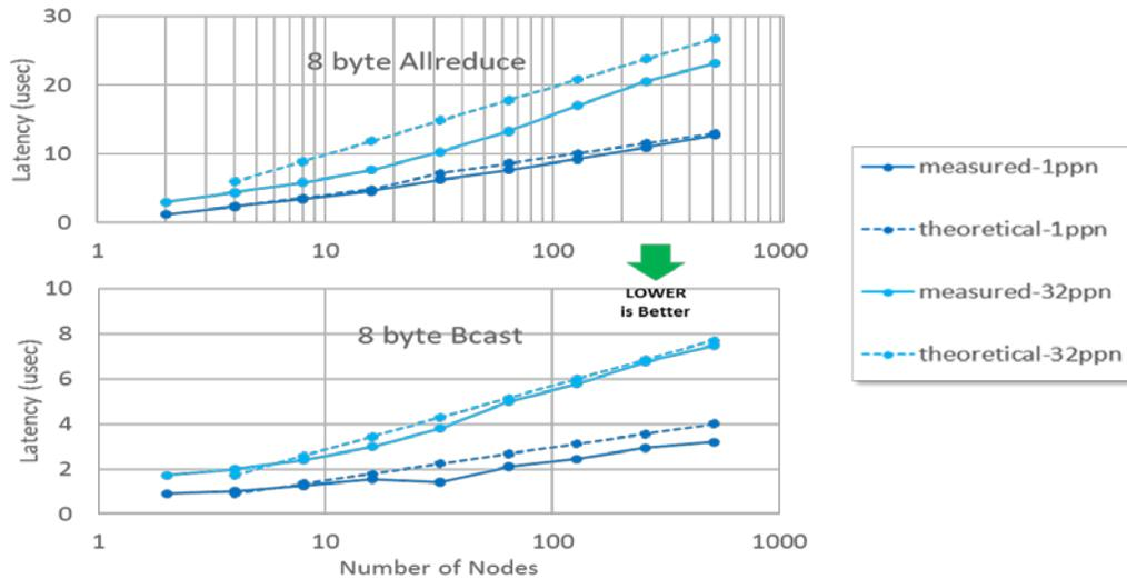
**Figure 8.** Scaling collectives up to 512 Intel<sup>®</sup> Xeon<sup>®</sup> Gold 6142 processor nodes (ppn is number of MPI ranks per node)
