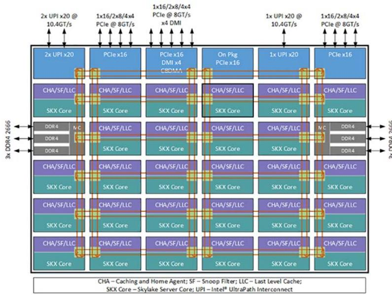
Figure 1. Intel Xeon Skylake-SP mesh-based microarchitecture
