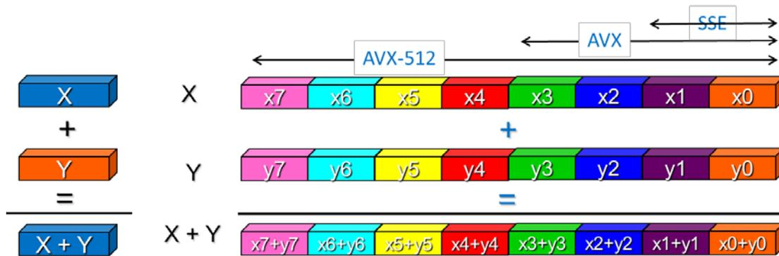
*Figure 3. Intel Advanced Vector Extensions technology*
