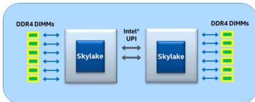
Figure 2. Two socket configuration with Intel UPI
