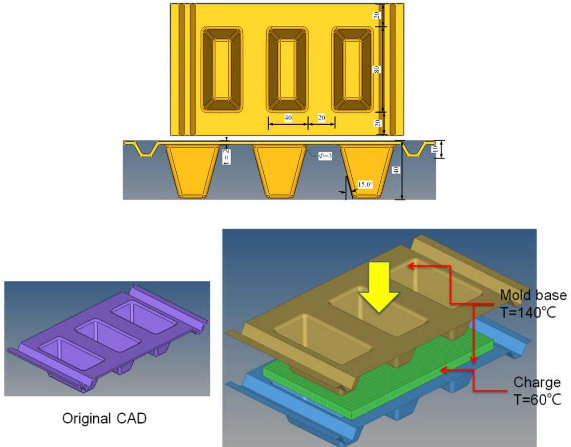
Figure 3. Compression molding model
