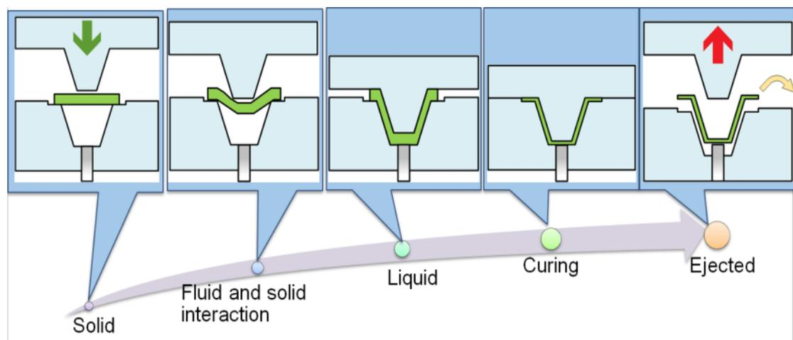
Figure 1: The compression molding process
