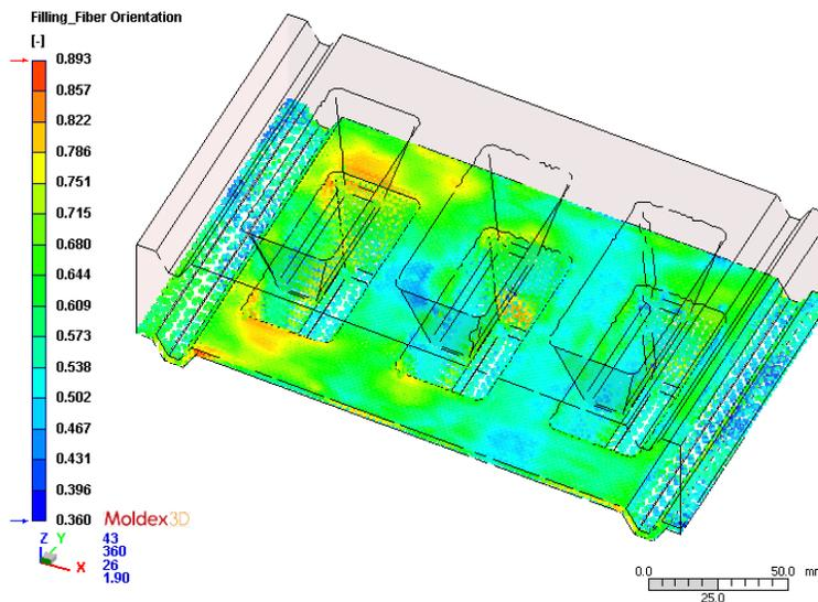
Figure 9. Fiber orientation at EOF
