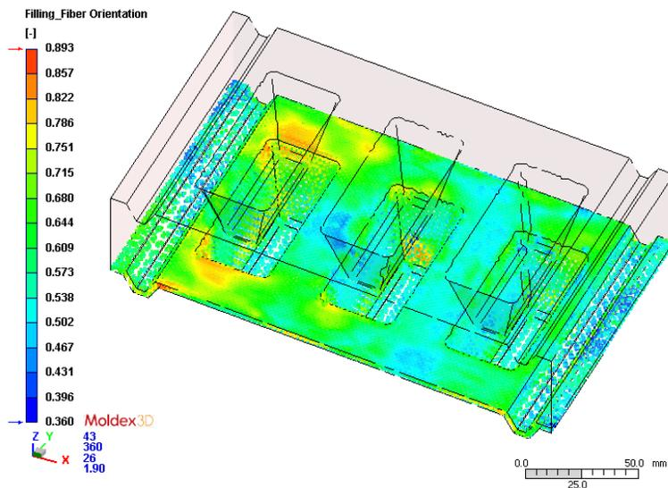
Figure 9. Fiber orientation at EOF
