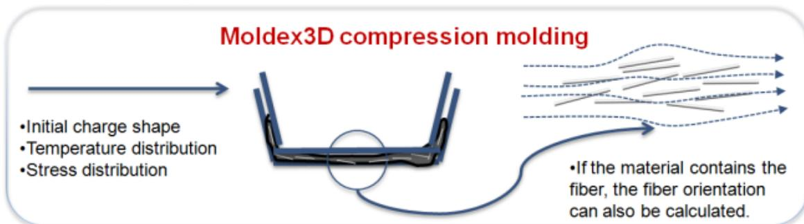
Figure 2. Integration analysis between Moldex3D and LS-DYNA
