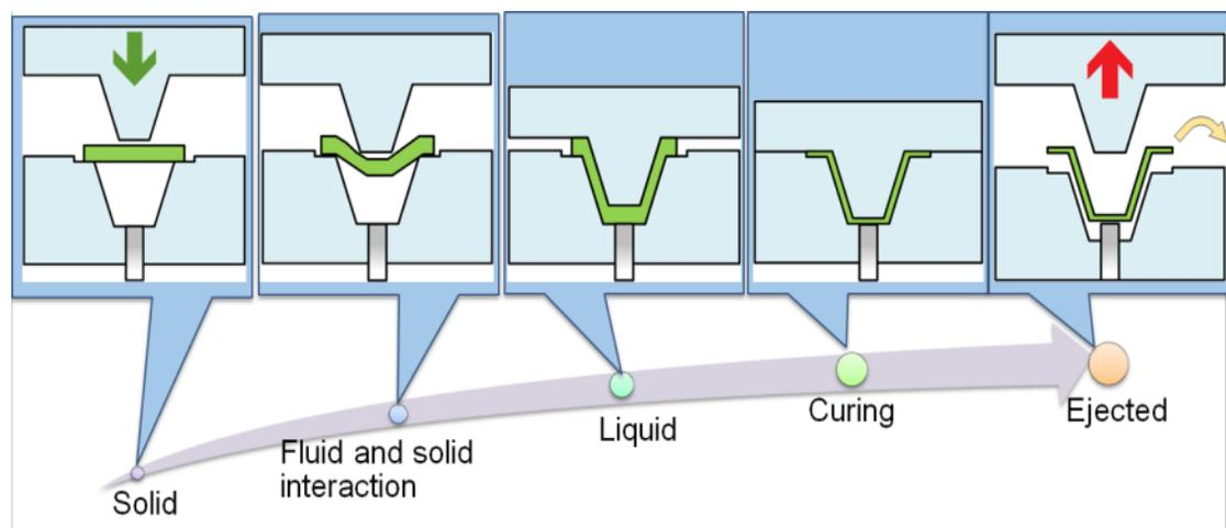
Figure 1: The compression molding process
