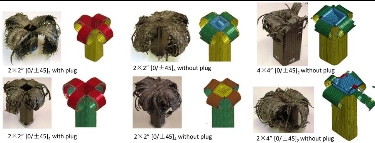
Figure 11. Comparison of predicted failure morphologies with experimental results.
