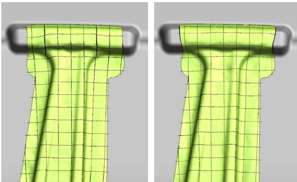
Figure 11: Comparison of deformation of automotive B-pillar of  $[(0/90)]_4$  and  $[(45/-45)]_4$  lay-ups.
