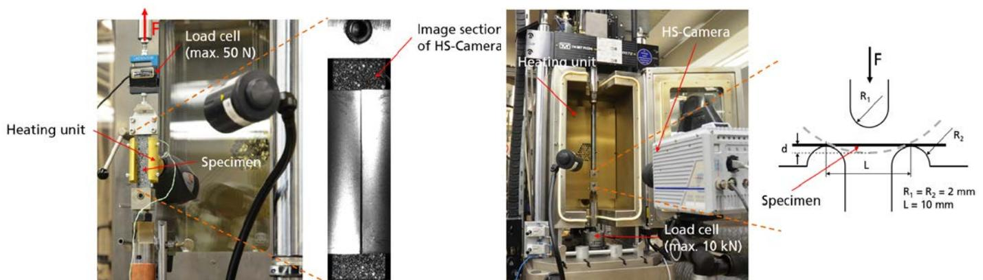
Figure 4: Setups for uniaxial tension and bias extension (left) and 3-point bending (right) at high temperatures.
