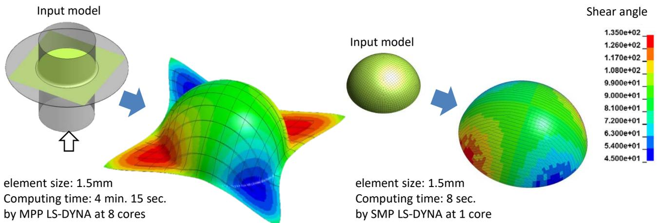
Figure 12: Comparison of incremental (shell-membrane model) and one-step inverse (shell) simulations.
