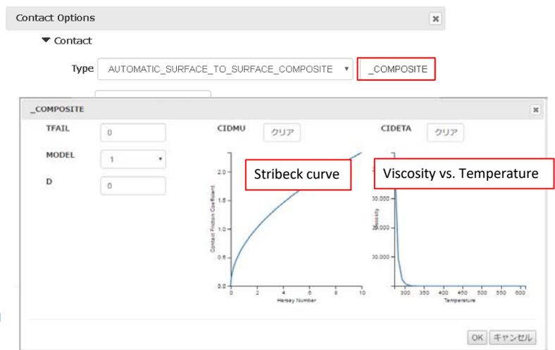
Figure 9: Stribeck curve (left) and UI to define the inter-laminar friction in Form Modeler (right).
