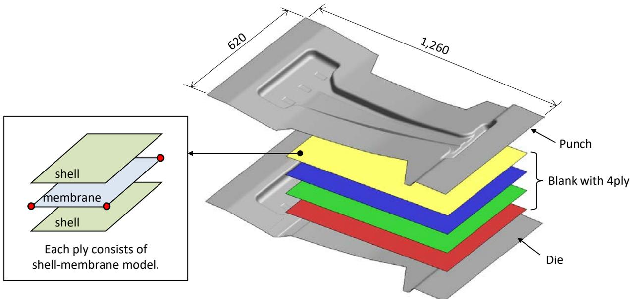
Figure 10: Automotive B-pillar forming simulation model of pre-consolidated laminate.
