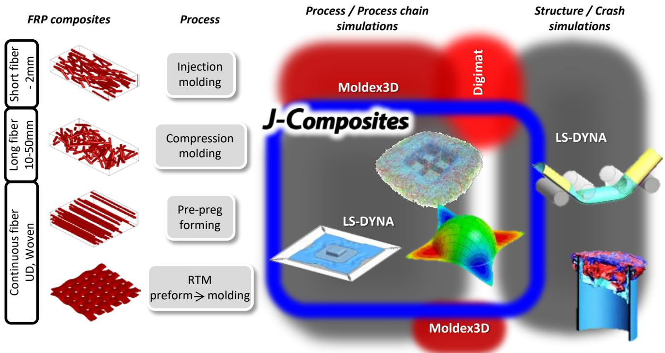
Figure 1: Overview of composite process and process-chain simulations with J-Composites.
