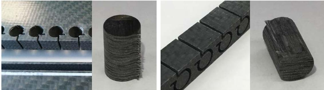
Figure 6: Sampling and specimen manufacturing: thickness direction (left) and fiber direction (right).
