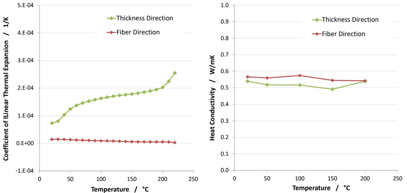
Figure 7: Coefficient of linear thermal expansion (left) and heat conductivity (right).
