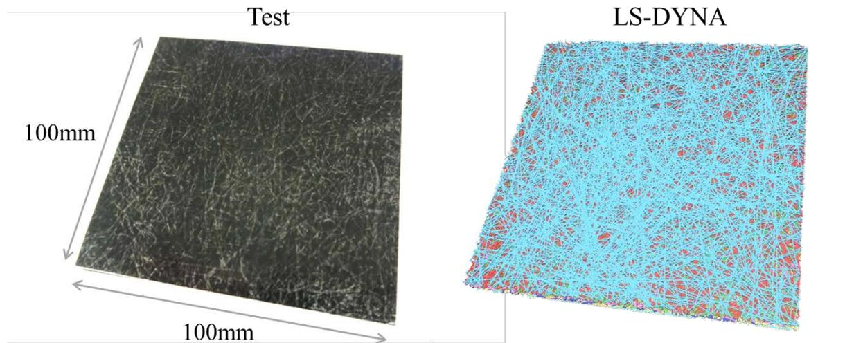
Figure 12: Long glass fiber reinforced thermoplastic sheet and LS-DYNA model
