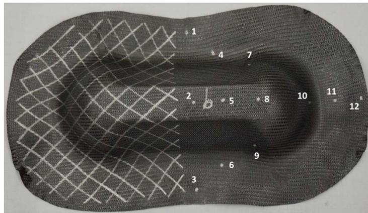
Figure 4 Preformed double dome part with initial yarn direction of  $\pm 45^\circ$
