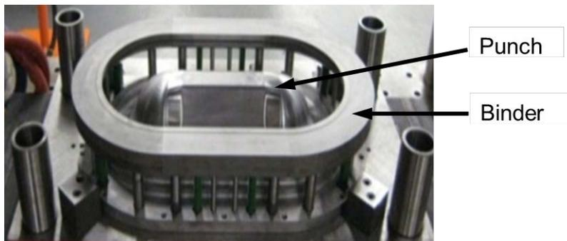
Figure 2: Experimental setup for the double dome test
