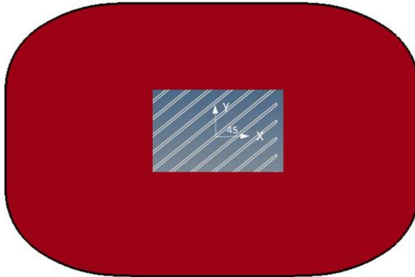
Figure 3: The initial blank shape with  $\pm 45^\circ$  prepeg layout
