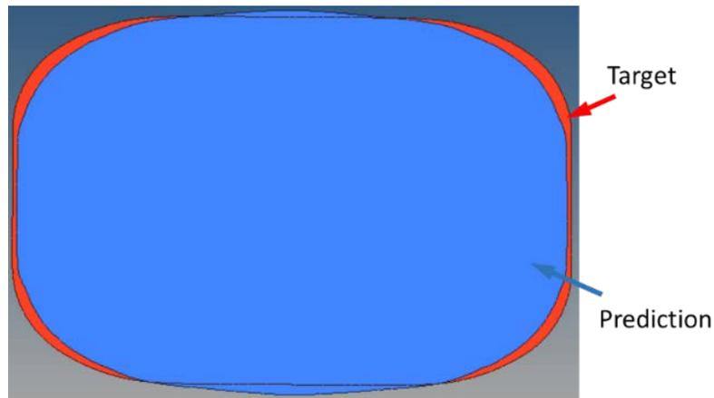
Figure 5: Comparison of the initial blank shape between the experiment and prediction
