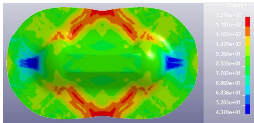
Figure 6: Predicted yarn angle distributions after preforming
