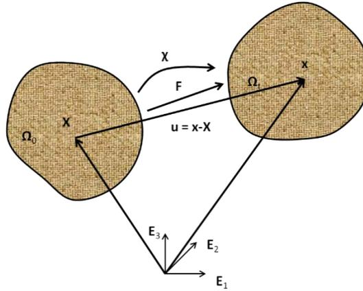
Figure 1: A carbon-fiber composite body deforms from  $\Omega_0$  to  $\Omega_t$  (F is the deformation gradient tensor)
