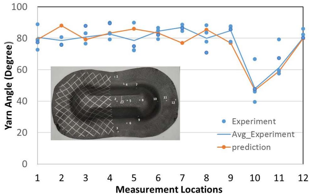
Figure 7: Comparison of experiment and predicted yarn angle at selected locations
