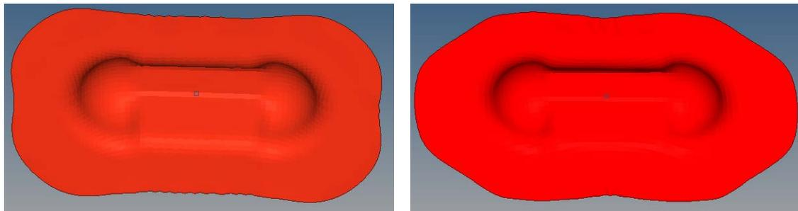
a) 0/90° prepreg layout      b) ±45° prepreg layout
