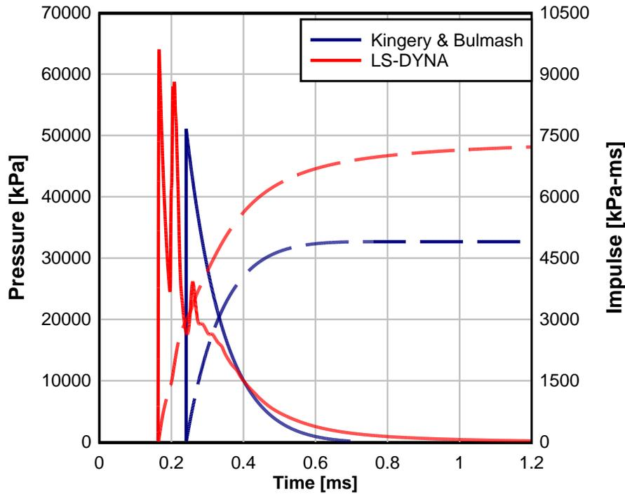
Figure 3: Comparison of waveforms from Kingery & Bulmash with high fidelity LS-DYNA result.
