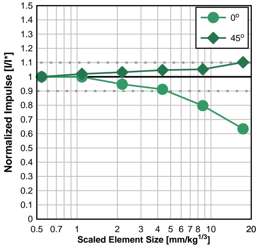
Figure 10: Comparison of normalized impulse along axis (0°) and diagonal (45°) of mesh.
