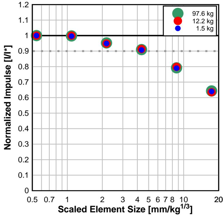
Figure 6: Normalized impulse versus scaled element size for each charge mass.
