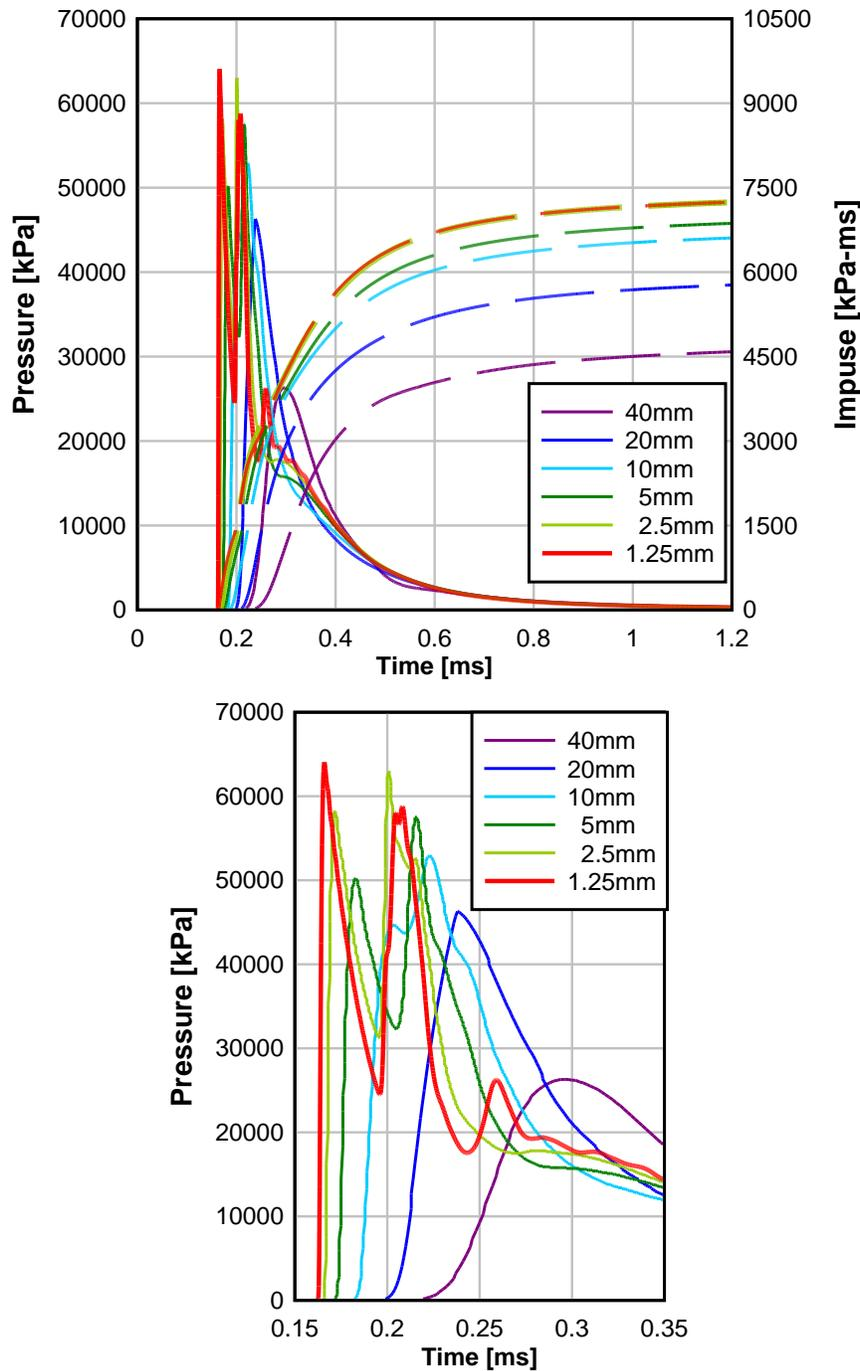
Figure 4: Pressure and impulse histories at a point opposite the charge on a reflecting wall (2-D axisymmetric).
