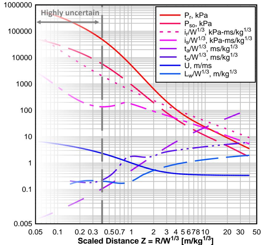
Figure 1: Kingery & Bulmash curves for positive phase shock wave parameters for a spherical TNT explosion.
