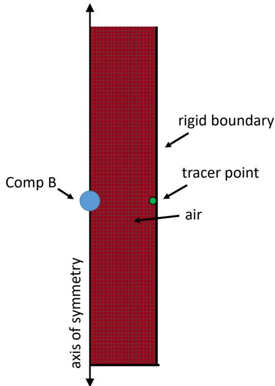
Figure 2: 2-D axisymmetric mesh for simulation of HE detonation
