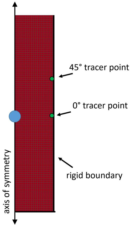
Figure 9: 2-D axisymmetric mesh showing the location where impulses were recorded.
