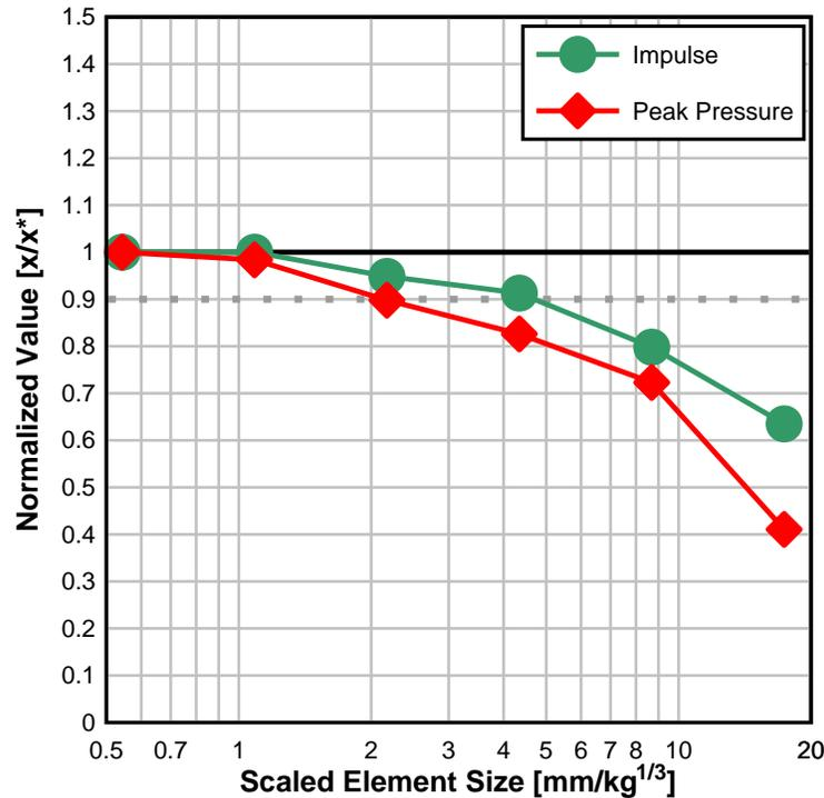
Figure 5: Normalized peak pressure and impulse vs scaled element size for 12.2 kg Comp B at a 0.762 m standoff.
