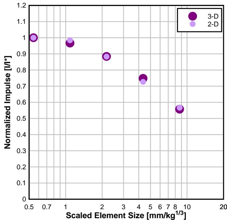
Figure 12: Comparison of mesh convergence for 2-D and 3-D simulations.
