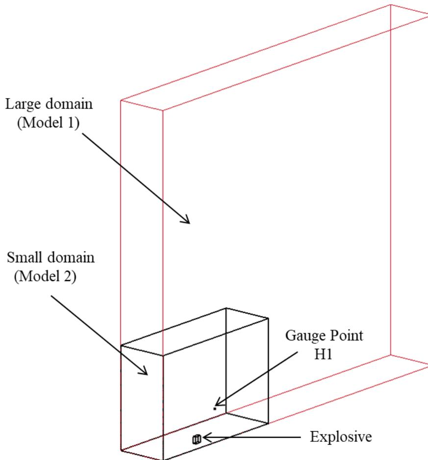
Figure 3: Two finite element model domains for the Dead End configuration.
