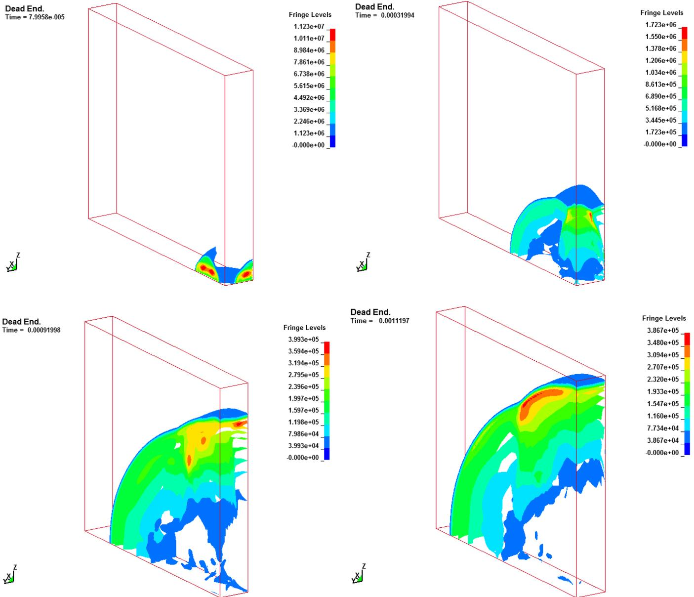
Figure 4: Pressure contour plots, Dead End configuration, Model 1 (large domain).
