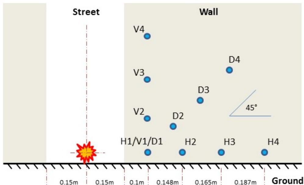
Figure 2: Schematic of experimental set-up and gauge locations.
