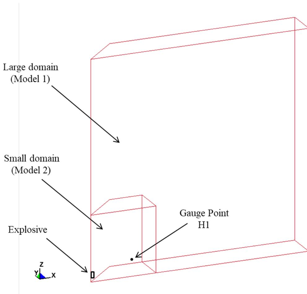
Figure 6: Two finite element model domains for the Crossroads configuration.
