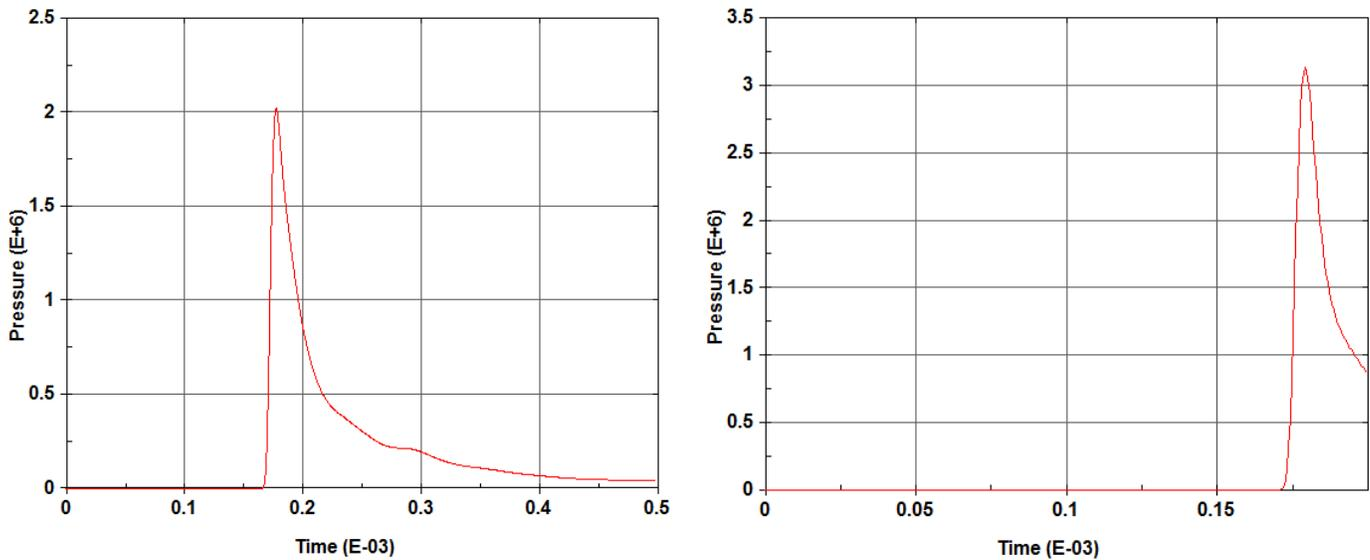
Figure 5: Pressure histories at point H1 from Model 1 (left) and Model 2 (right).
