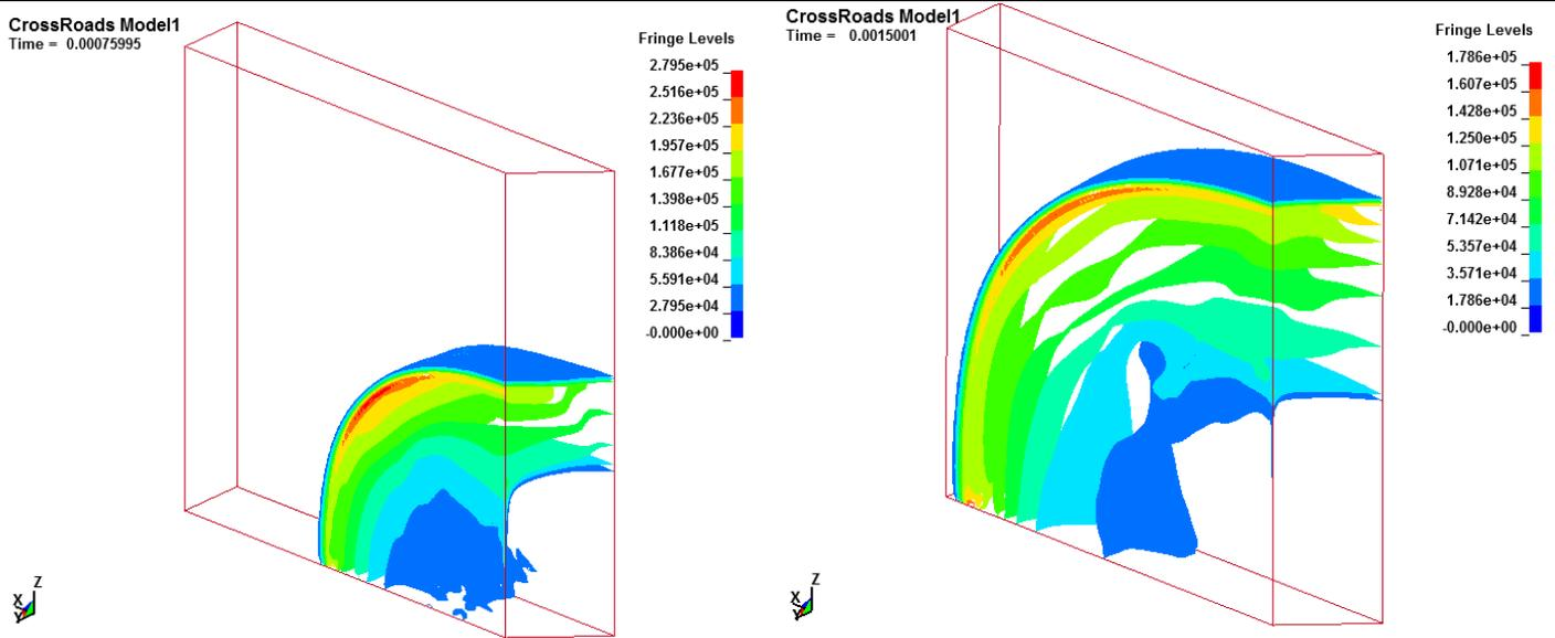
Figure 7: Pressure contour plots, Crossroads configuration, Model 1 (large domain).
