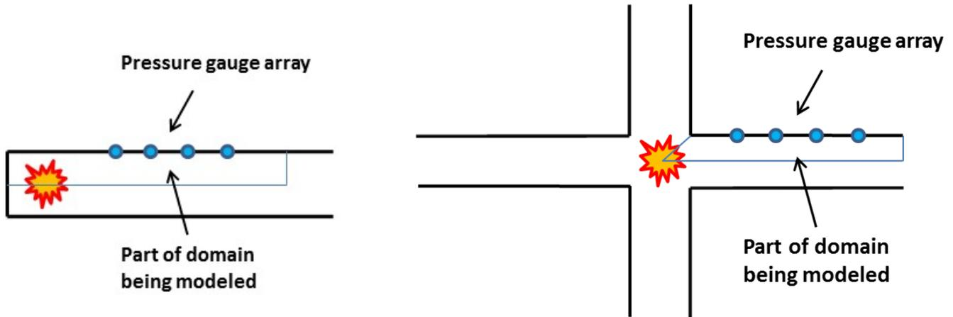
Figure 1: Schematic of the two test configurations for blast in an urban environment: Dead End (left) and Crossroads (right).
