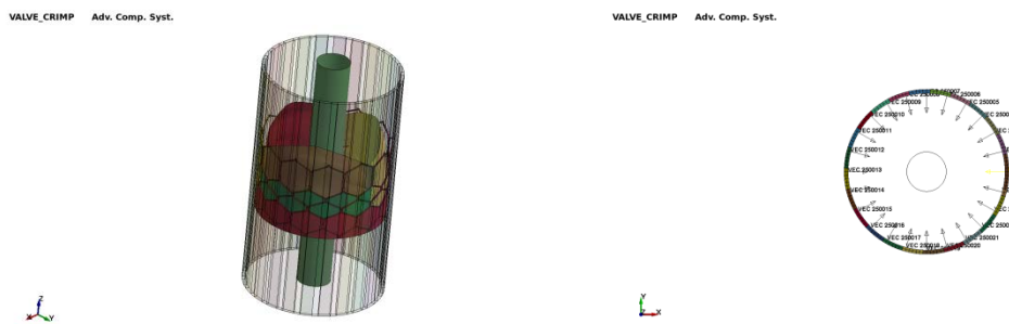
Figure 8. Crimping Device Approximation and radial movement of the strips.
