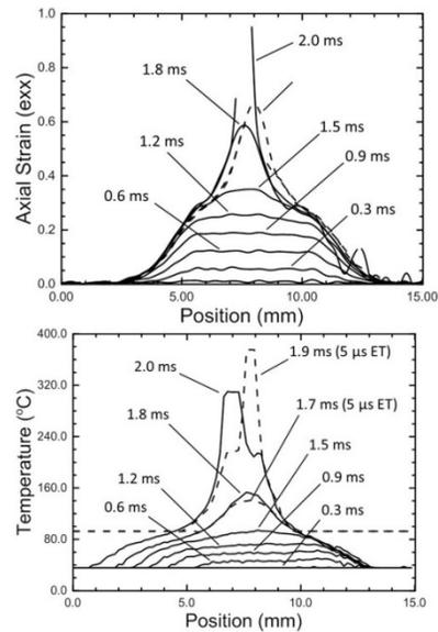
Figure 2: Strain and temperature along the center line of the specimen.
