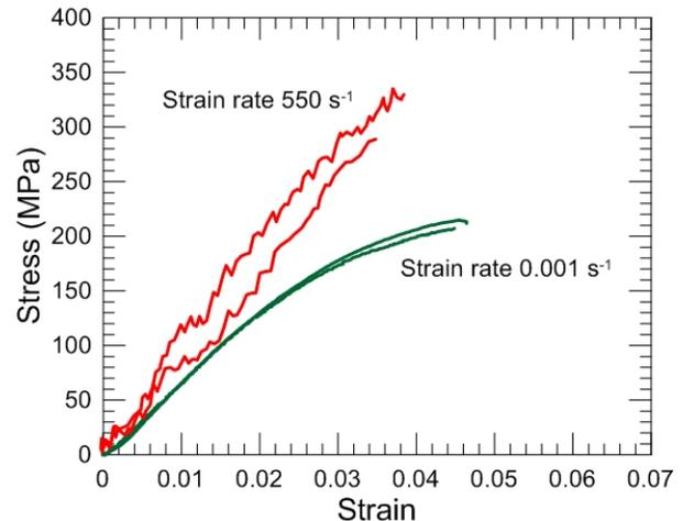
Figure 9: Compression stress strain curves of T800/F3900 composite in the 90° direction.
