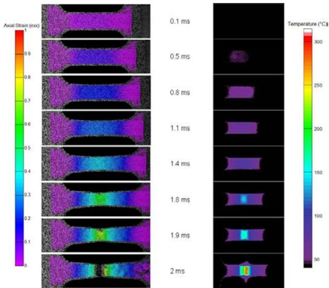
Figure 1: DIC and IR images from tensile test of 316 stainless steel at strain rate of  $200 \text{ s}^{-1}$ .
