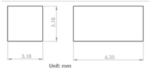
Figure 5: Compression specimen geometry.
