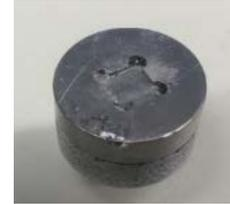
Figure 6: Titanium platens
