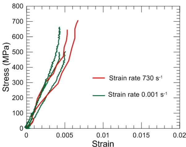
Figure 8: Compression stress strain curves of T800/F3900 composite in the 0° direction.
