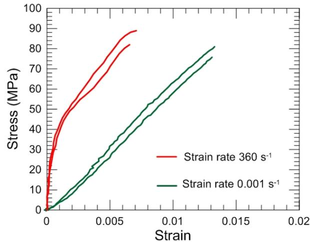
Figure 10: Tension stress strain curves of T800/F3900 composite in the 90° direction.
