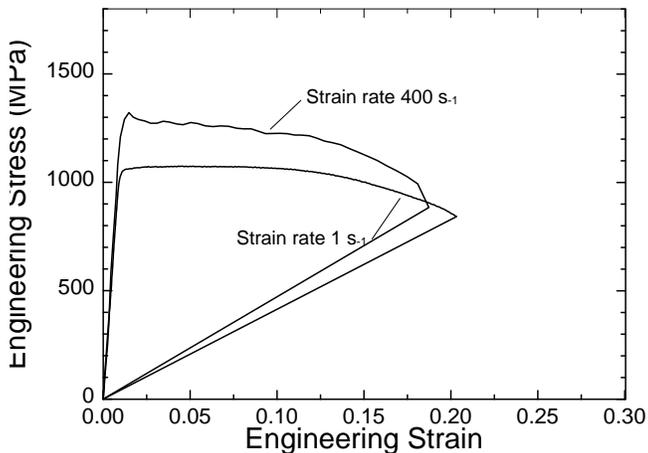
Figure 3: Tensile engineering stress strain curves of Ti-6Al-4V at strain rates of 1 and  $200 \text{ s}^{-1}$ .
