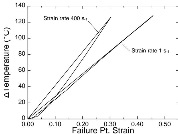
Figure 4: Temperature at the failure point as a function of strain.
