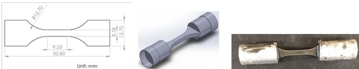
Figure 7: Tensile specimen geometry (left), specimen with adaptors (middle), photo (right).
