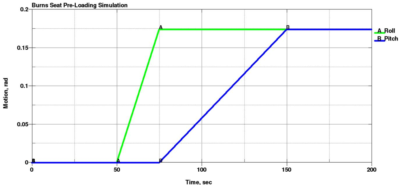
Fig 4. Roll and Pitch motion as applied to seat mounts
