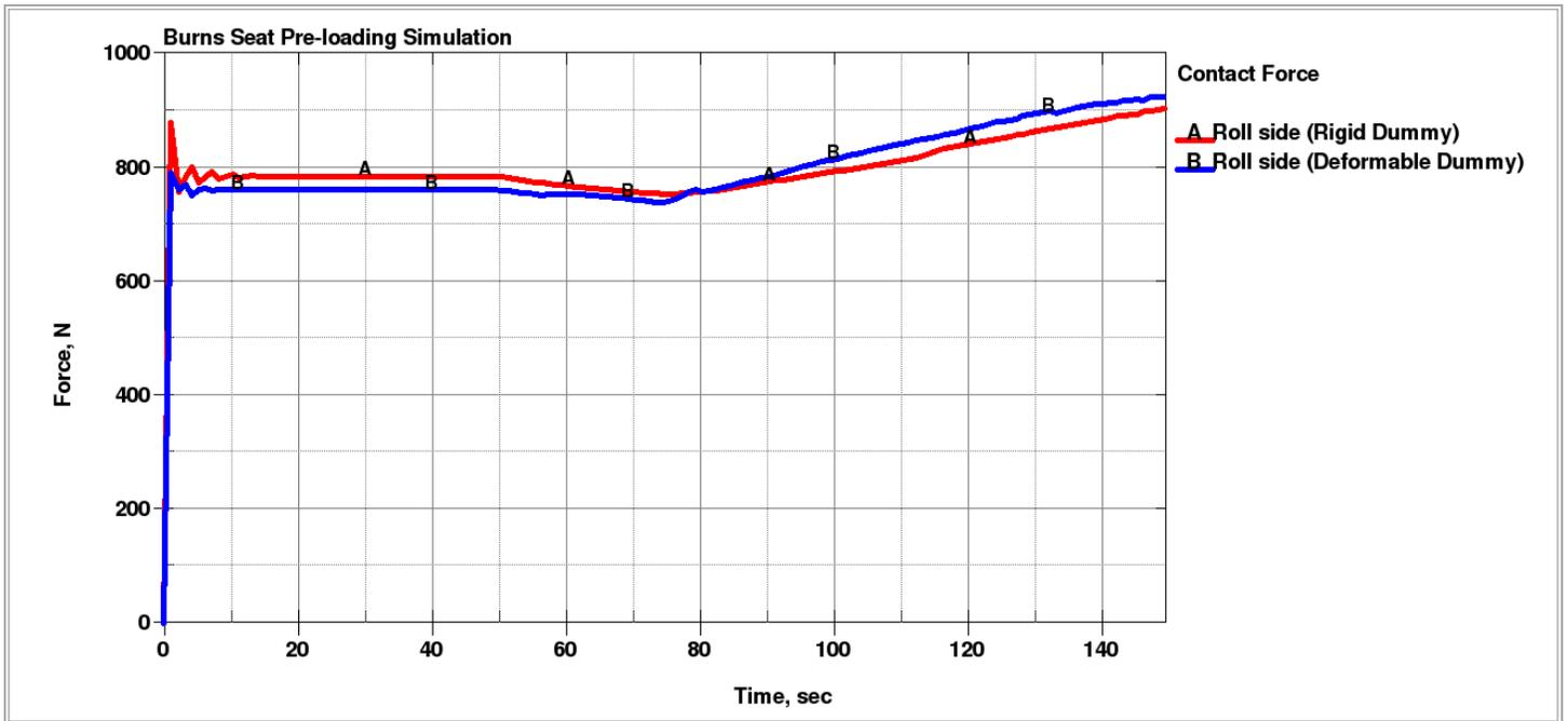
Fig 8. Contact force between the dummy and seat on the roll side
