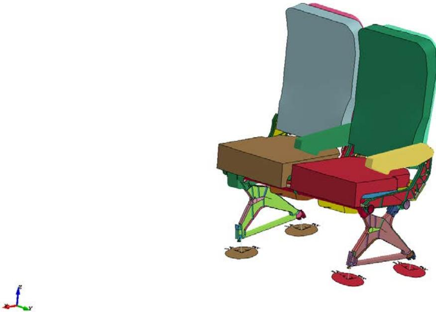
Fig 5. Seat Only subjected to pre-loading as integrity test
