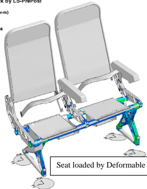
Seat loaded by Deformable Dummy
