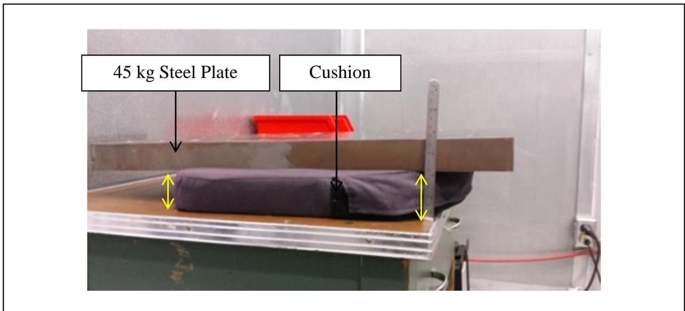
Figure 5: Compression Test Setup
