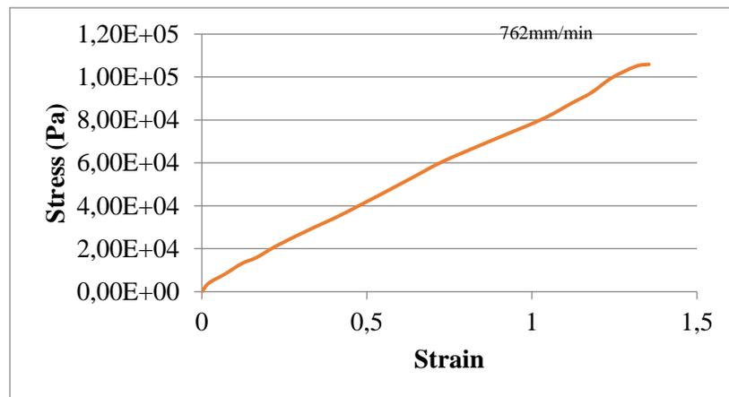
Figure 3: HS-70 Ethafoam Stress-Strain Curve
