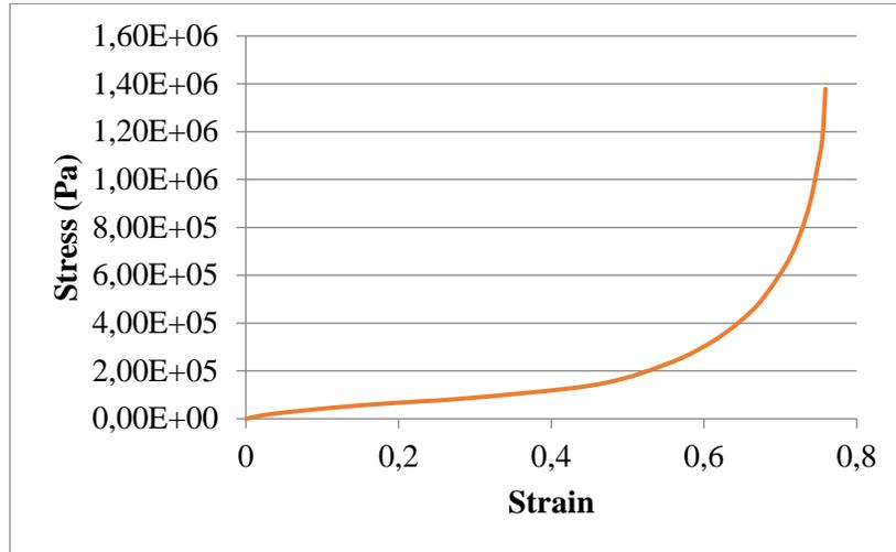
Figure 2: T41 Temperfoam Stress-Strain Curve
