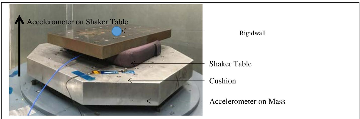
Figure 7: Shaker Table Setup
