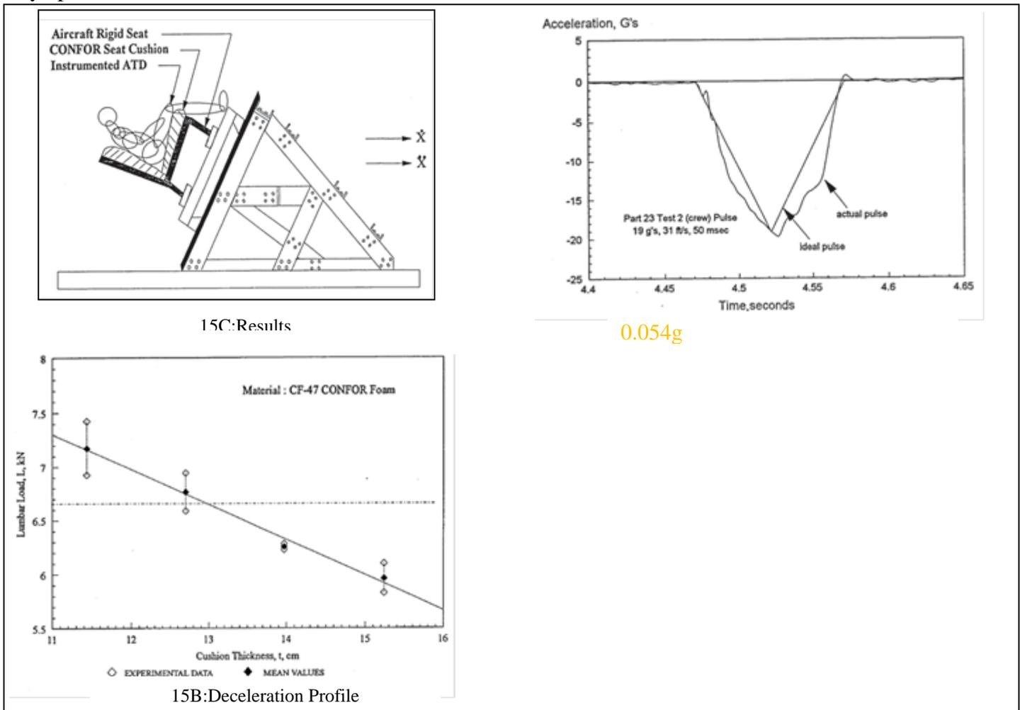
Figure 15: 14-Code of Regulations Part 230 Air wothiness Standard Test
