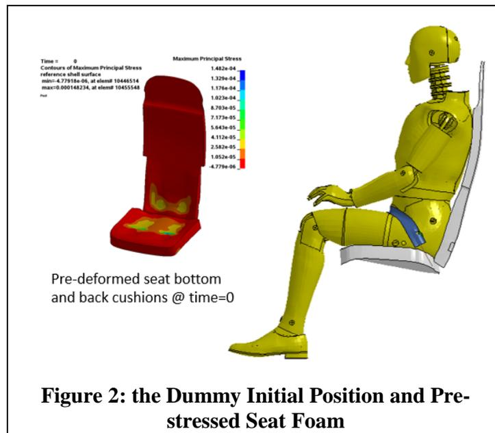
Boundary conditions are applied such that the floor and seat track fixtures are constrained in all degrees of freedom. But, a 16G force input is imposed on the full seat/dummy model. This force was applied as the ideal triangular pulse shown in Figure 3 using \*LOAD\_BODY\_X.
