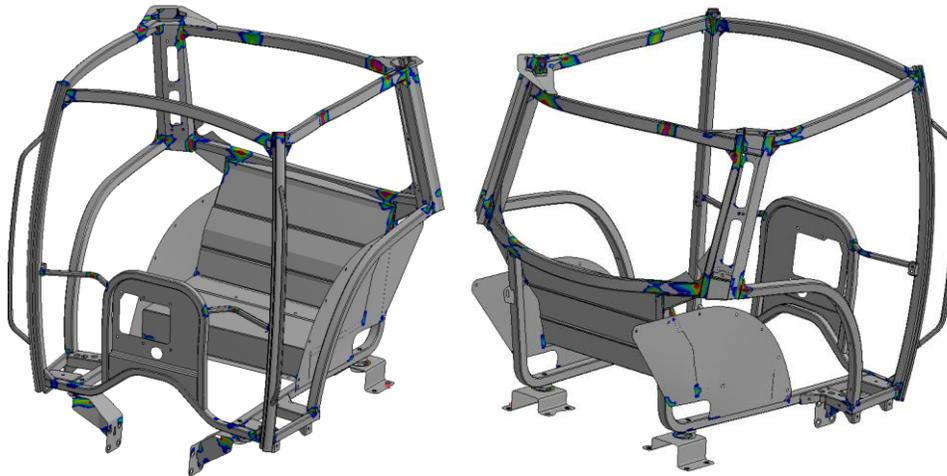
Fig.27 Front crushing. Grey: elastic region areas. Colored: main plastic strain areas.
