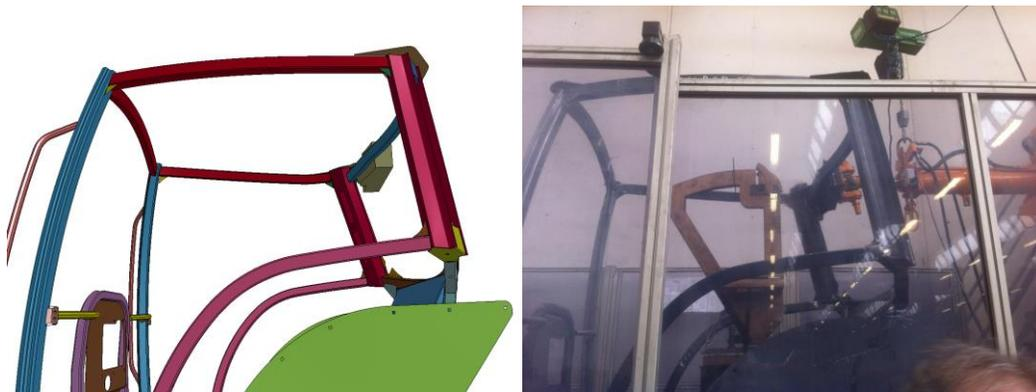
Fig.14 Numerical ROPS prediction vs real test for longitudinal loading @ 6.16 kJ
