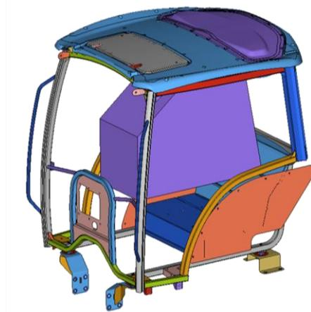
Fig.2 CAD model of the tractor showing the protective structure FOPS.
