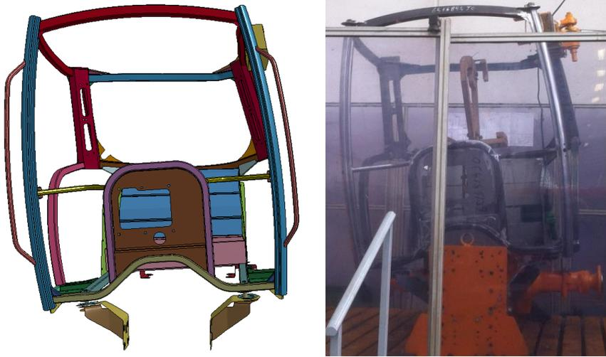
Fig.22 Numerical vs experimental side loading test
