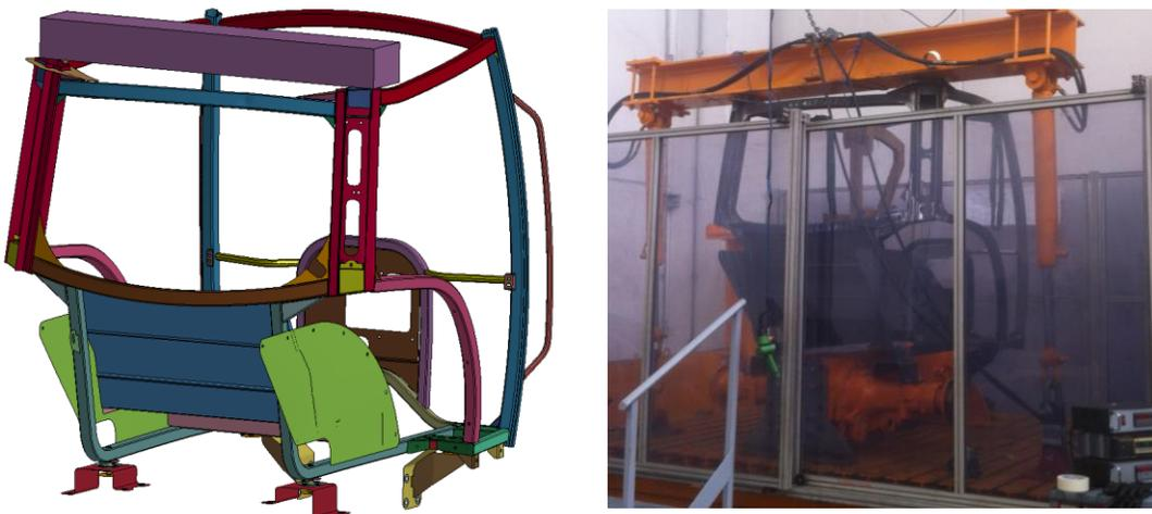
Fig.19 Numerical vs experimental rear crushing test
