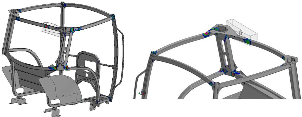
Fig.16 Longitudinal loading. Grey: elastic region areas. Colored: main plastic strain areas.
