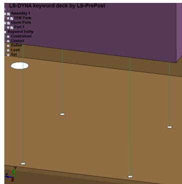
Fig.8 Mesh detail showing the anchoring points of the clearance zone
