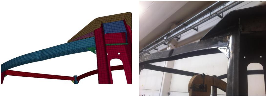
Fig.18 Numerical deformation vs experimental test after the longitudinal test
