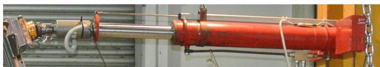
Fig.12 Hydraulic piston and respective rotation due to the universal joint
