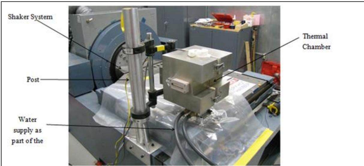
Figure 2: Thermal chamber supporting posts
