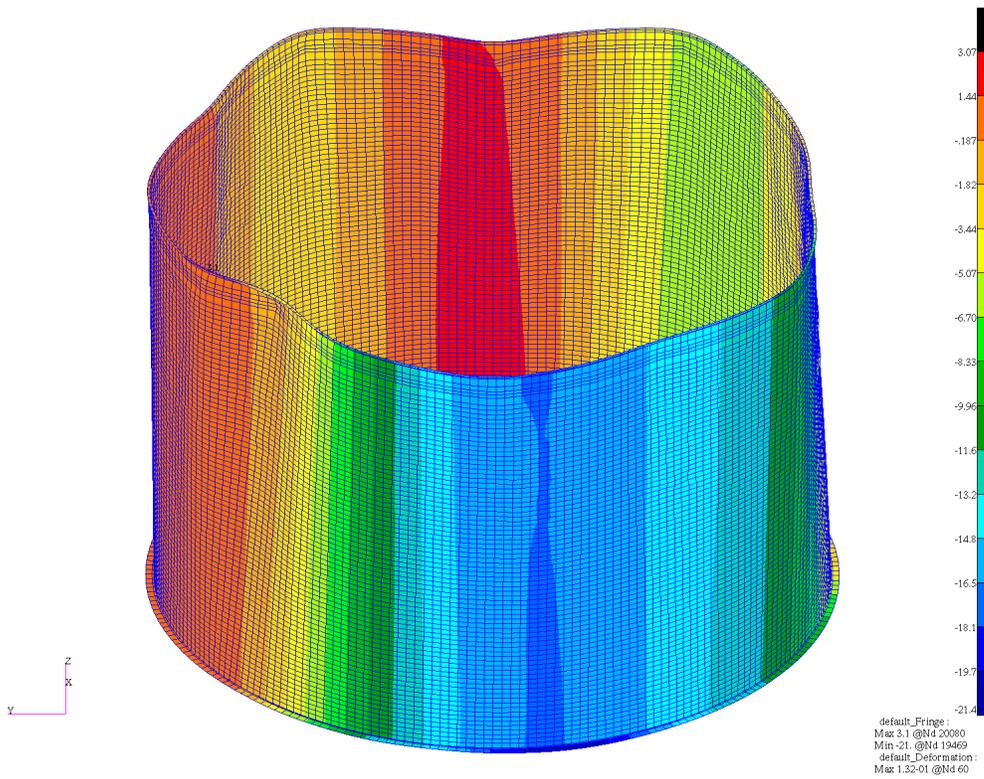
Figure 6: Analysis A - vertical deflection [mm]
