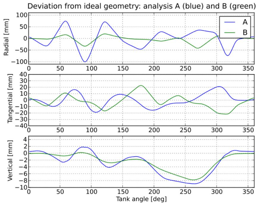
Figure 9: Component deviations from ideal shape at top of tank
