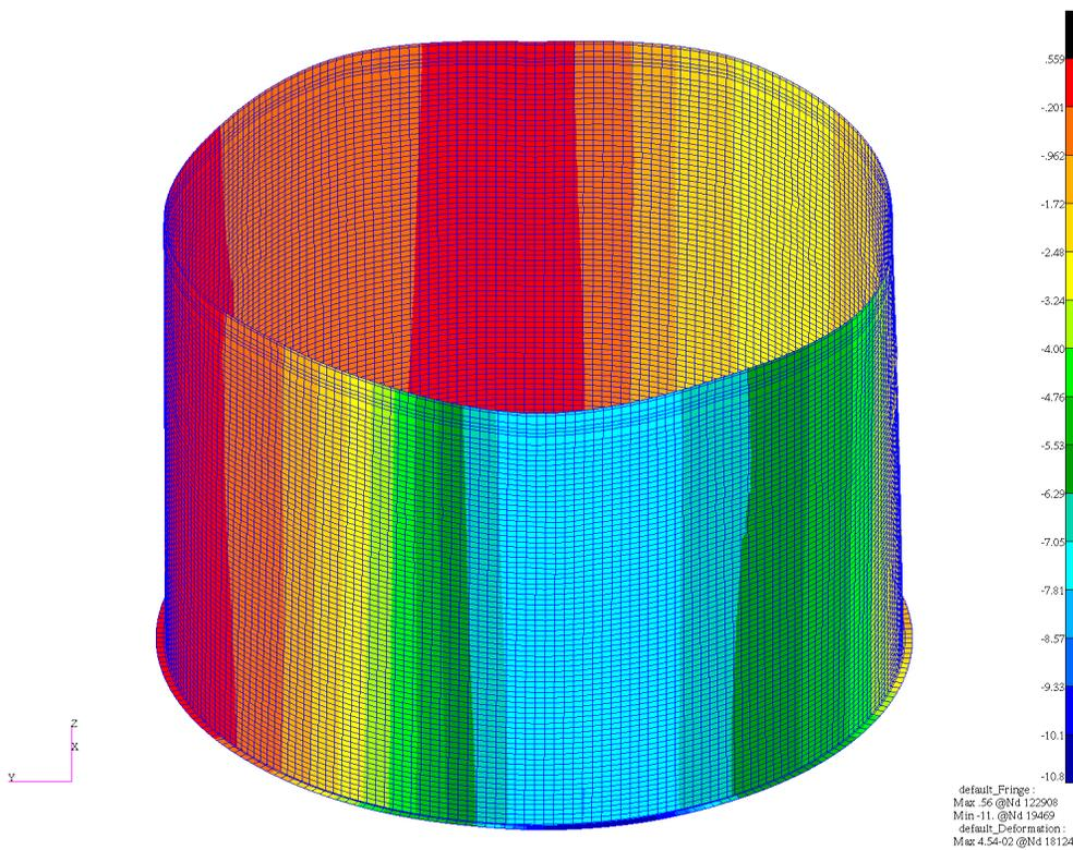
Figure 7: Analysis B - vertical deflection [mm]
