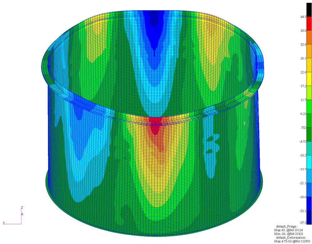
Figure 4: Analysis B - radial deflection [mm]
