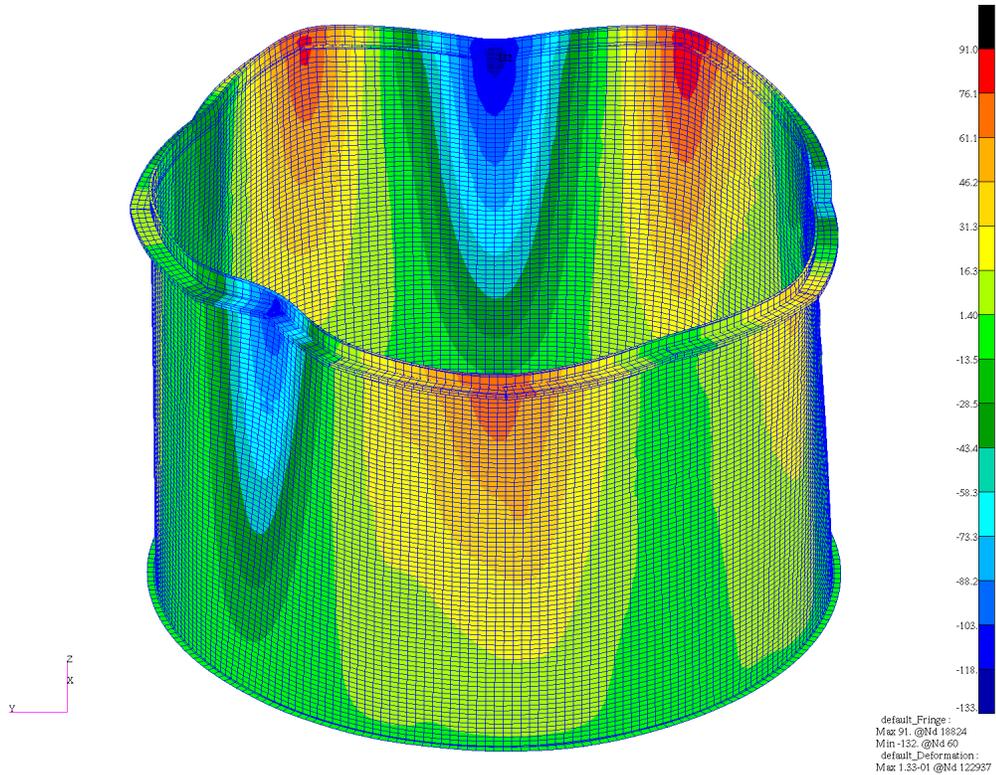
Figure 5: Analysis A - radial deflection [mm]
