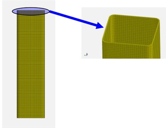
Figure 11 Model set up for crush box, one layer of mesh over thickness
