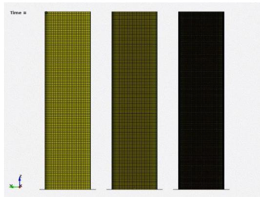
Figure 12 Model discretization with 4mm, 2mm, and 1mm mesh
