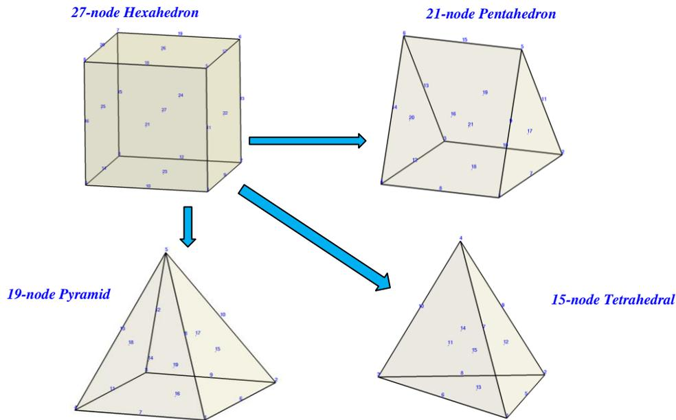
Figure 3 27-node Hexahedron element and degenerated 21-node pentahedron, 19-node pyramid, and 15-node tetrahedron element
