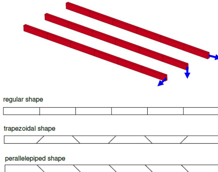
Figure 4 Straight cantilever beam test. Loading: unit forces at free end
