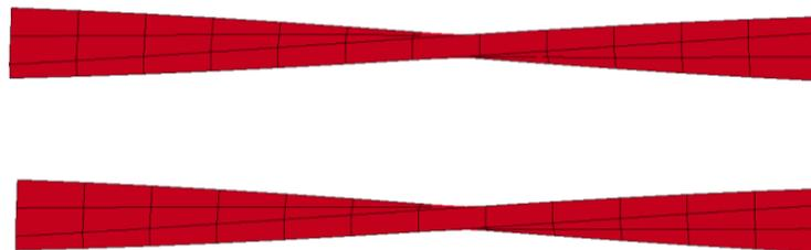
Figure 6 Twisted beam test
