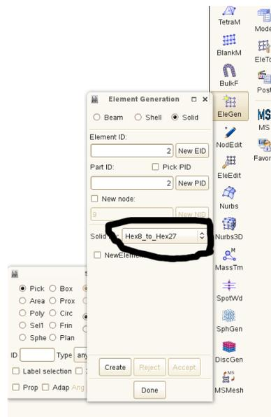
Figure 2 using LS-PrePost to transfer 8-node brick element to 27-node brick element
