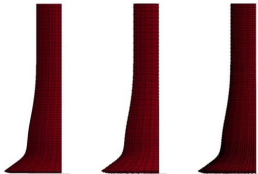
**Figure 8 Deformed model for bar impact problem using a) 972 Elform2 element b) 972 Elform24 Element c) 7776 Elform2 element**
