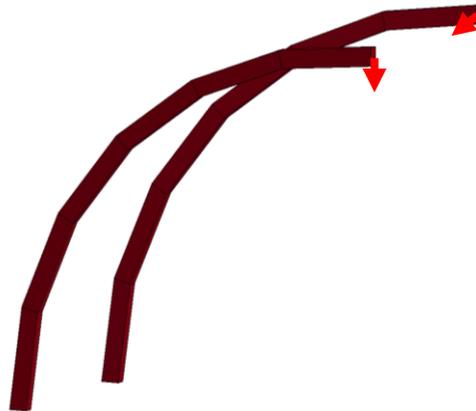
Figure 5 Curved beam test. Loading: unit forces at tip
