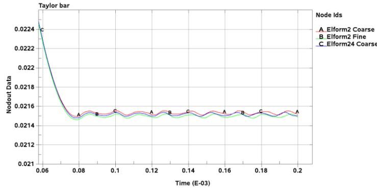
Figure 9 Displacement comparison between a) 972 Elform2 element b) 972 Elform24 Element c) 7776 Elform2 element
