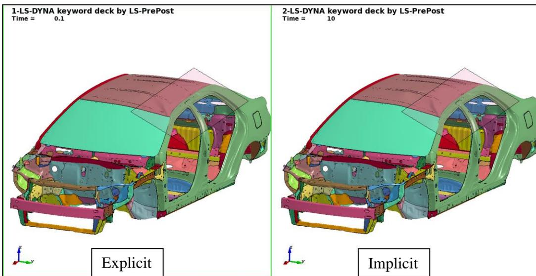
Figure 3 Final deformed state comparison
