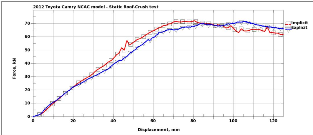
Figure 2: Force-Displacement plot
