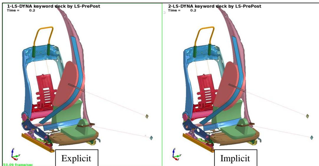
Figure 4 Final deformed state of seat structure
