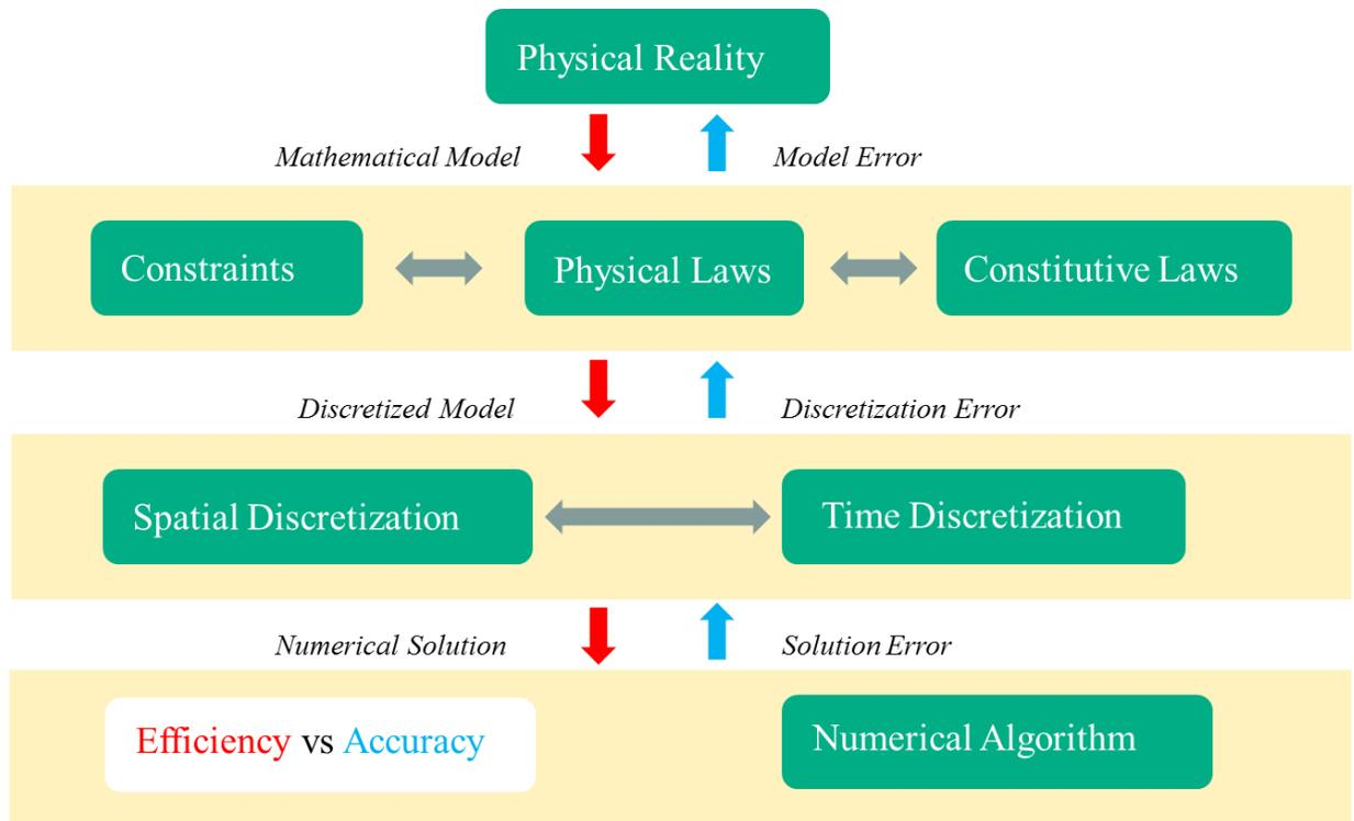
Figure 1 Numerical simulation chart
