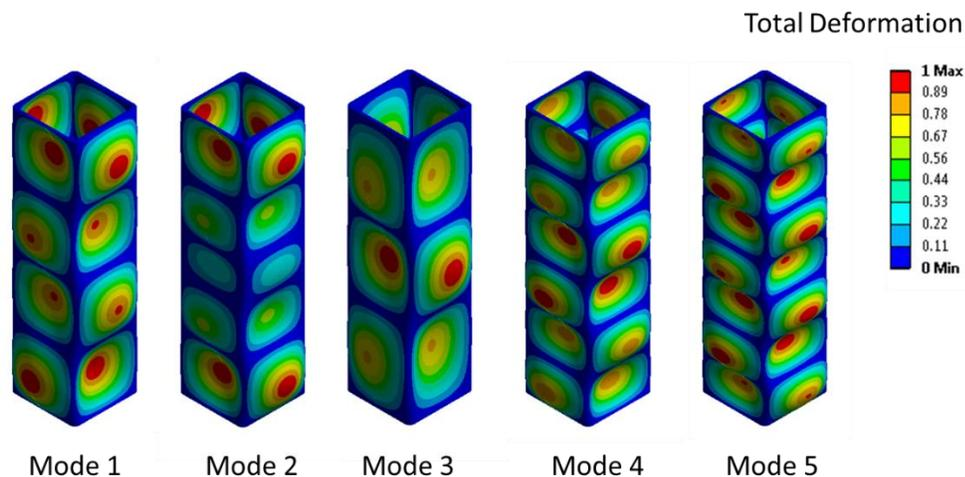
Figure 6 – Linear Buckling Mode Shapes for the tube with 3.5 mm thickness
