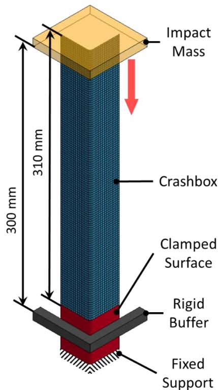
Figure 1 – Model Setup
