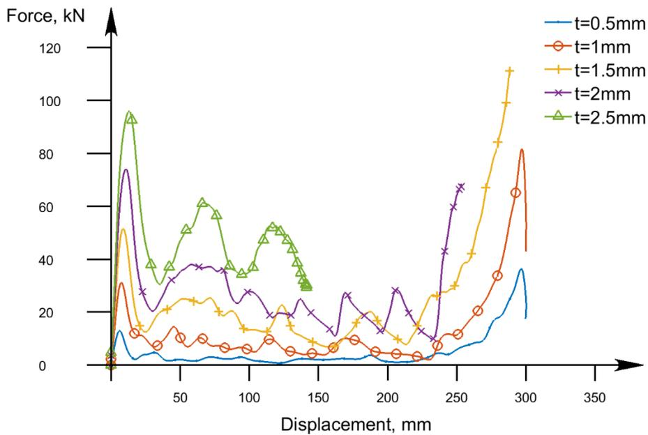
Figure 4 – Force-Deflection Curves for Thickness Variations
