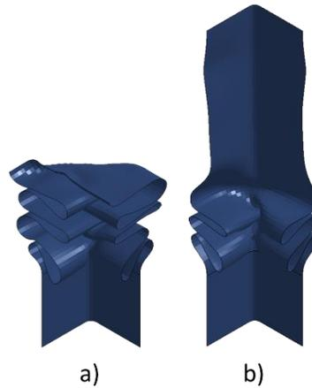
Figure 3 – Crushing Modes of the Specimens
