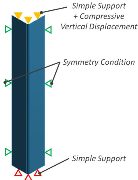
Figure 5 – Boundary Conditions for Linear Buckling Analysis
