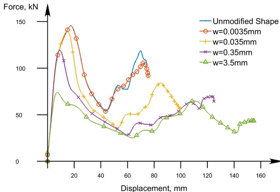
Figure 7 – Effect of Alternation Magnitude (*w*) on Force-Deflection Curves
