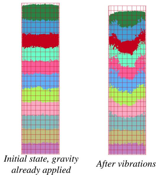
Figure 7: Gravity compaction illustration
