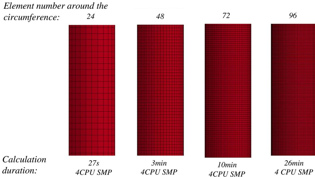
Figure 4: Mesh and performance studies with the vibratory explicit method
