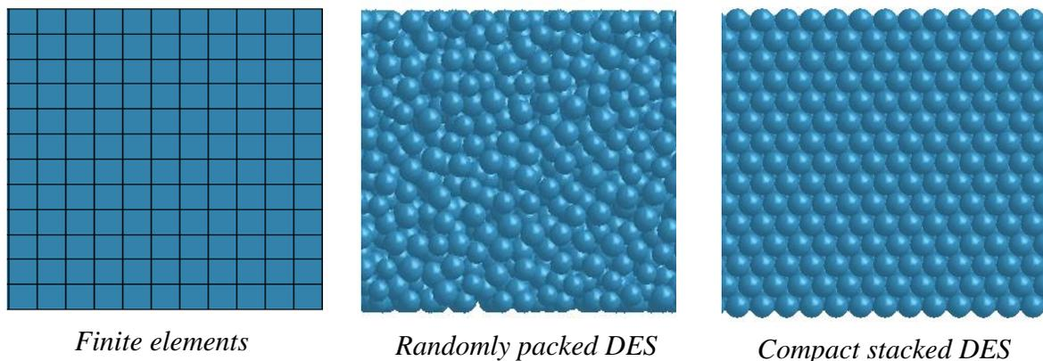
Figure 12: Finite elements and DES “mesh” illustration
