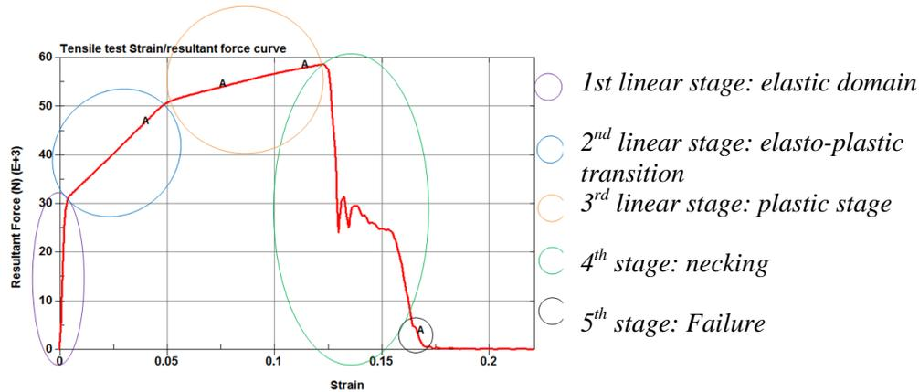
Figure 15: Description of the various stages of the compact stacked DES elasto-plastic behavior
