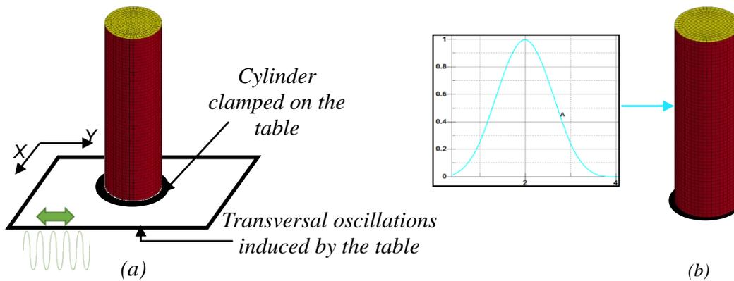
Figure 3: Load illustration for numerical mode detection: (a) transversal vibration, (b) pulse
