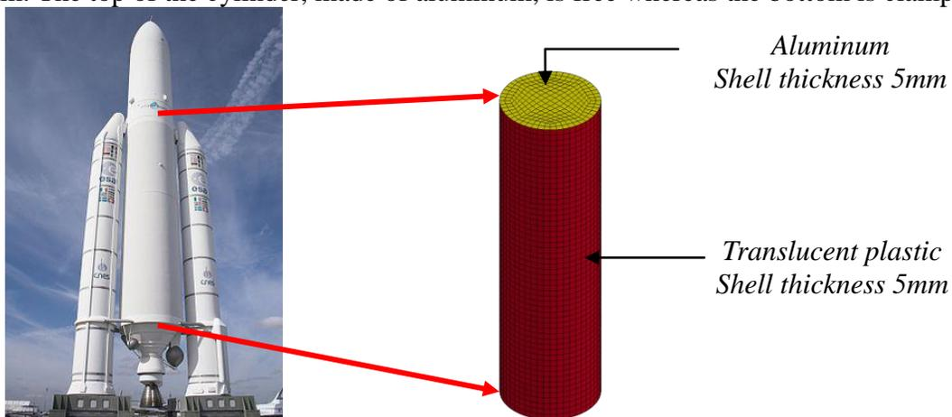
Figure 2 : Cryogenic tank simplified model
