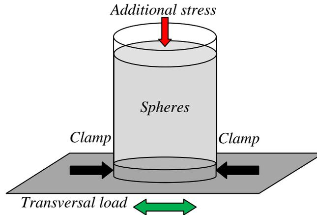
Figure 8: Illustration of the pressure used to constraint spheres and prevent their relative movements considering the vibration method
