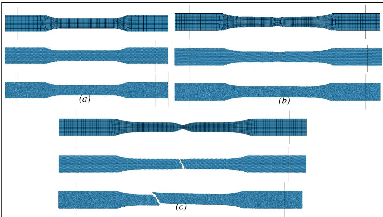
Figure 13: Screenshots of the three specimens behaviors at the initial state (a), at maximal necking (b) and at failure (c)
