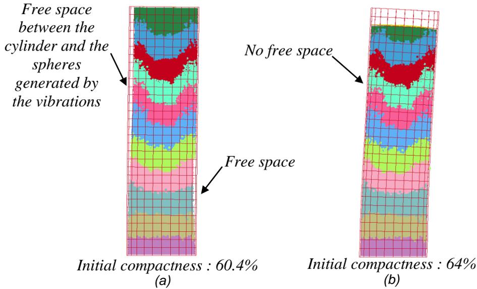
Figure 9: Comparison of the spheres behavior in the vibrating cylinder for unconstrained spheres (a) and constrained ones (b)
