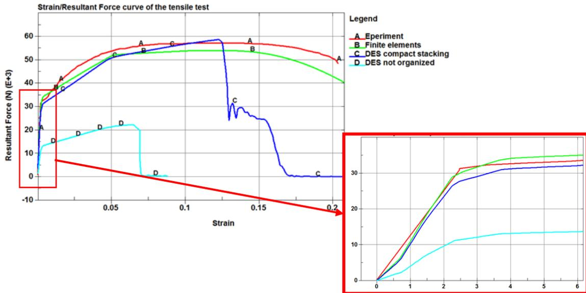
Figure 14: Force-strain curves of the experimental specimen (red), the finite elements one (green), the compact stacked DES one (dark blue) and the randomly packed DES one (light blue). The middle cross section force-displacement curves of the experimental specimen (red), the finite elements one (green), the compact stacked DES one (dark blue) and the randomly packed DES one (light blue) are drawn on the Figure 14.
