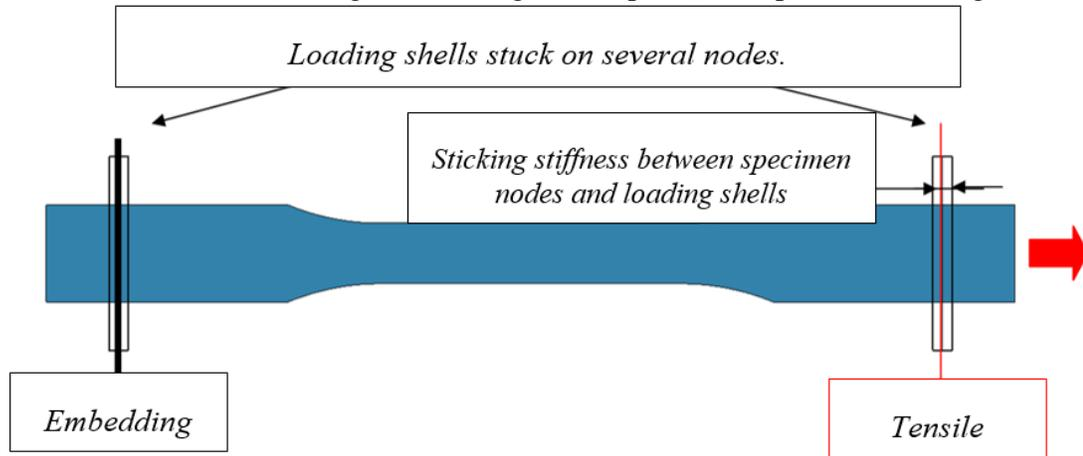
Figure 11: Boundary conditions and loads applied on every samples
