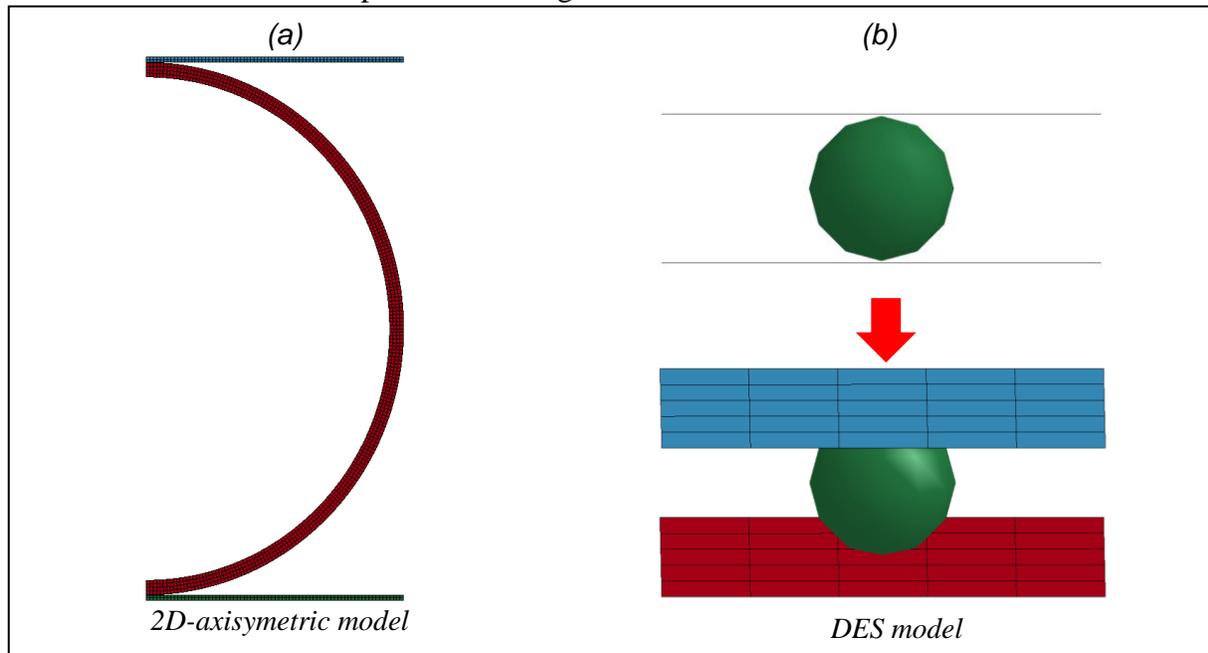
Figure 5: Compression test 2D-axisymmetric model (a) and DES model (b)
