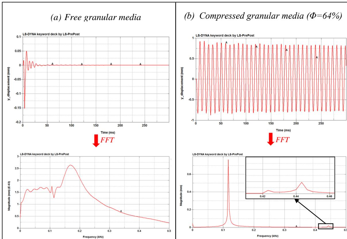
Figure 10: Time histories and associated spectrums of a cylinder filled with unconstrained (a) and compressed (b) spheres
