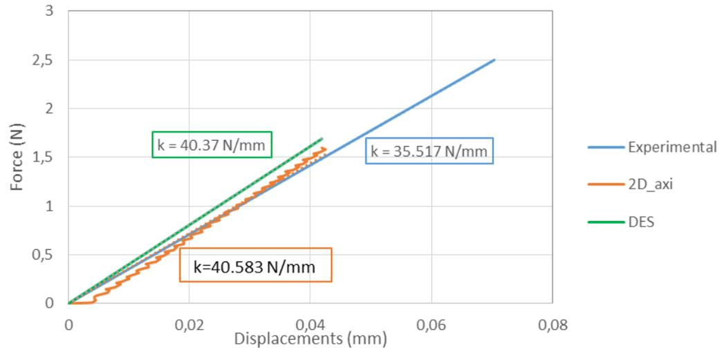
Figure 6: Force-displacement curve of the experimental (blue), hollow 2D-axisymmetric (red) and full DE (green) spheres for small strains
