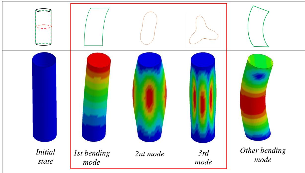
Figure 1 : Mode shapes illustration and specification of the three researched ones (red frame) obtained by an implicit calculation
