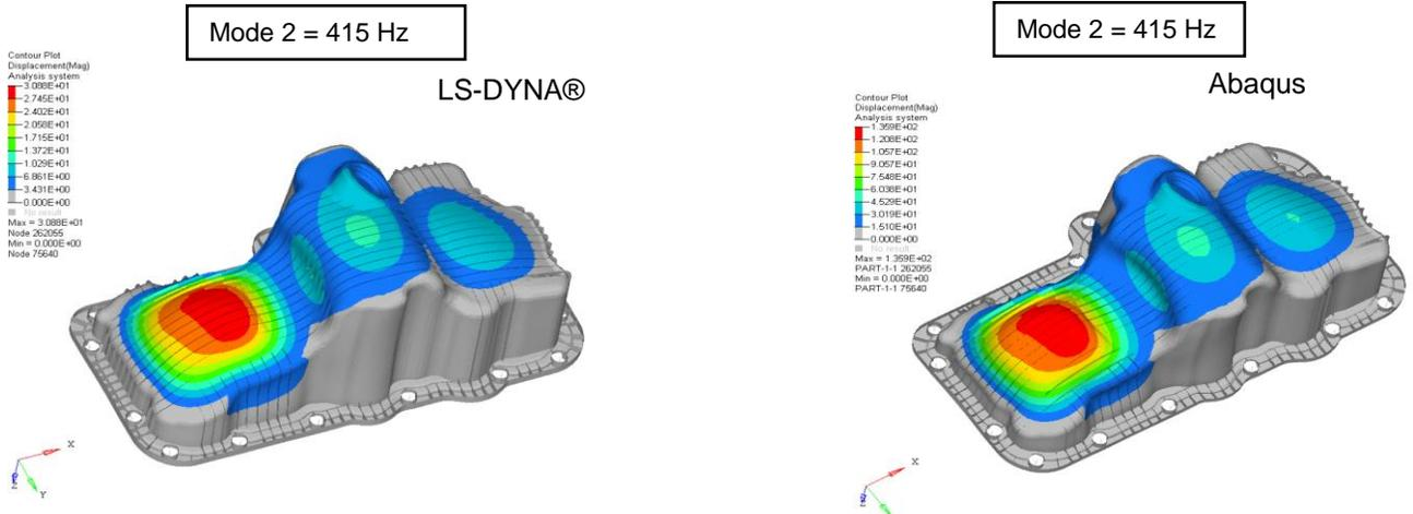
Figure 3 Mode Shape & Frequency for Mode 2
