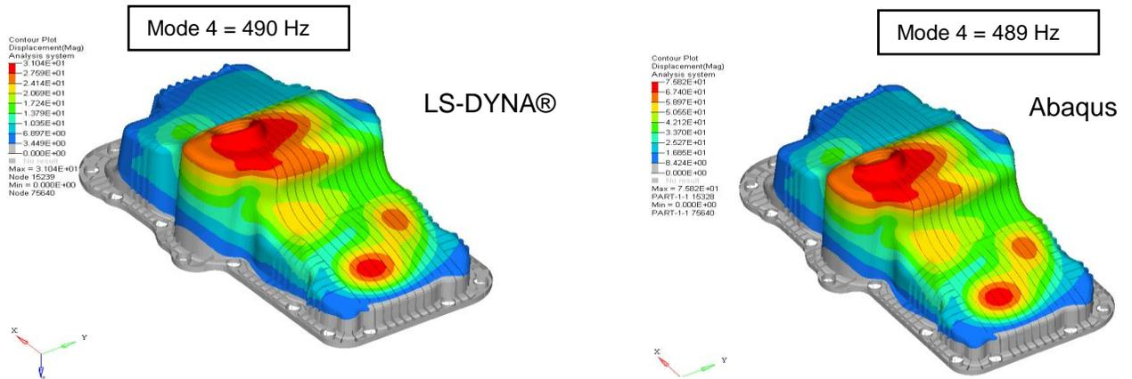
Figure 5 Mode Shape & Frequency for Mode 4
