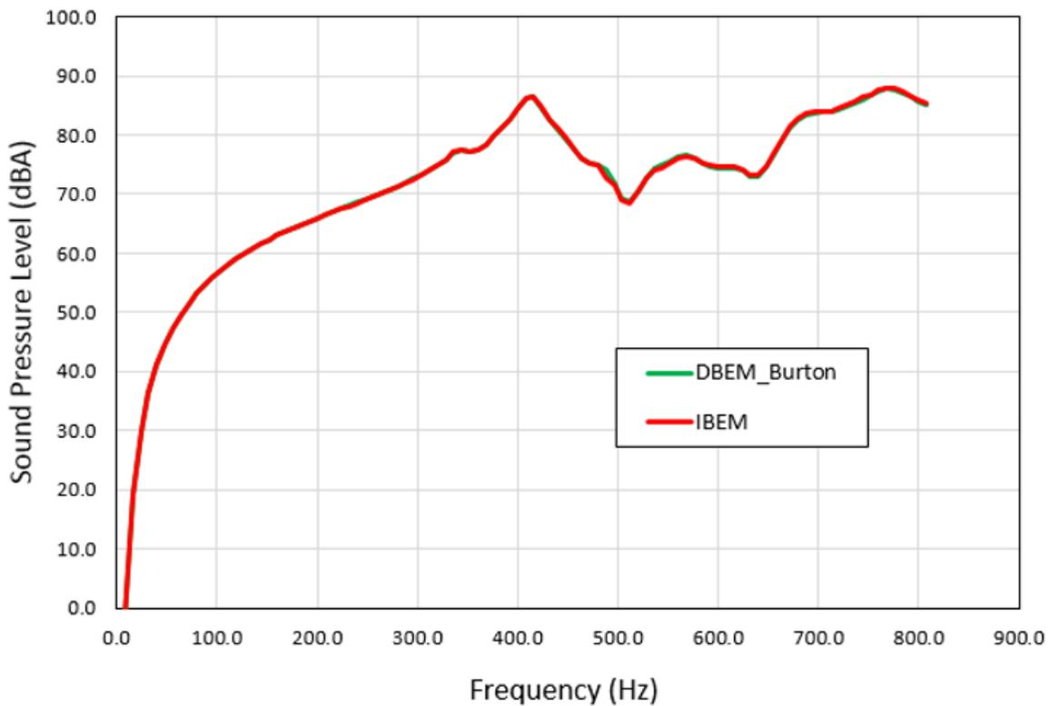
Figure 10 Sound Pressure Level (dBA) at 1/2 meter above Oil Pan
