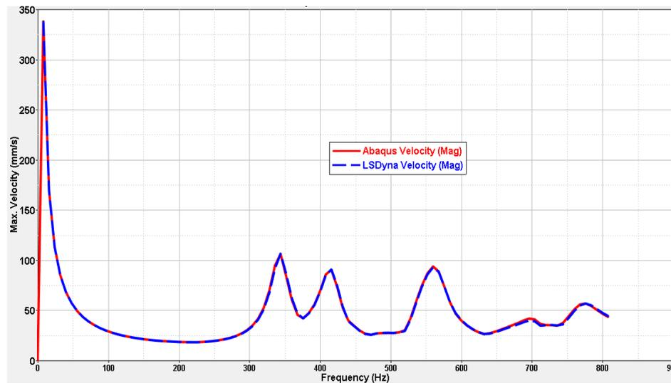
Figure 7 Comparison of Max. Velocity (amplitude) across the frequency range
