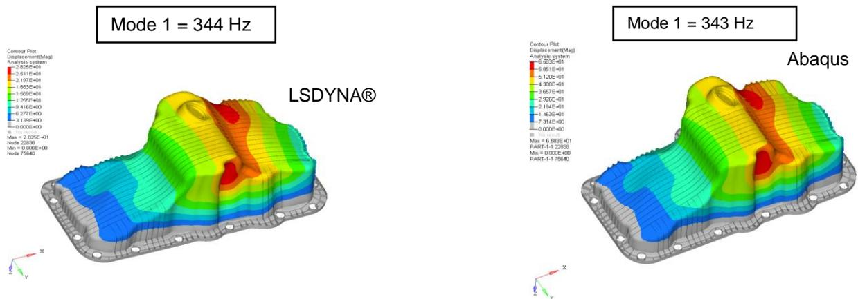
Figure 2 Mode Shape & Frequency for Mode 1
