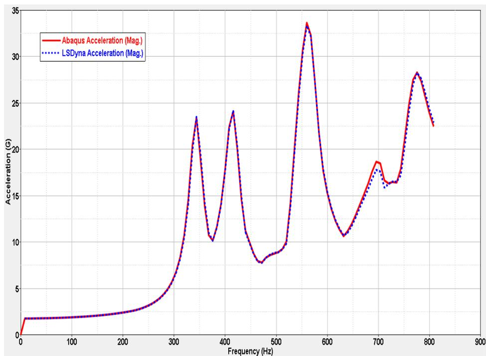
Figure 8 Comparison of Max. Acceleration (amplitude) across the frequency range
