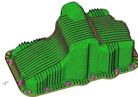
Figure 1 Plastic Oil Pan made of Ultramid® A3WG7 (Glass Reinforced Polyamide 66)
