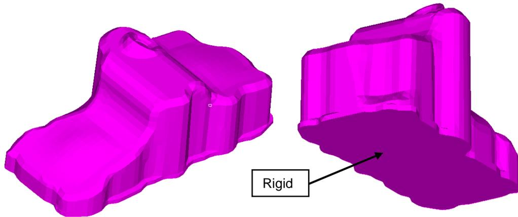
Figure 9 Boundary element model of oil pan
