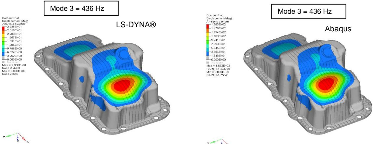
Figure 4 Mode Shape & Frequency for Mode 3
