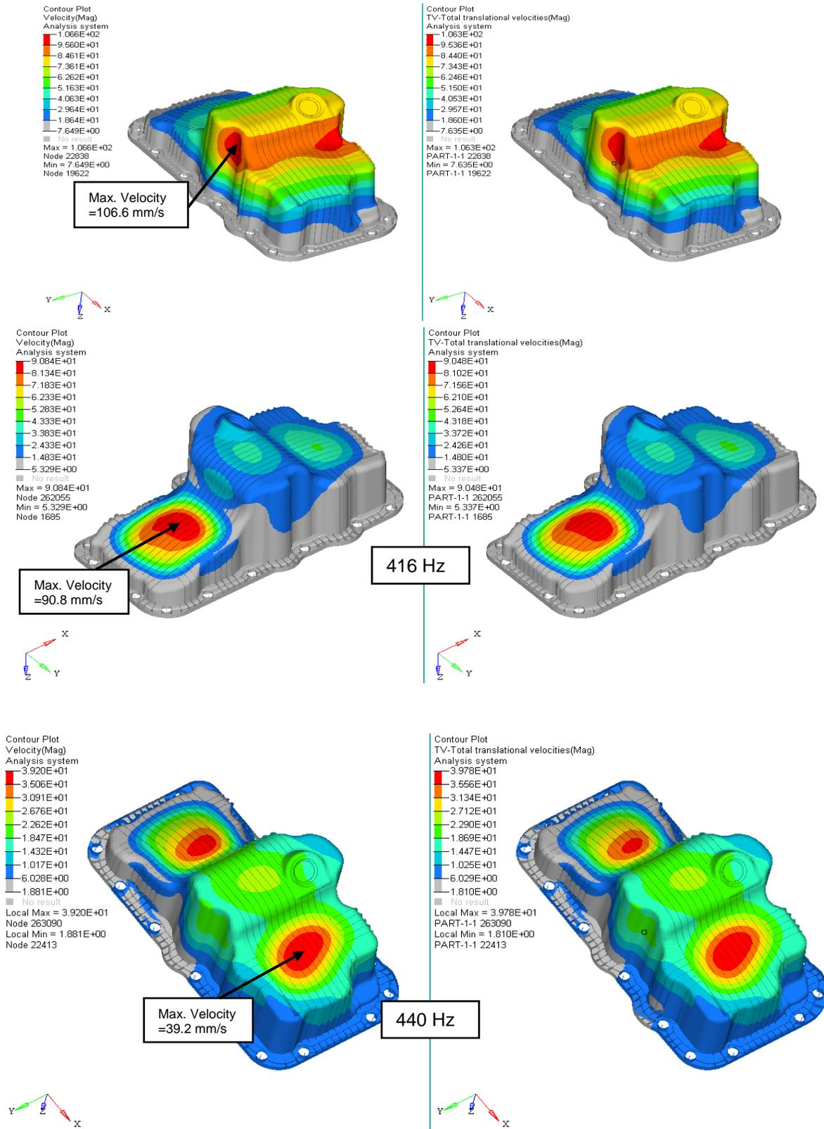
Figure 6 Comparison of velocity contour at different frequencies
