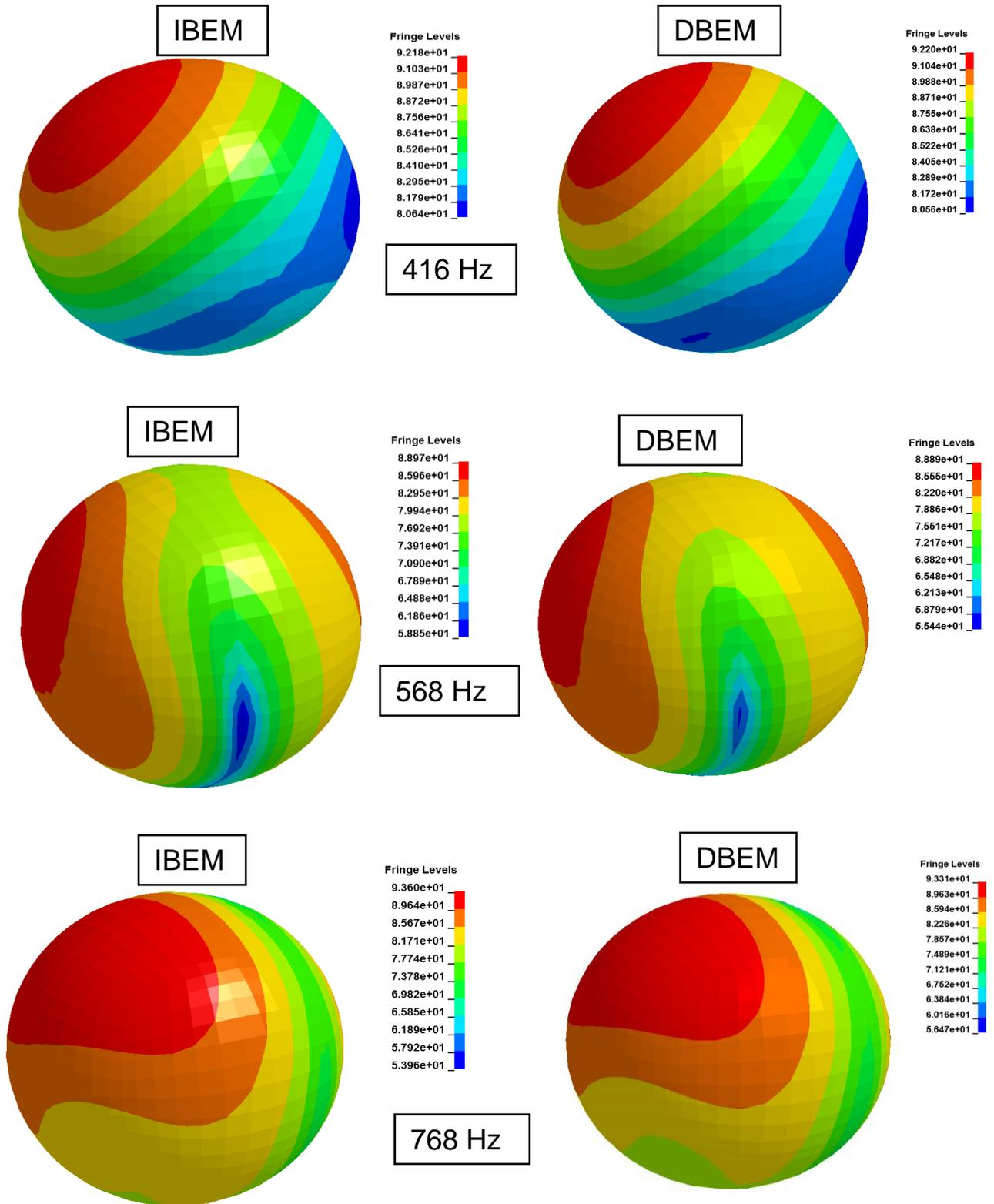
Figure 11 SPL contour on a spherical surface at different frequencies
