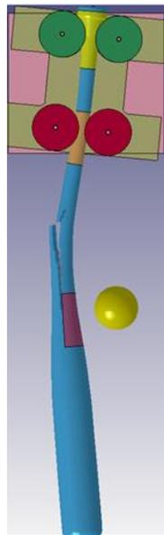
Figure 4: Single-piece failure of a baseball bat.
