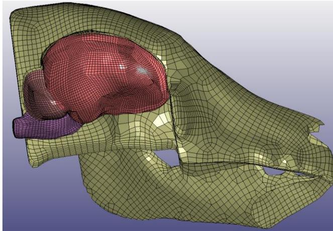
Figure 1. Pig head model with cerebrum, cerebellum, and brainstem visible.
