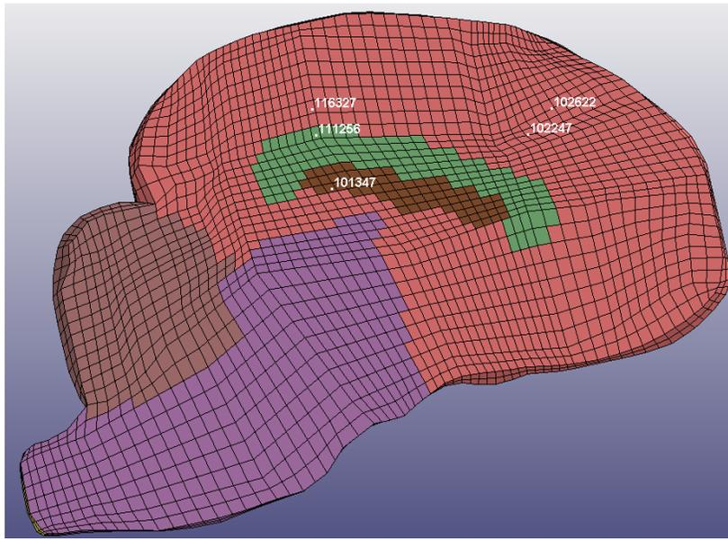
Figure 3. Half brain mesh showing locations of the nodes used for validation.
