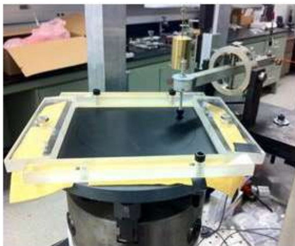
Figure 3 Experimental set-up for friction measurements.
