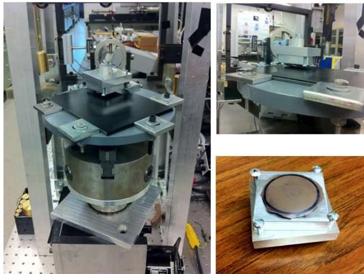
Figure 9 Experimental set-up for friction measurement between rubber and class C coated steel.
