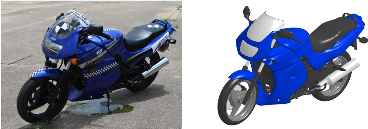
Figure 2. Comparison of Physical and FE model of 2005 Kawasaki Ninja 500R motorcycle.
