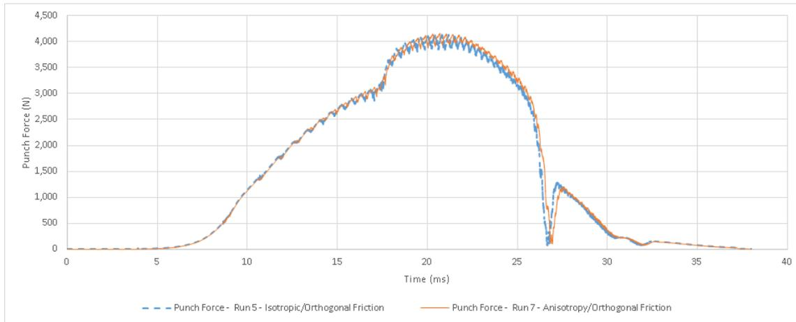
Figure 10: Punch Force Comparison for Runs 5 and 7
