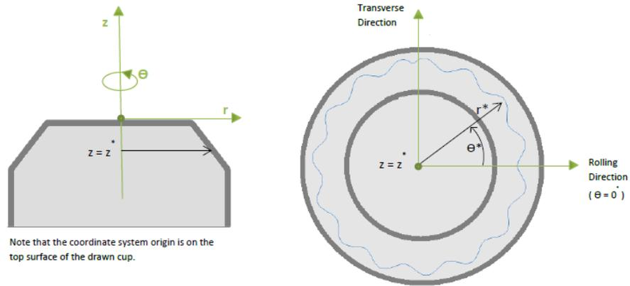
Figure 2: Model Coordinate System for Wrinkle Amplitude Examination
