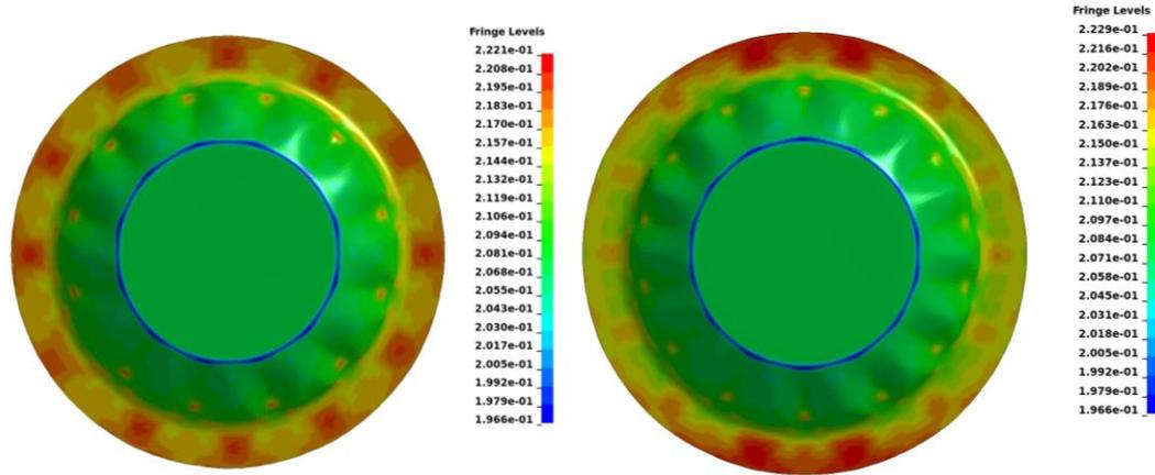
Figure 8: Flange shell thickness during draw with isotropic material model (left), flange shell thickness during draw with anisotropic material model (right)
