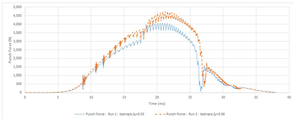
Figure 5: Punch Force Comparison for Runs 1 and 2
