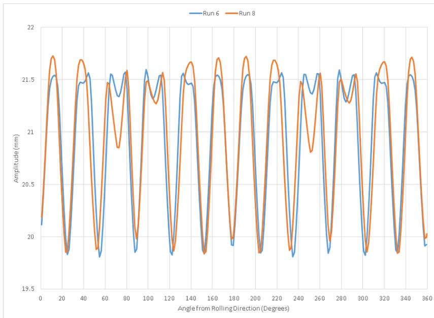
Figure 11: Wrinkle Amplitude for Runs 6 (Isotropic Material) and 8 (Anisotropic Material)
