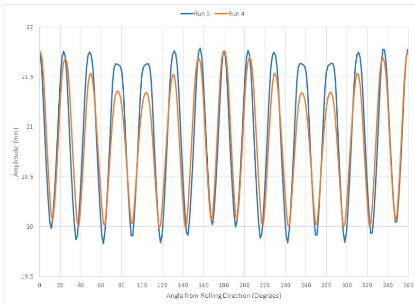
Figure 6: Wrinkle Amplitude for Runs 3 and 4
