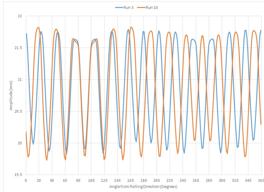
Figure 14: Wrinkle Amplitudes for Runs 3 and 10 (Blank shifted  $y = -0.2\text{mm}$ )
