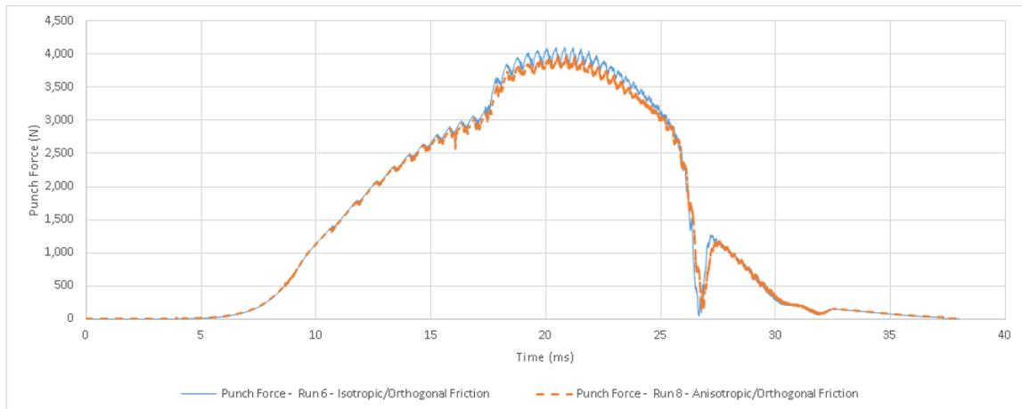
Figure 12: Punch Force Comparison for Runs 6 and 8
