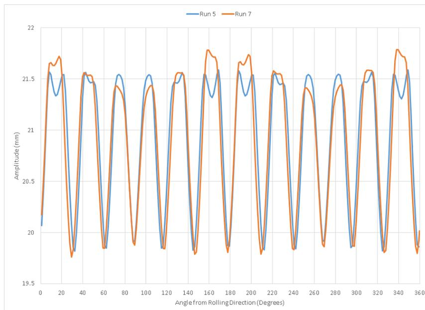
Figure 9: Wrinkle Amplitude for Runs 5 (Isotropic Material) and 7 (Anisotropic Material)
