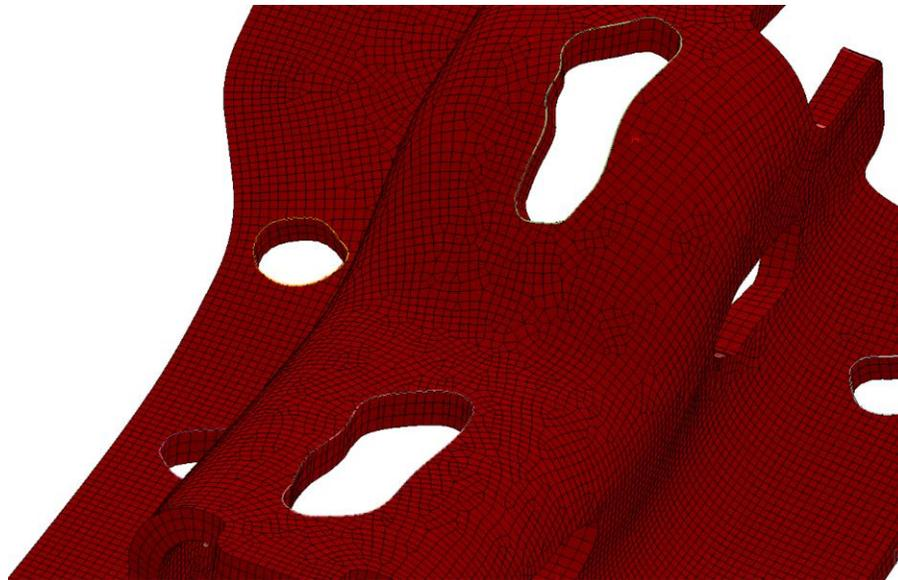
Figure 14. 2-D trimming of solid elements.
