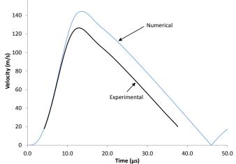
Figure 12: Predicted velocities with the modified Voce model and measured ring velocities.
