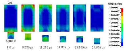
Figure 13: Current density distribution of the coil and sample. Contours are of µJ/mm<sup>3</sup>.
