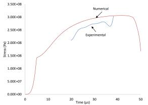
**Figure 12:** Predicted stresses with the modified Voce model and measured stresses. Experimental stresses are only shown for the area where eq. 4 is valid.
