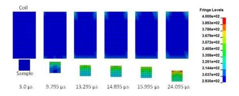
Figure 14: Temperature distribution of the coil and sample. Contours are of K°.
