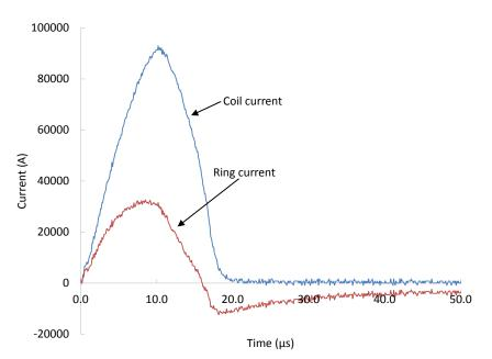
Figure 5: Experimental coil and ring currents from an interrupted pule EM expanding ring test.
