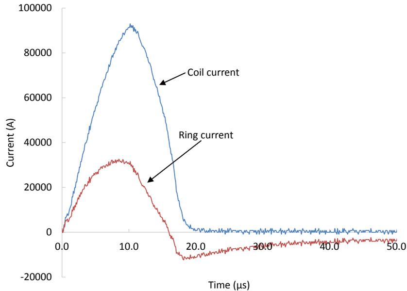
**Figure 5:** Experimental coil and ring currents from an interrupted pulse EM expanding ring test.
