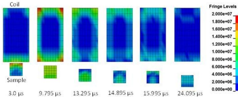
**Figure 13:** Current density distribution of the coil and sample. Contours are of  $\mu\text{J}/\text{mm}^3$ .
