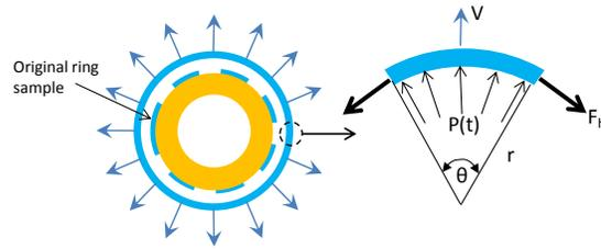
**Figure 1:** Basic principles of the expanding ring test.
