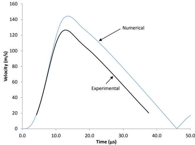
**Figure 12:** Predicted velocities with the modified Voce model and measured ring velocities.
