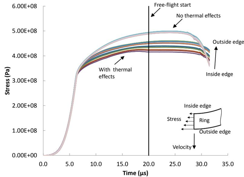
**Figure 15:** Predicted V-M stresses vs. time along the ring cross section from simulations with and without thermal effects. The inset shows an illustration of the stress state (Imbert and Worswick, 2016).
