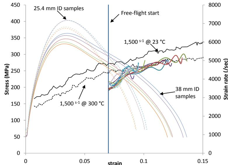
**Figure 7:** Strain rate and stress versus true strain for the five 38 mm ID and five 25.4 ID sample. Data for  $1,500 \text{ s}^{-1}$  from Smerd *et al.* (2005). (Imbert and Worswick, 2016).
