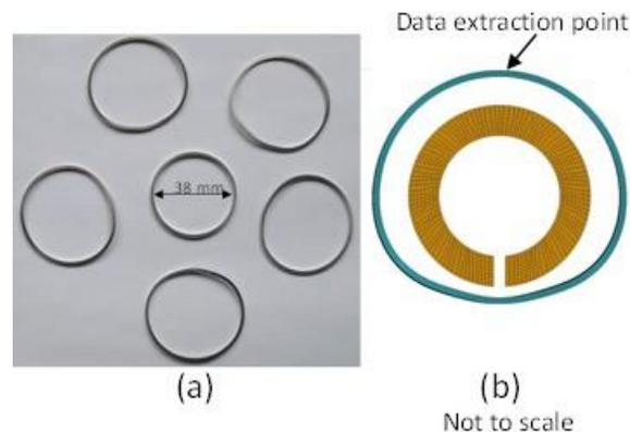
**Figure 9:** Rings expanded experimentally surrounding an un-deformed ring (a) and the final predicted shape of an expanded ring (b).
