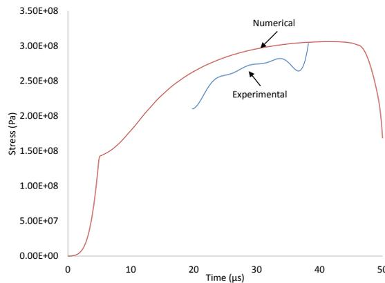
**Figure 12:** Predicted stresses with the modified Voce model and measured stresses. Experimental stresses are only shown for the area where eq. 4 is valid.
