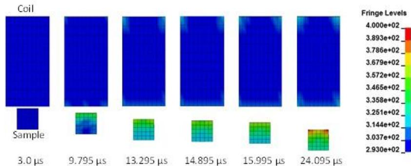
**Figure 14:** Temperature distribution of the coil and sample. Contours are of  $\text{K}^\circ$ .
