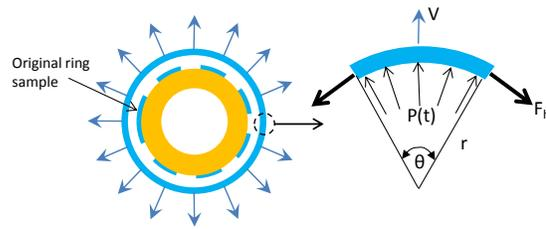
**Figure 1:** Basic principles of the expanding ring test.
