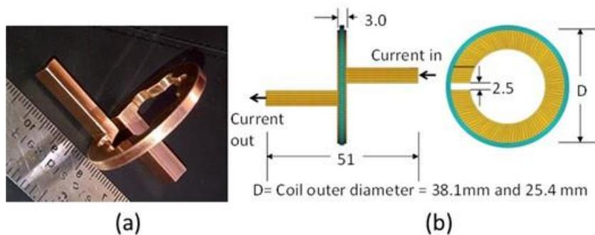
**Figure 6:** Single turn copper coil used (Imbert and Worswick, 2016).
