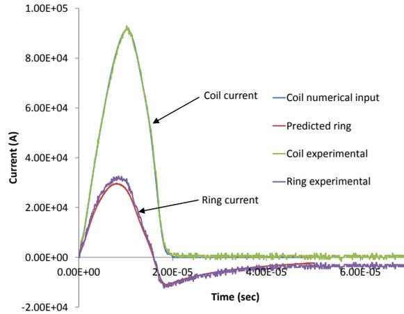
**Figure 10:** Measured and predicted coil and ring currents (Imbert and Worswick, 2016).
