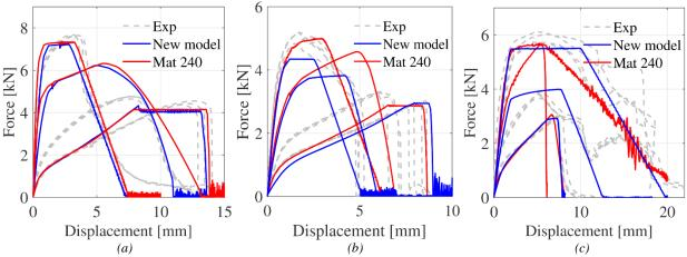
Figure 10: Results from calibration of the new model compared to \*MAT\_240 for (a) the SPR connection, (b) the small FDS connection and (c) the large FDS connection.
