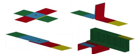
Figure 9: FE models used: cross (top left), single lap joint (bottom left), peeling (top right) and T-component (bottom right).
