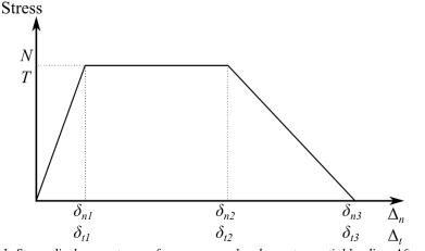
Figure 1: Stress-displacement curve for pure normal and pure tangential loading. After [3].
