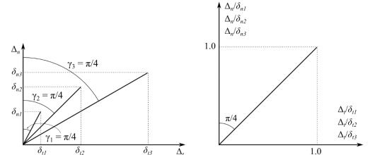
Figure 2: Illustration of normalized mode mixity angles in displacement plane (left) and normalized displacement plane (right).
