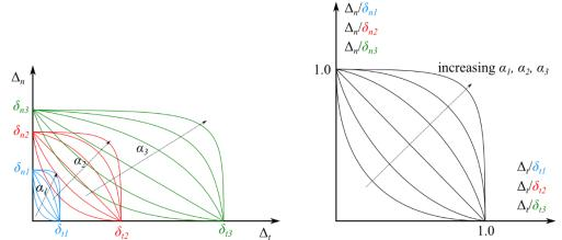
Figure 3: Interaction curves for yield-, damage initiation- and failure displacements in displacement plane (left) and normalized displacement plane (right).
