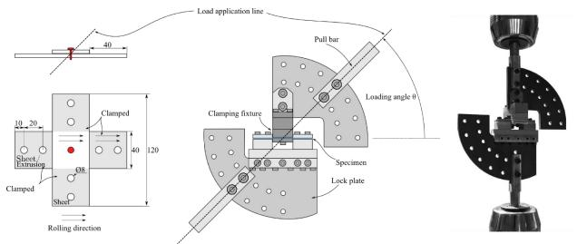
Figure 5: Cross specimens (left) and cross test rig (middle and right). After [1].
