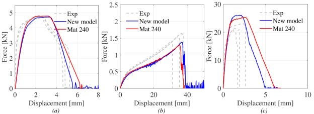
Figure 12: Validation simulations for the small FDS connection, (a) single lap-joint, (b) peeling and (c) T-component test.
