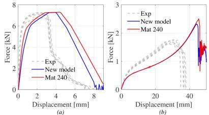
Figure 11: Validation simulations for the SPR connection, (a) single lap-joint and (b) peeling test.
