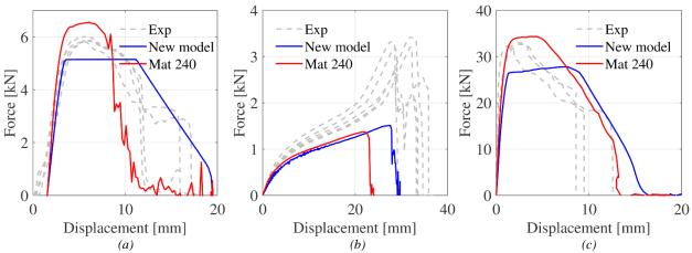
Figure 13: Validation simulations for the large FDS connection, (a) single lap-joint, (b) peeling and (c) T-component test.
