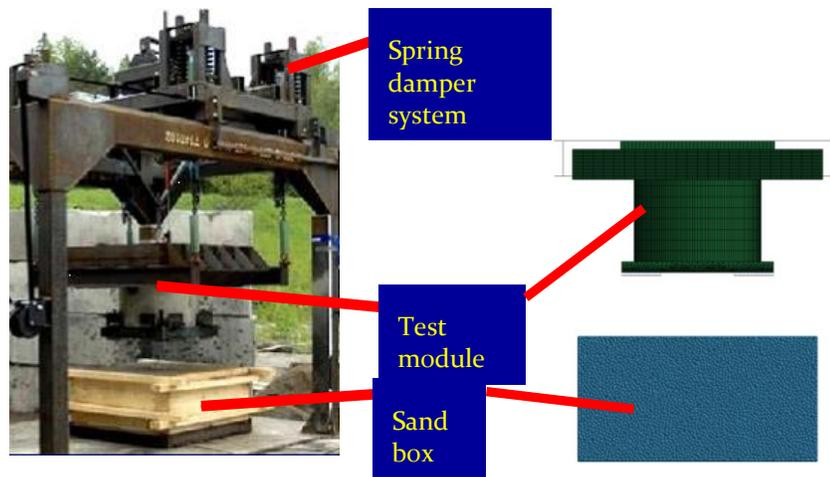
Figure 10 Experimental set up and numerical model of explosions in soil
