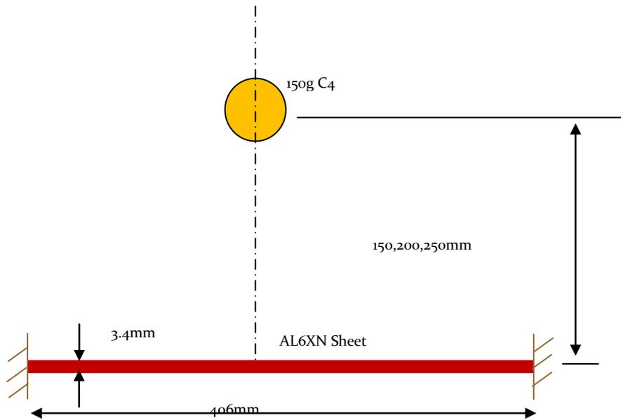
Figure 3 Sketch of the experimental set-up
