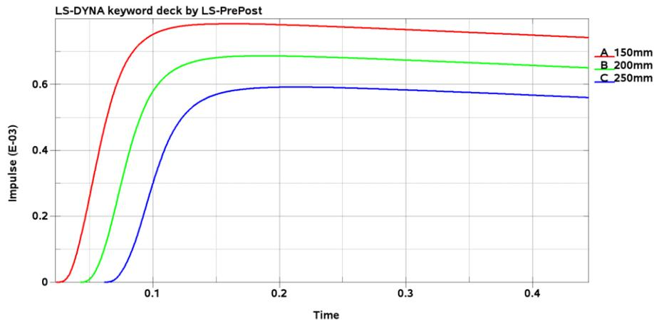
Figure 6 Reflected impulse for 150mm, 200mm and 250mm stand-off distance
