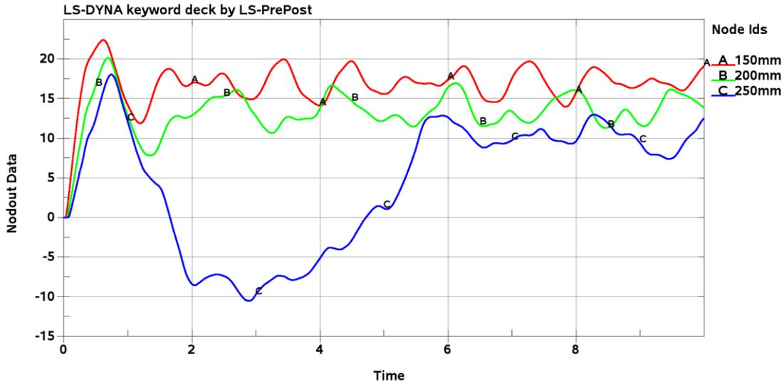
Figure 5 Central node displacement versus time for 150mm, 200mm and 250mm stand-off distance.
