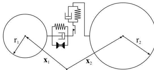
Figure 8 *Penalty-based particle-particle interaction in LS-DYNA.*
