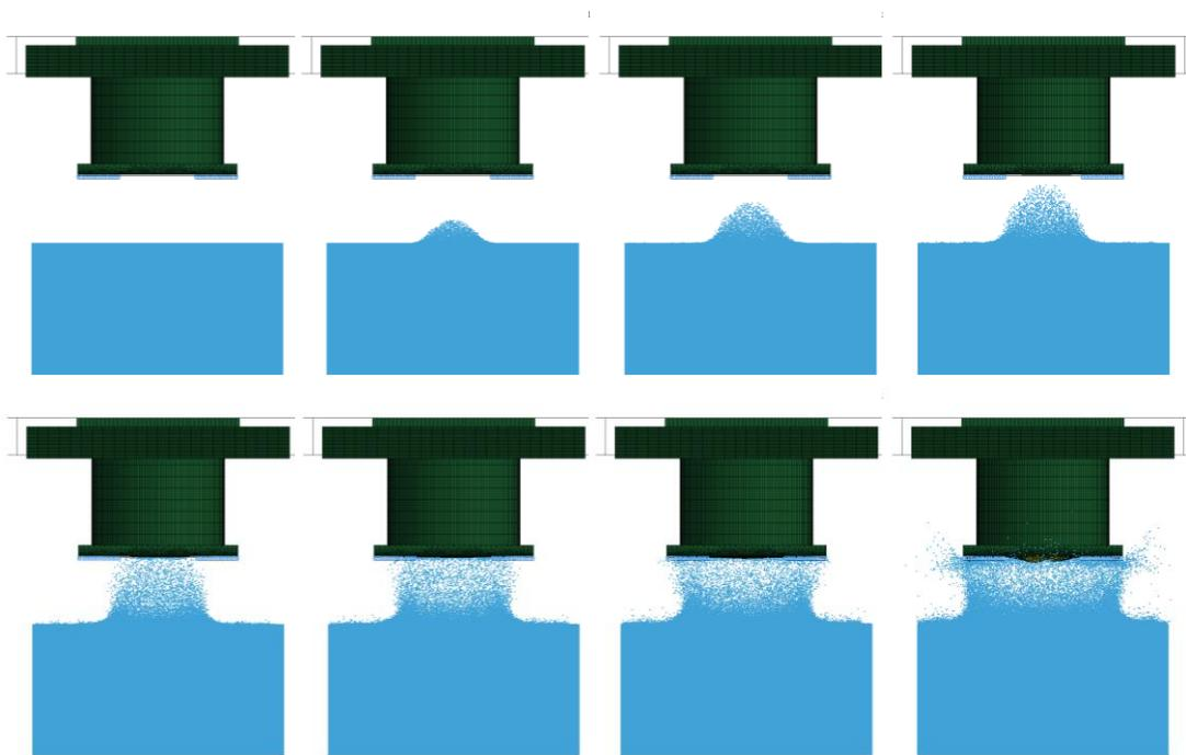
Figure 11 Explosion behavior for 50mm DOB
