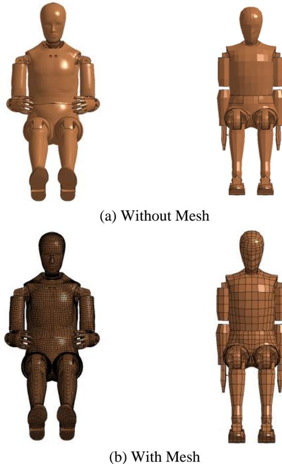
**Figure 6. Comparison of detailed dummy model (left) and fast dummy model (right).**
