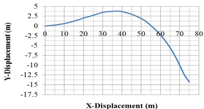
**Figure 5. Rollover path as input into TruckSim tractor-trailer rollover event.**
