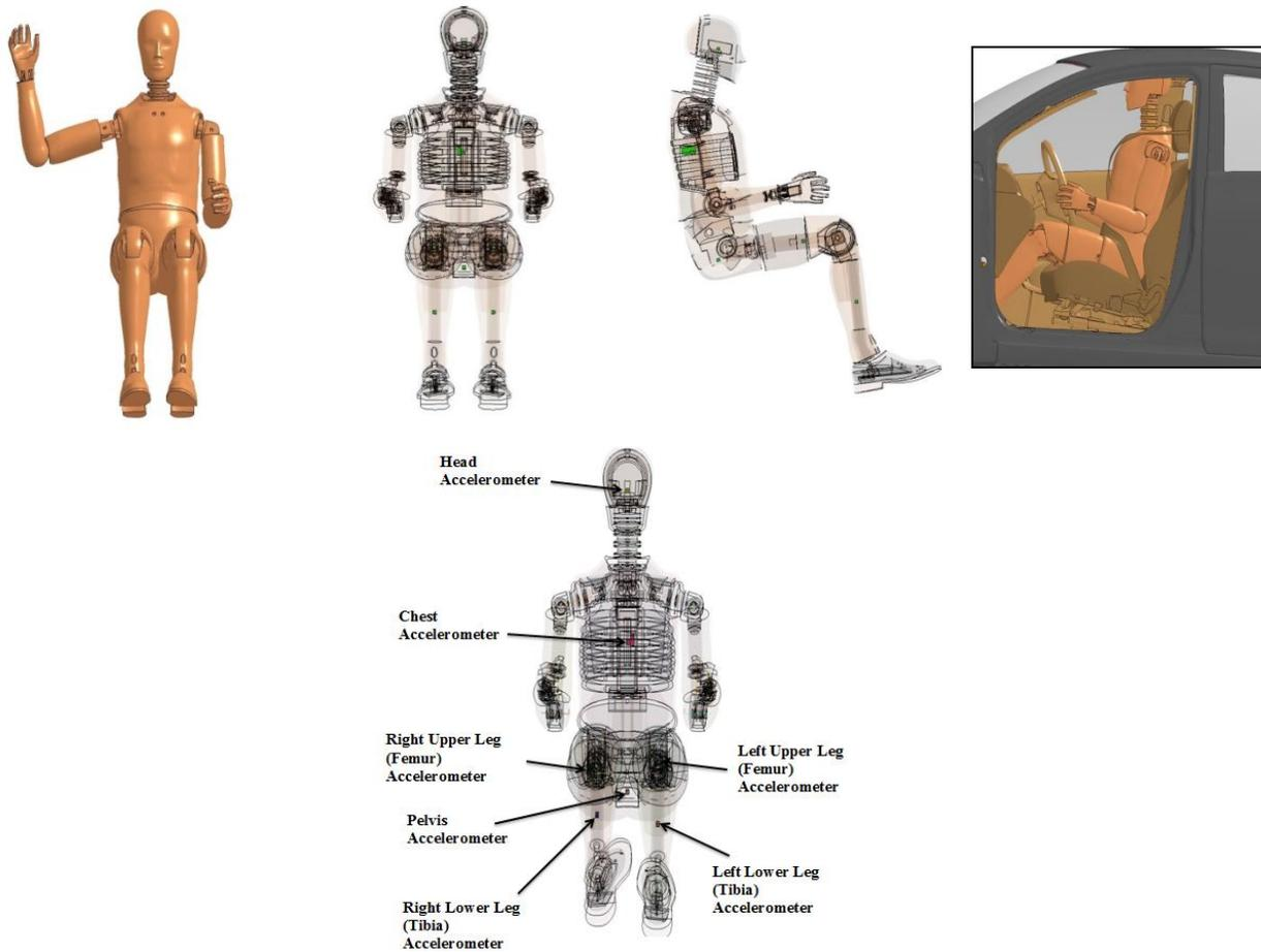
Figure 3. FE model of the Hybrid III 50<sup>th</sup> percentile male dummy.
