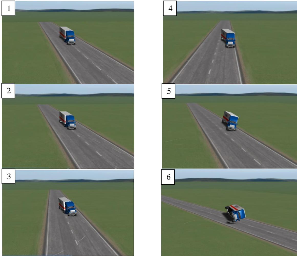
Outputs of interest from the TruckSim rollover simulation were displacements at four cab mount locations. Measurements were taken in a FE model of a tractor-trailer for the exact locations of the cab mounts to determine where to output displacements from TruckSim. At these four locations x, y and z displacements were output over time. These displacement curves were then applied in our truck cabin model by BOUNDARY\_PRESCRIBED\_MOTION cards at the four locations.
